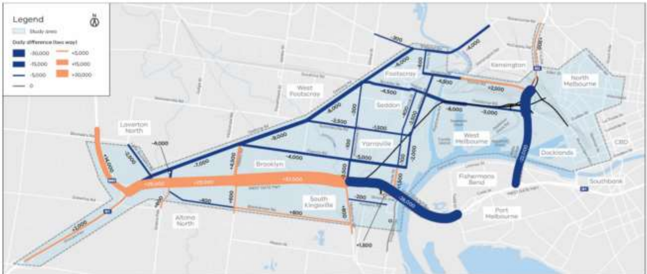
Figure 5-3 Difference in daily two-way traffic volumes (for all vehicles) - 2031 project case vs 2031 no project case Source: West Gate Tunnel Project, EES, Chapter 11 – Effects on traffic and transport
