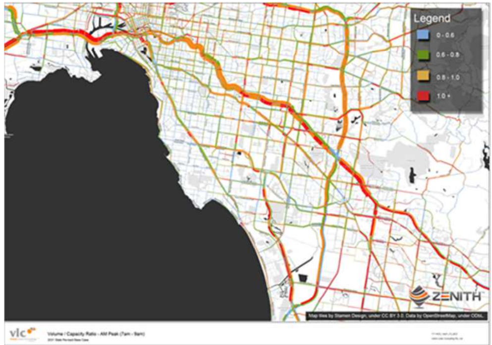
Figure 14: Base case volume capacity ratios – AM peak (7am – 9am), 2030/31
