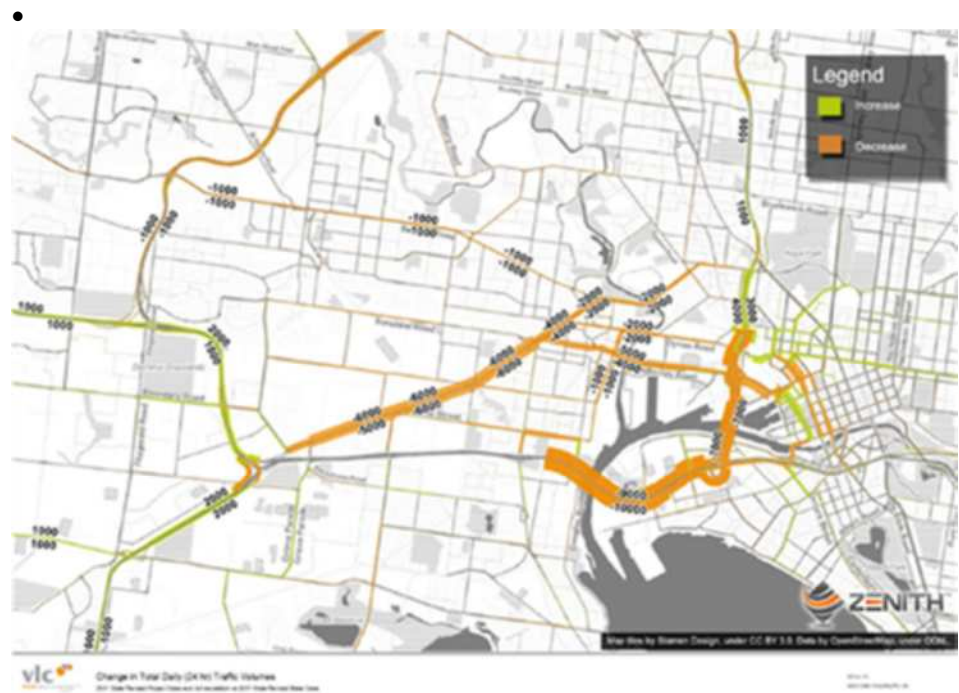
Figure 5: Change in total daily traffic volumes (2030/31 project case vs 2030/31 base case, 24 hour average weekday)
