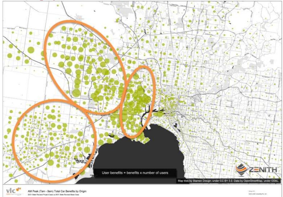
Figure 8: Travel Time Benefits by Origin – Car, AM Peak (7am - 9am), (2030/31 project case vs 2030/31 base case)
