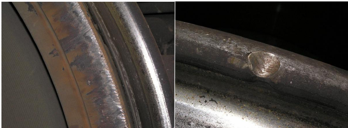
Figure 3 - Wheel 7 scuff marks and indentation
