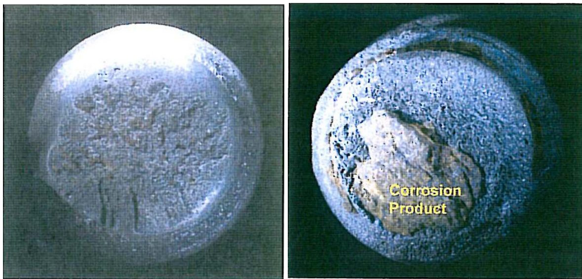
Figure 11 - Fracture surface of 'R' and 'S' screws
