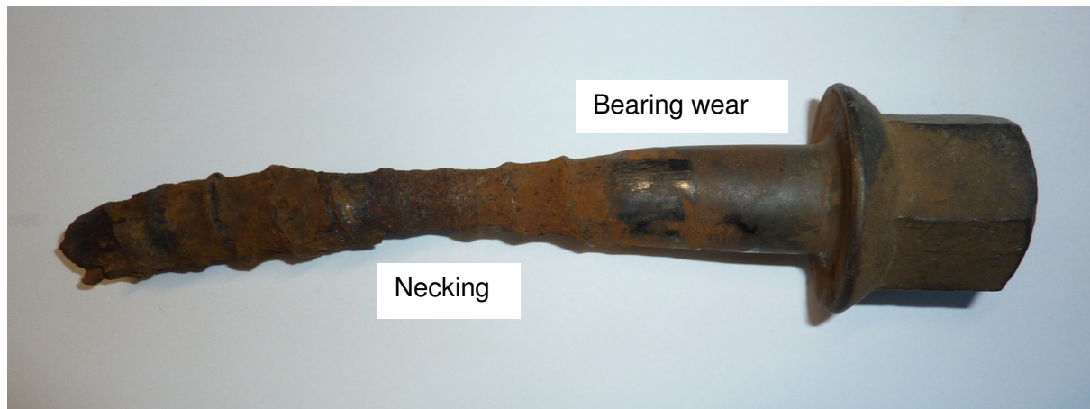
Figure 9 - Corroded 'S' Screw showing bearing wear on shank
