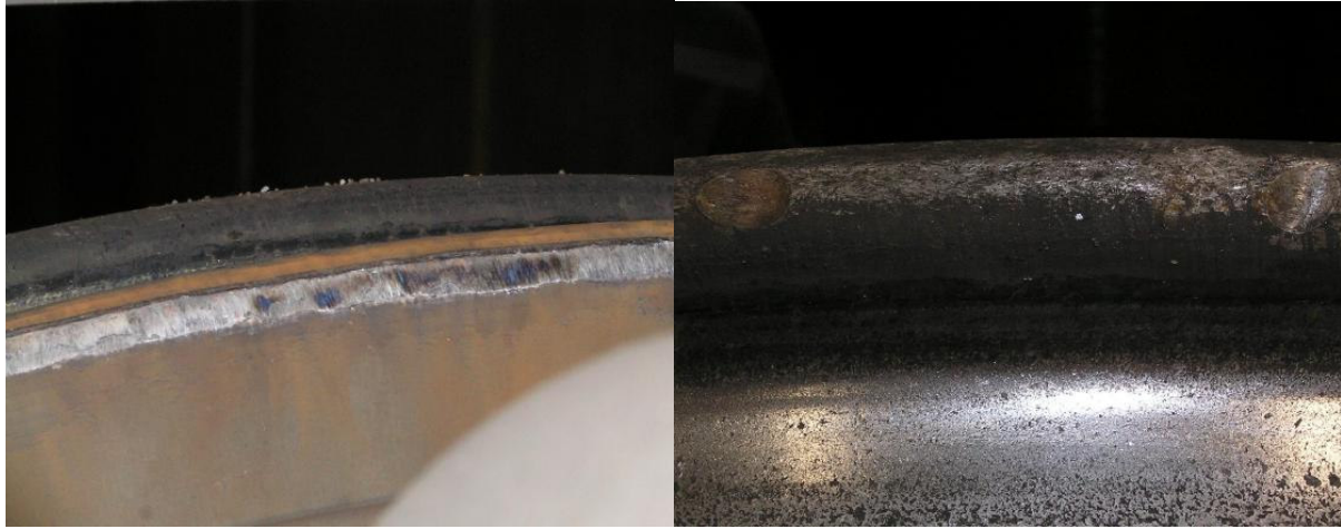
Figure 4 - Wheel 8 scuff marks and indentation
