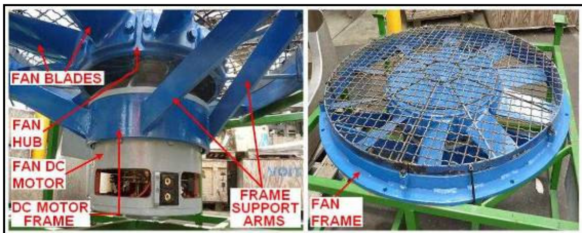
Figure 2 - Dynamic brake grid blower assembly showing component parts
