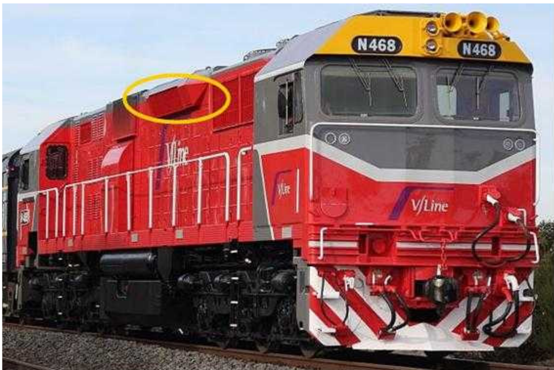
Figure 1 - An N-class locomotive, with the air intake to the dynamic brake grids circled
