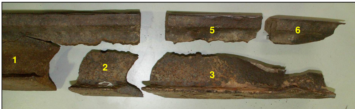
Figure 10 - Side elevation showing corroded web fracture
