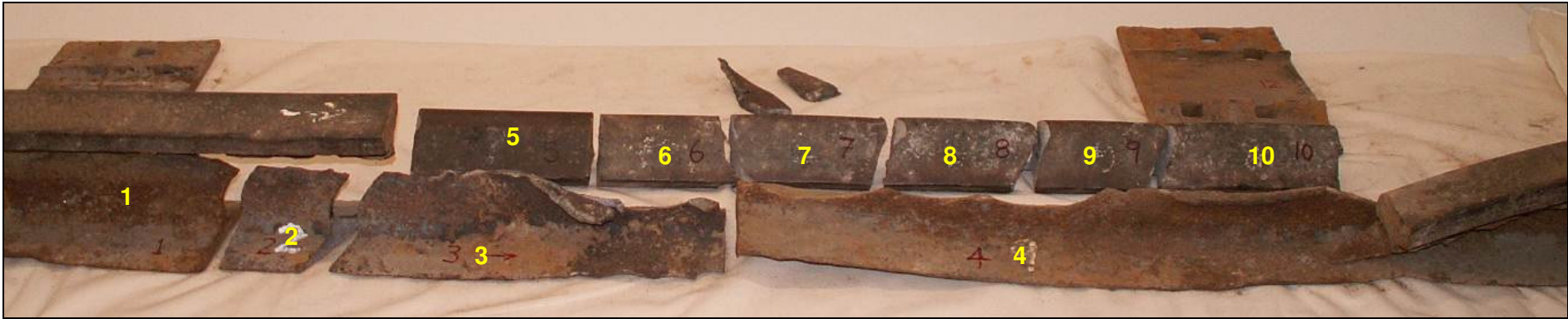
Figure 9 - Side elevation of the broken rail subject to metallurgical inspection
