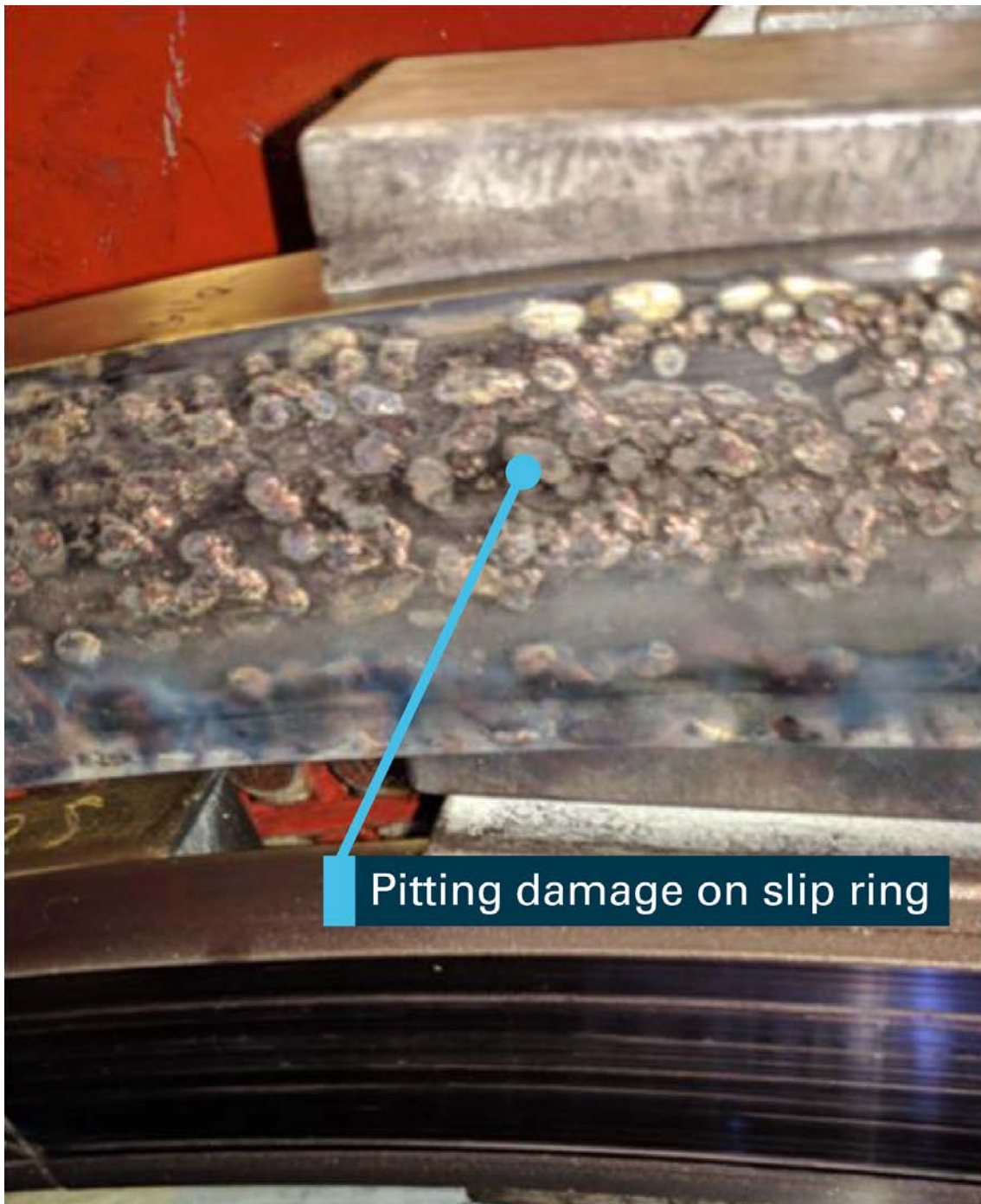
Figure 6: Arcing damage on the outer slipring
