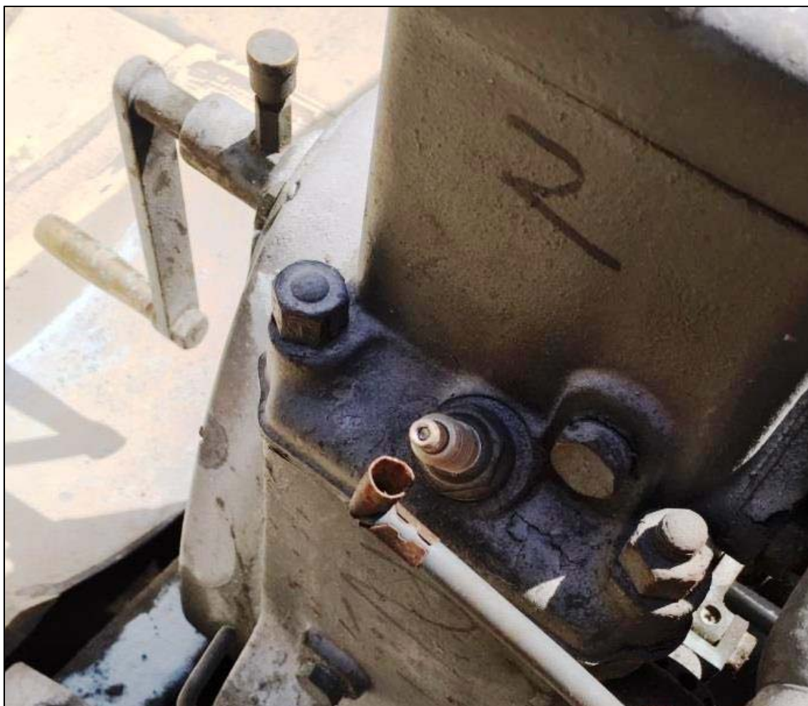
Figure 6: Connecting arrangement between high-tension lead and spark plug. The terminal connection could easily be lifted from the spark plug as shown
