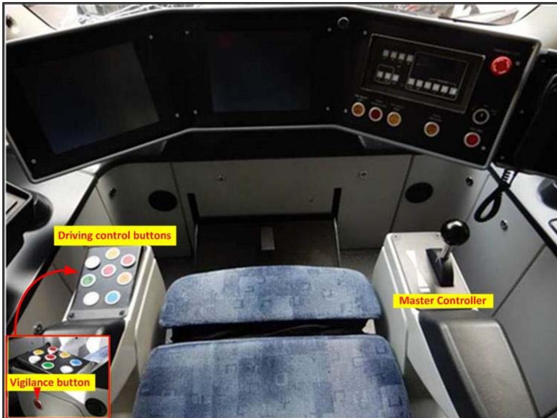
Figure 3: E Class tram driving controls. Inset: vigilance button on the side of the armrest.
