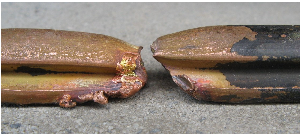
Figure 13 ‘Necking’ shape of contact wire evidences the tensile failure and consequent pull-apart.
