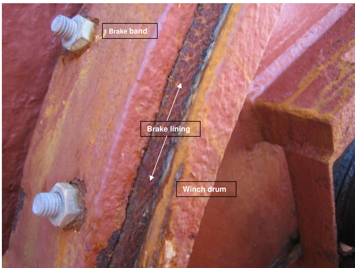
Figure 8 – Close-up of winch brake assembly post incident
