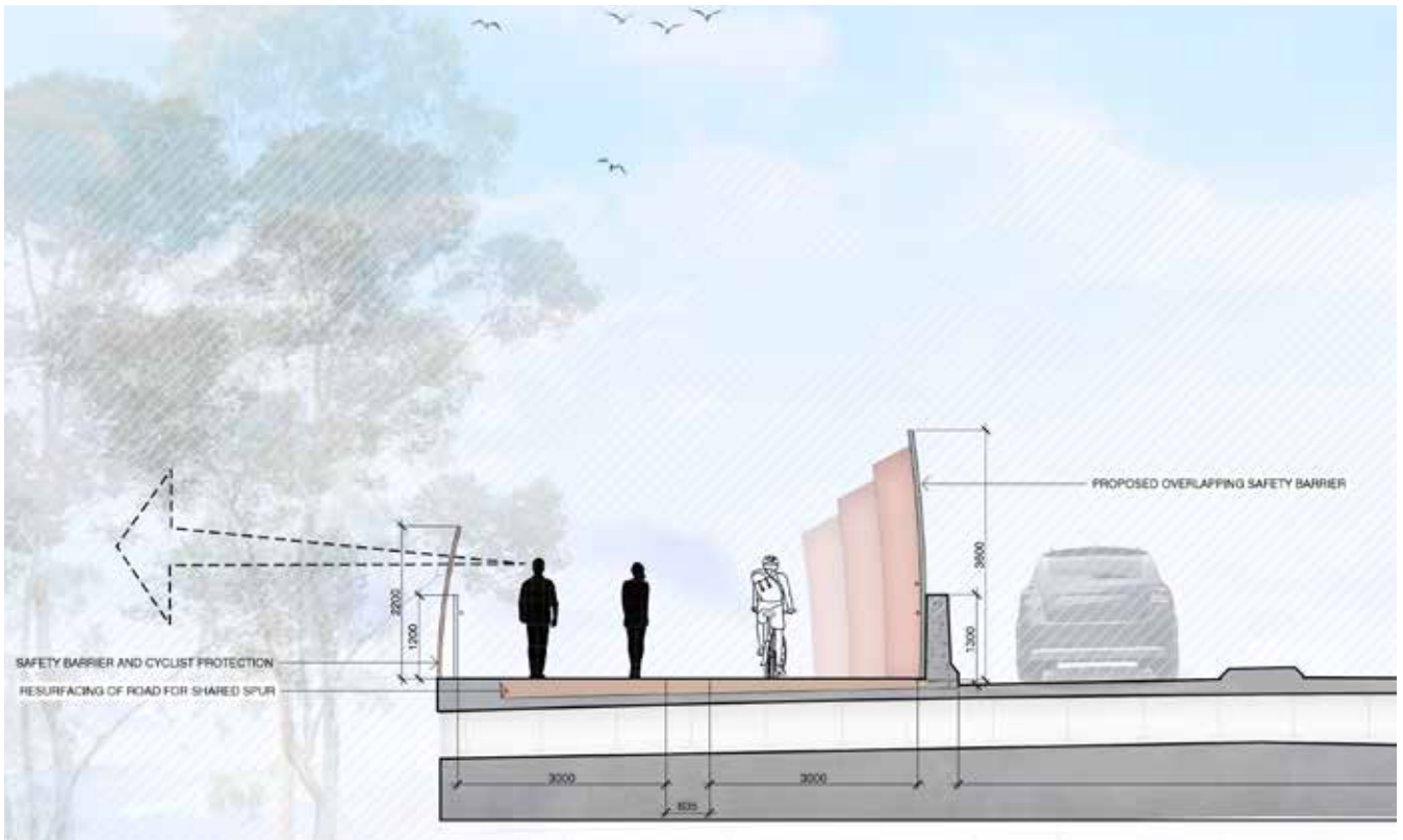
Illustrative, indicative typical section of the spurline, showing the separation between people walking and cycling and vehicles, a safety barrier on the northern edge and the resurfacing of the road.
