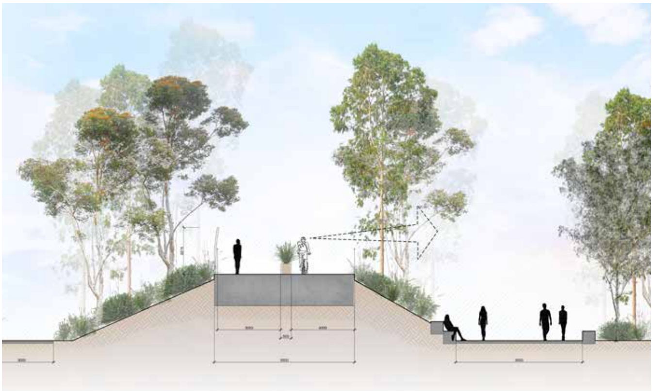
Illustrative, indicative section of the spurline on the eastern side, showing how the space on the spurline could be split for both walking and cycling, with the new direct pedestrian route connecting with Hampshire Road main street and the new open space on the right.
