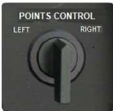
Figure 7: Points selector switch
