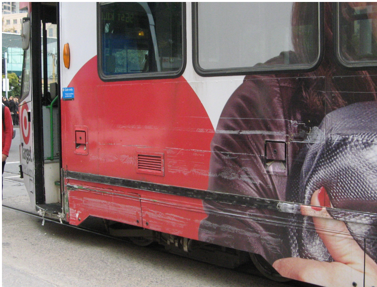
Figure 5. View of side panel damage to Tram 2103.
