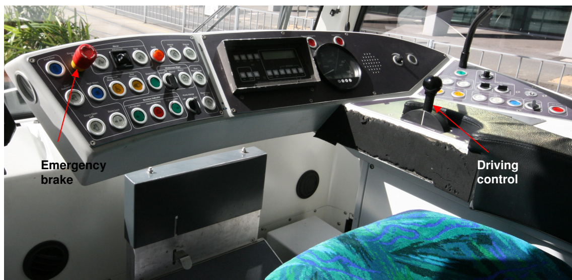
Figure 3 Tram 3510 Driving console
