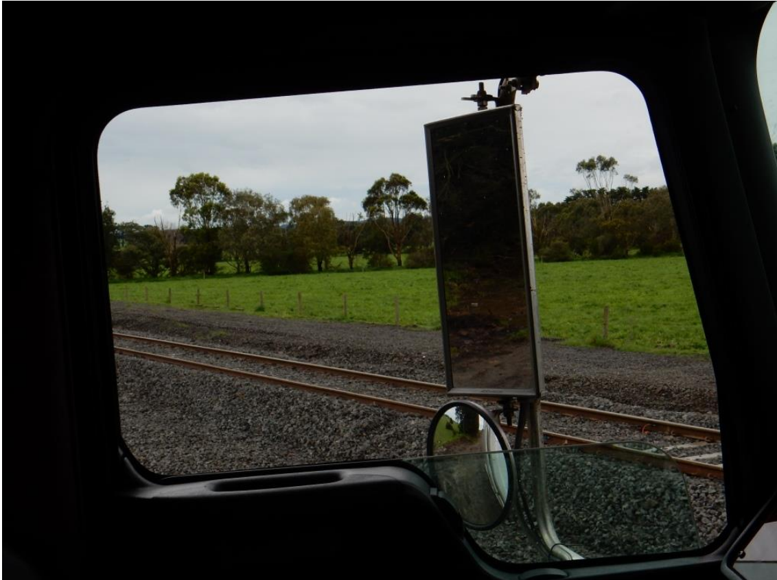
Figure 14: The restricted view along the track with the truck stopped 10 m from the track
