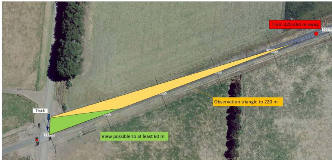
Figure 17: The position of the train when the truck started moving towards the crossing.
