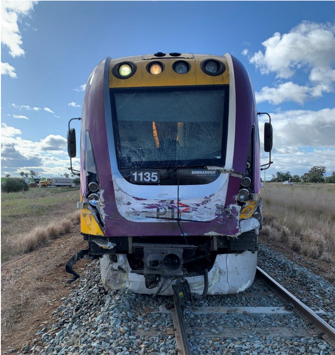
Figure 7: Damage to the front of the train
