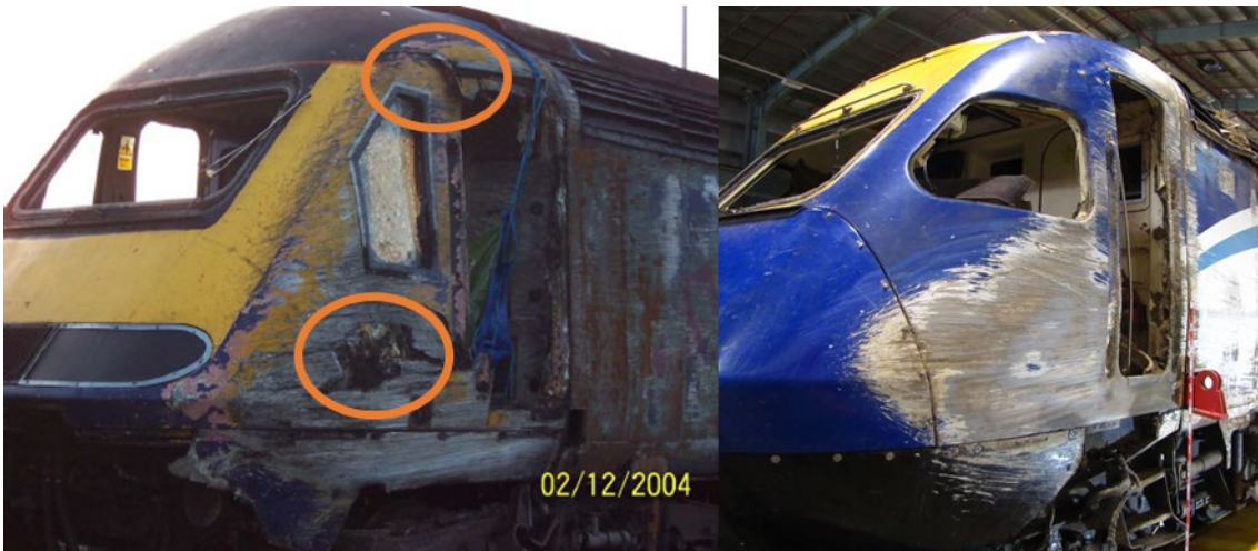
Figure 21: Ufton Nervet cab side damage (left) and Wallan cab side damage (right)
