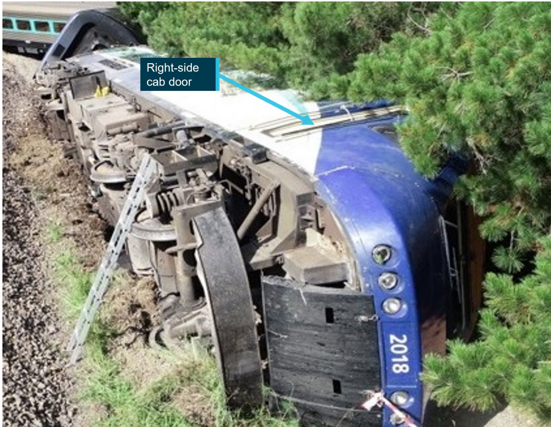
Figure 15: Power car XP2018 overturned and access route via right door
