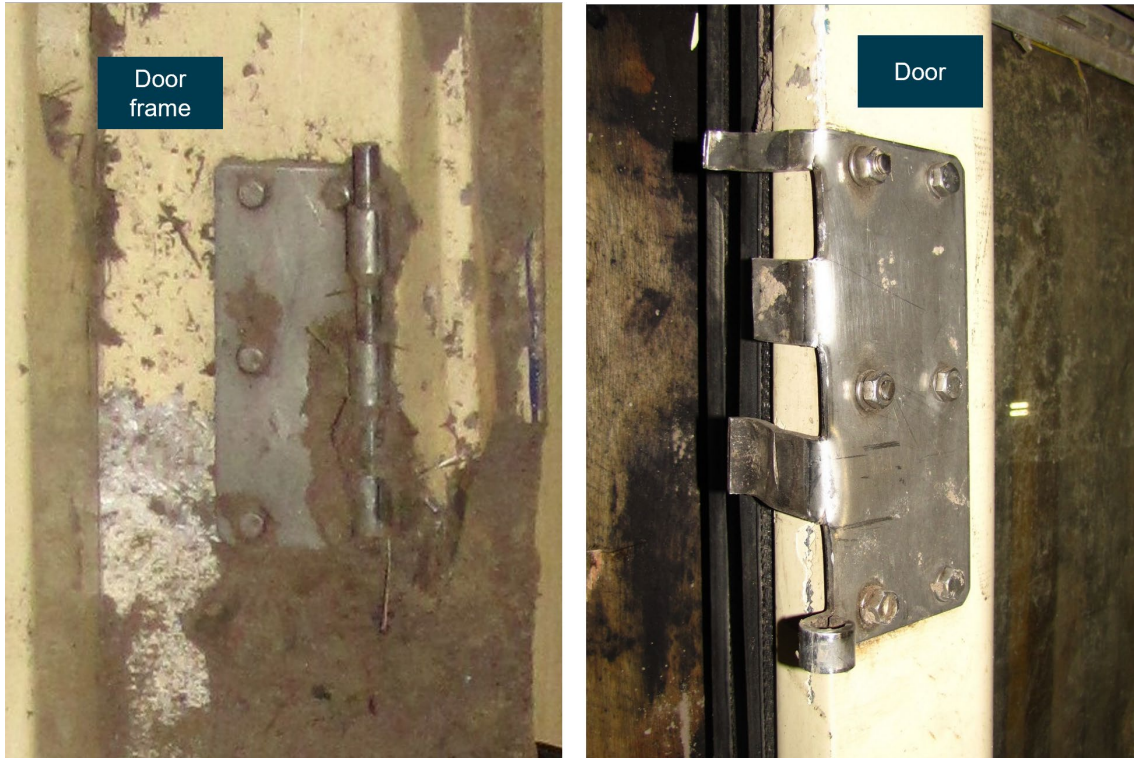
Figure 18: Upper internal hinge of left cab door of XP2018
