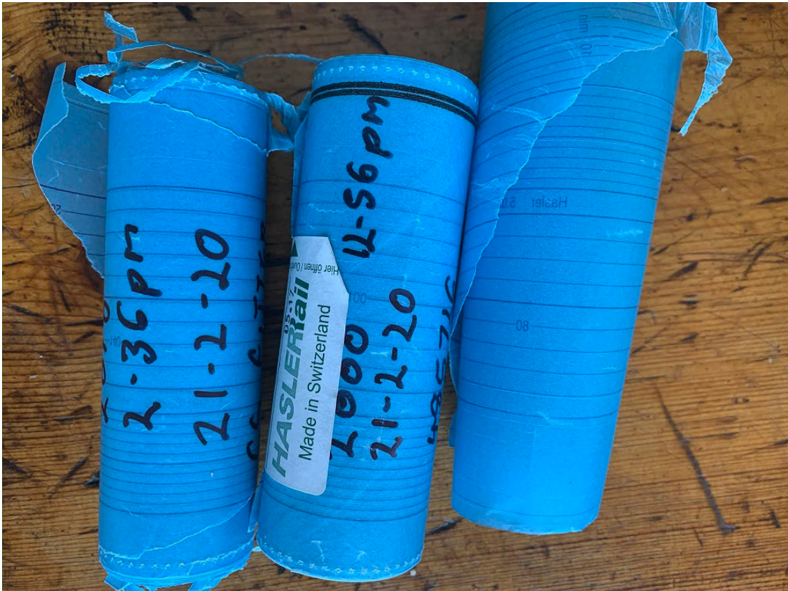
Figure 23: Hasler waxed paper rolls removed from power cars XP2018 and XP2000
