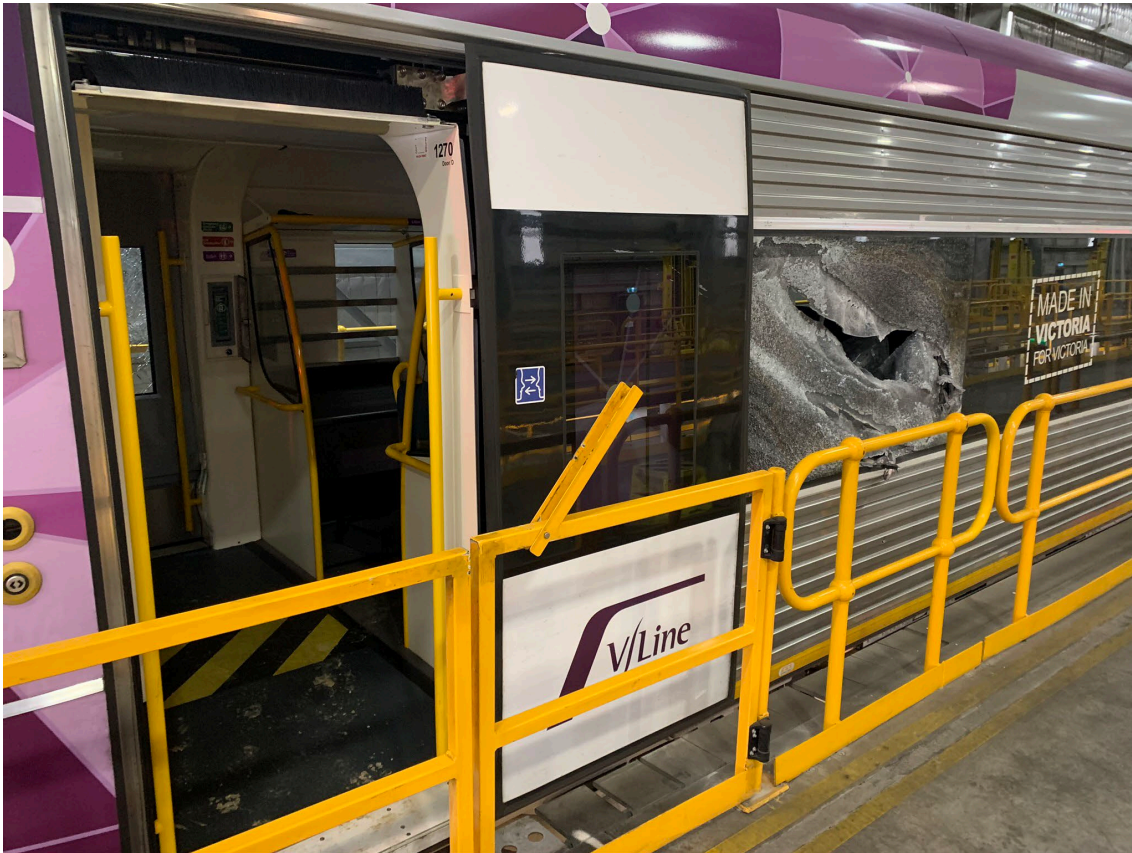
Figure 4: VLocity car 1270 impact damage to passenger (left) side leading window
