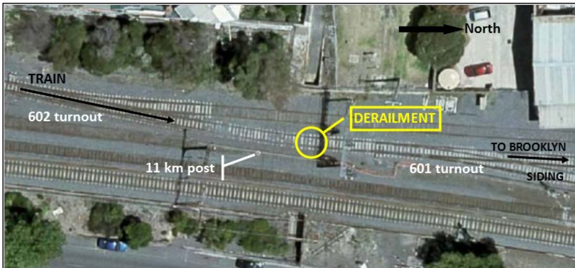
Figure 2: Track layout, shown after restoration works
