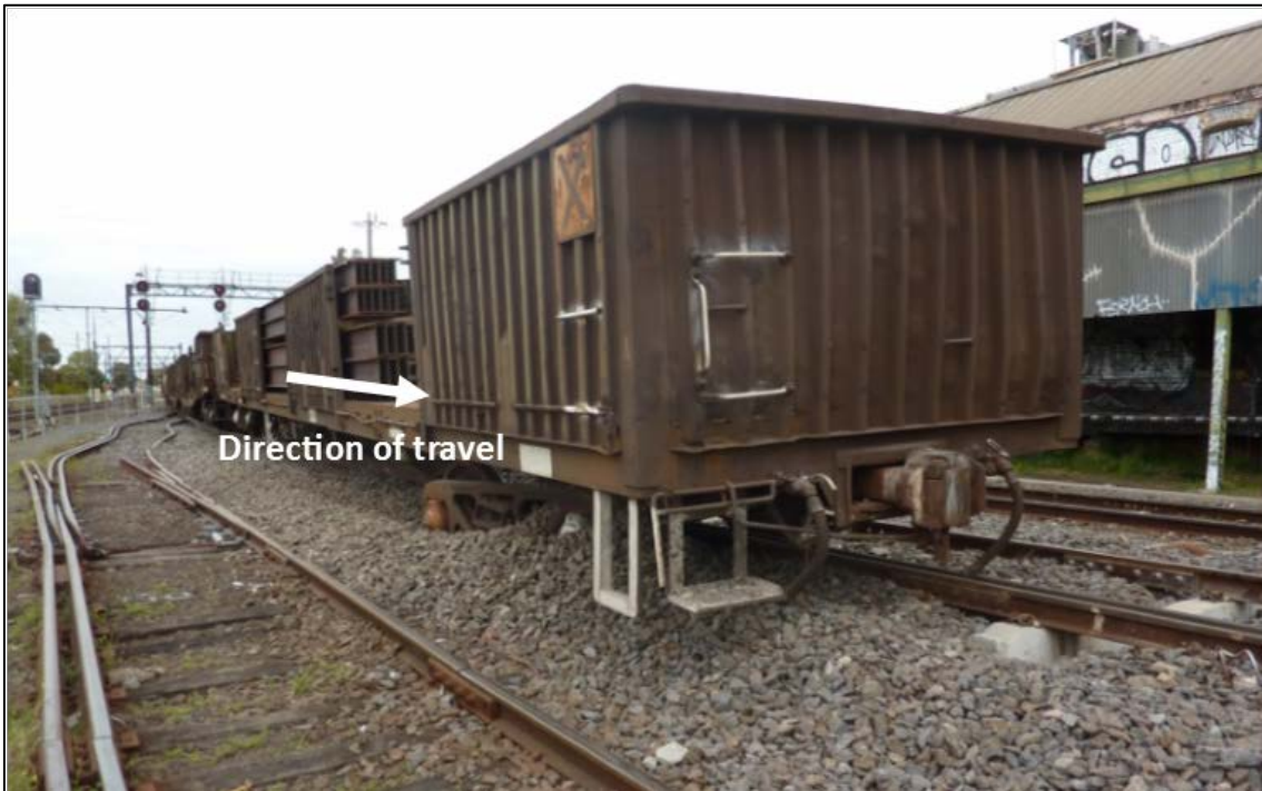
Figure 1: Derailed wagon RKOX 4072D and track damage to adjacent siding
