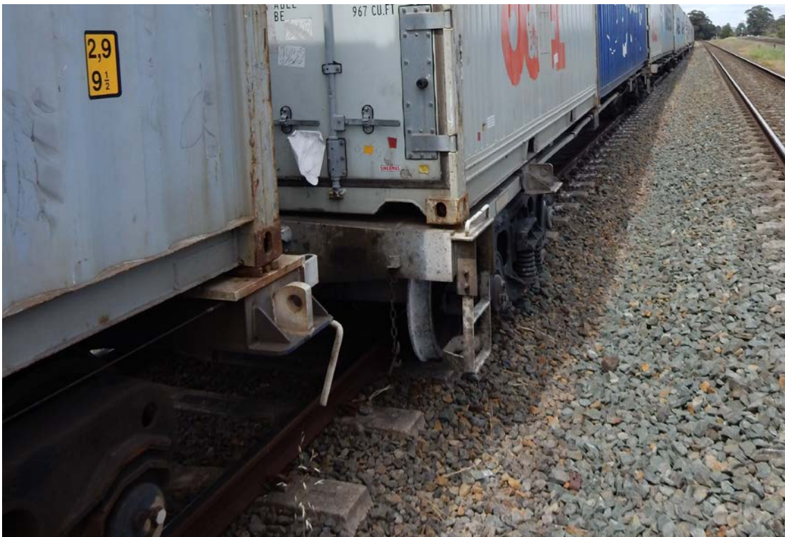
This picture shows the derailed wagon after the train was stopped when departing Wallan Loop. Source: Chief Investigator, Transport Safety (Vic)
