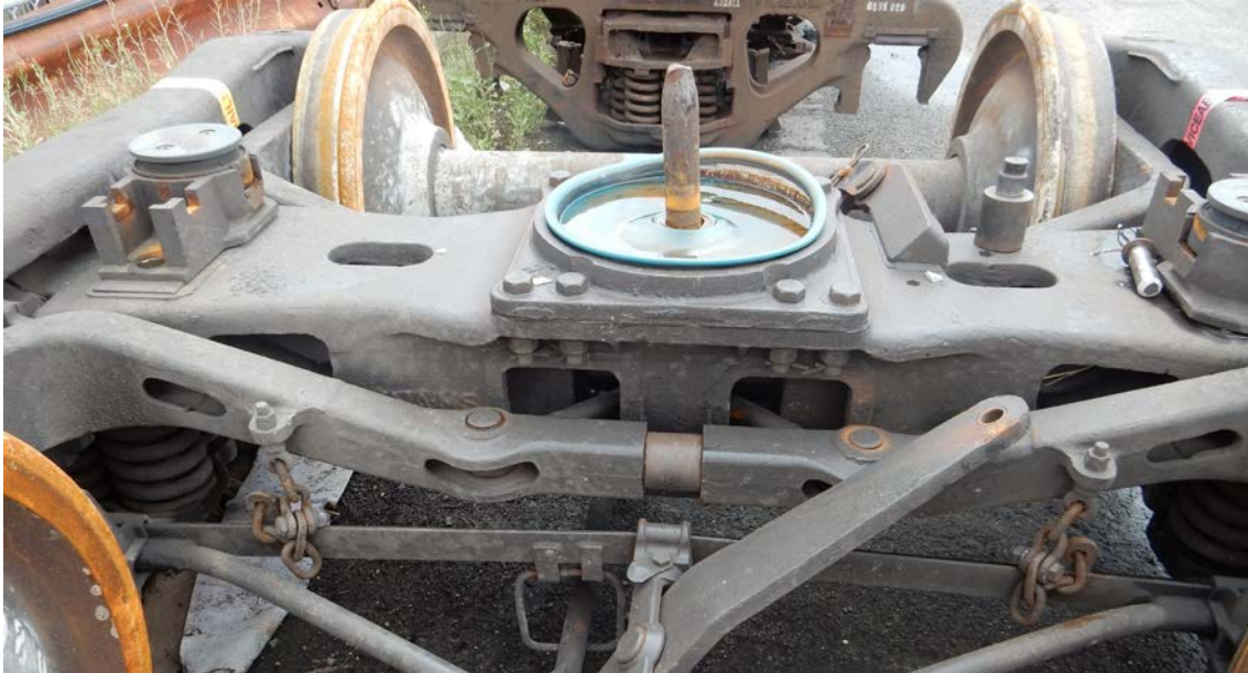
Figure 15: The derailed bogie at the post-incident inspection
