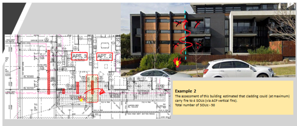
Figure 5.5: Example plan/elevation markup and screen capture from Max SOU assessment (from presentation slides prepared by CSV in February 2021)
