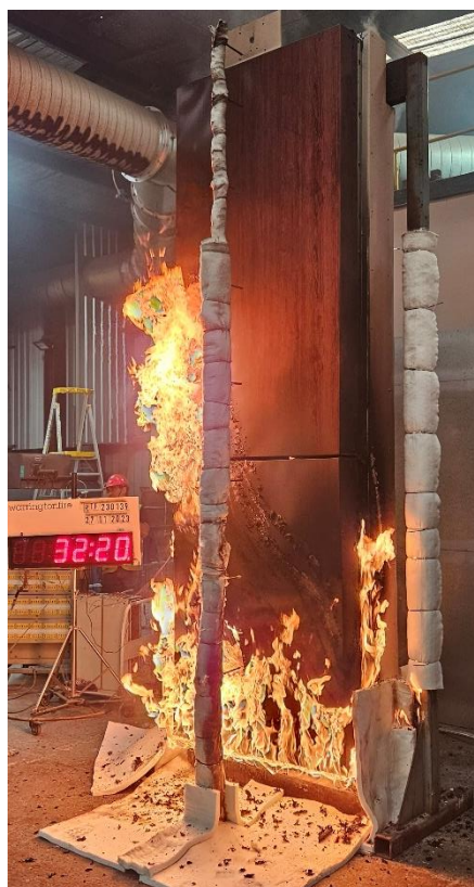
Figure 19 The specimen 32 minutes 20 seconds into the test (17 minutes 20 seconds after burner output was changed to 300 kW)
