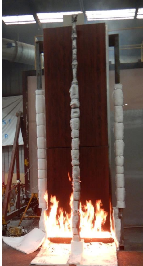
Figure 14 The specimen 8 minutes 49 seconds into the test (burner output at 100 kW)
