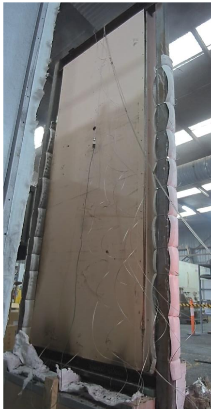
Figure 27 The specimen after the test – unexposed side.
