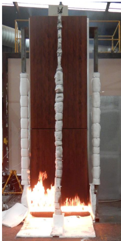
Figure 13 The specimen 3 minutes 58 seconds into the test (burner output at 100 kW)
