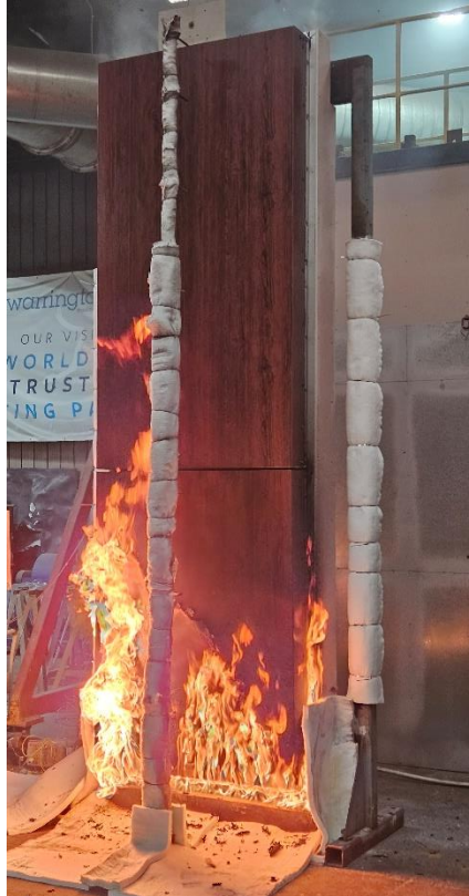
Figure 16 The specimen 16 minutes 12 seconds into the test (1 minute 12 seconds after burner output was changed to 300 kW)
