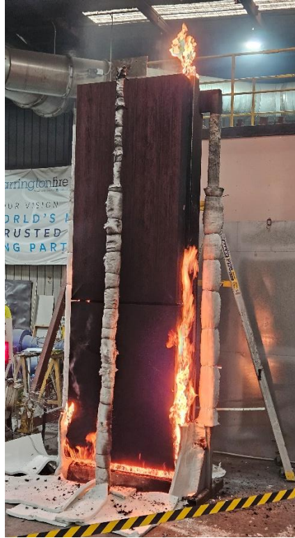
Figure 22 The specimen 40 minutes 30 seconds into the test (30 seconds after burner was switched off)
