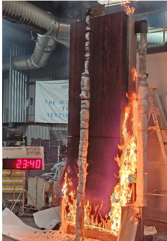
Figure 18 The specimen 23 minutes 40 seconds into the test (8 minutes 40 seconds after burner output was changed to 300 kW)
