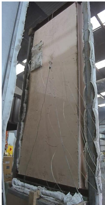
Figure 25 The specimen after the test – unexposed side
