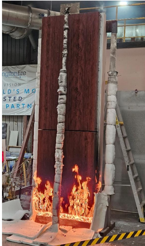
Figure 14 The specimen 8 minutes 35 seconds into the test (burner output at 100 kW)
