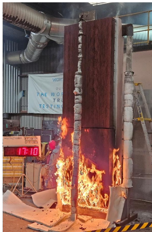
Figure 17 The specimen 17 minutes 10 seconds into the test (2 minutes 10 seconds after burner output was changed to 300 kW)
