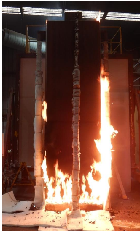
Figure 19 The specimen 29 minutes 50 seconds into the test (14 minutes 50 seconds after burner output was changed to 300 kW)
