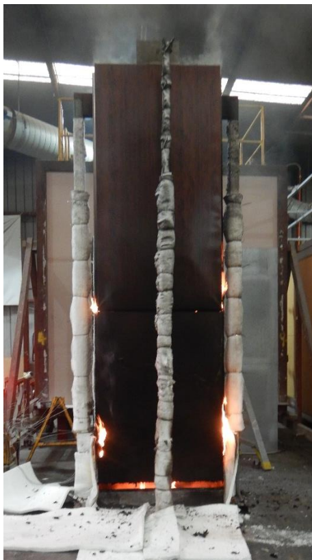
Figure 23 The specimen 42 minutes 25 seconds into the test (2 minutes 25 seconds after burner was switched off)
