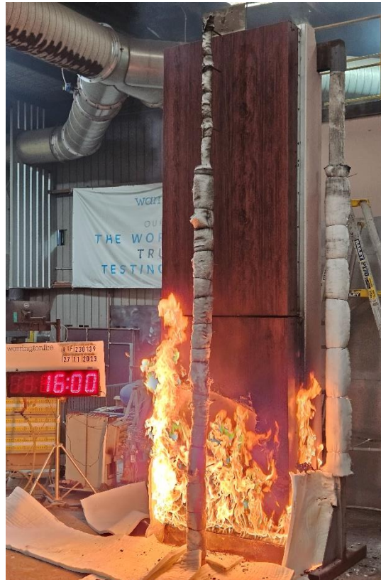
Figure 16 The specimen 16 minutes into the test (1 minute after burner output was changed to 300 kW)
