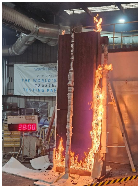
Figure 21 The specimen 38 minutes into the test (23 minutes after burner output was changed to 300 kW)
