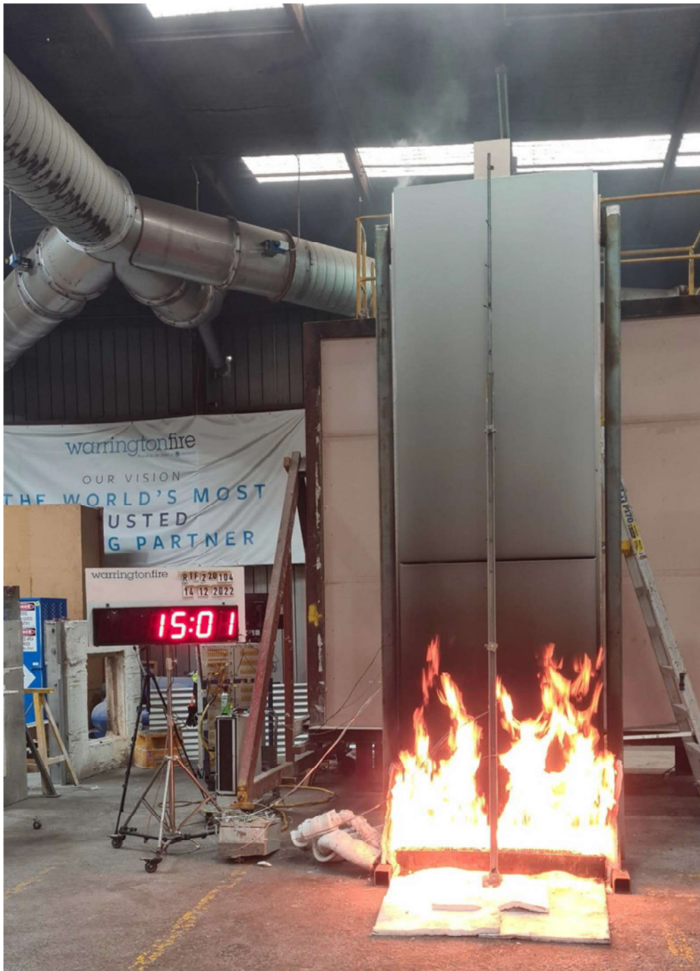
Figure 12 The specimen 15 minutes 1 second into the test (burner output at 100 kW changed to 300 kW)
