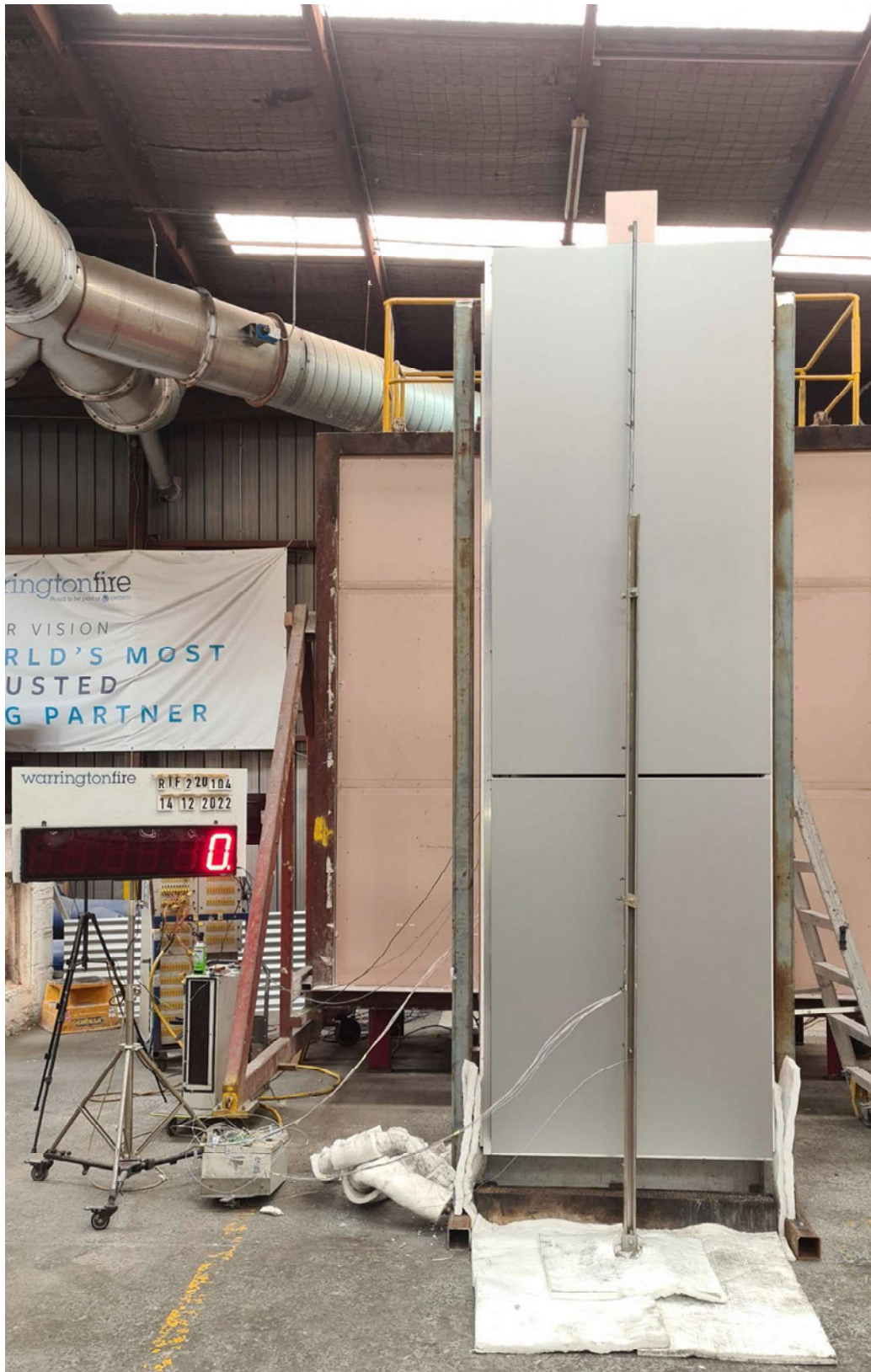
Figure 9 The specimen before the reaction to fire test
