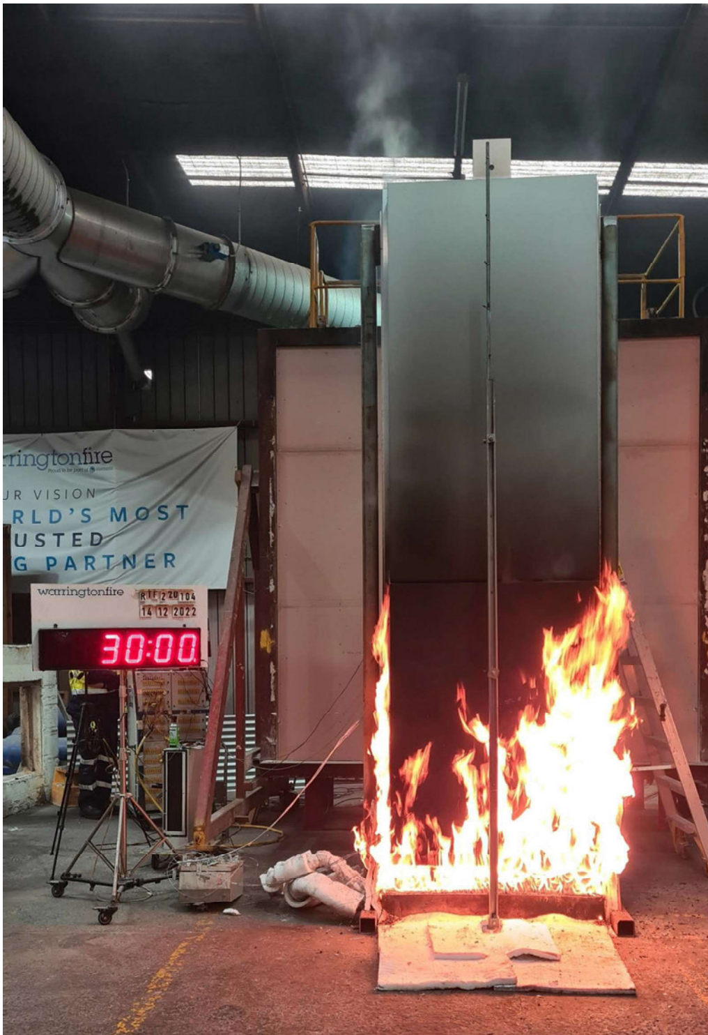
Figure 14 The specimen 30 minutes into the test (15 minutes after burner output was increased to 300 kW)
