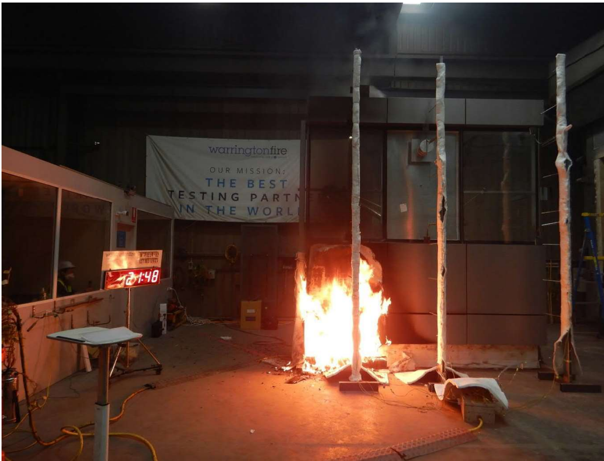
Figure 30 The specimen 21 minutes 48 seconds into the test (burner output at 300 kW).
