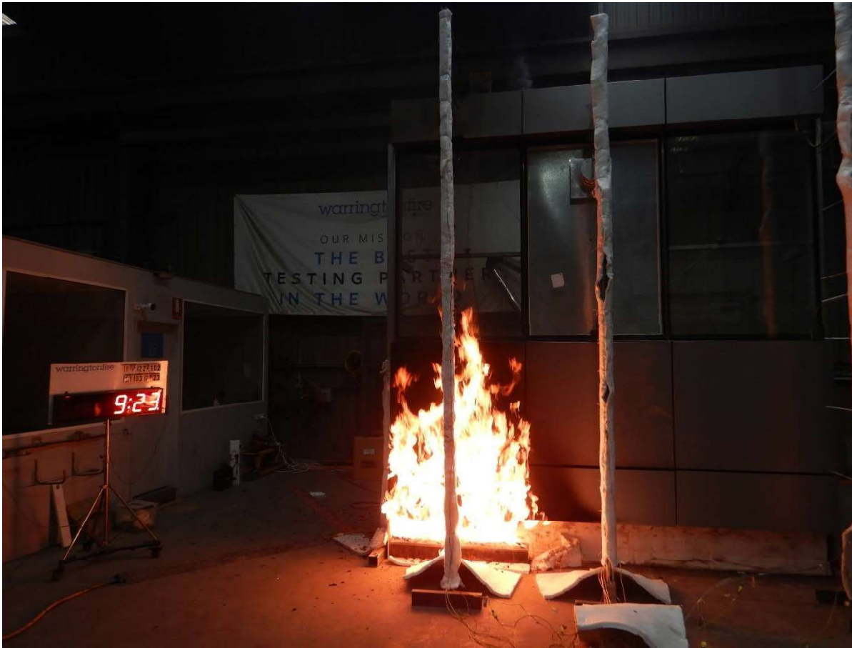
Figure 24 The specimen 9 minutes 23 seconds into the test (burner output at 300 kW)
