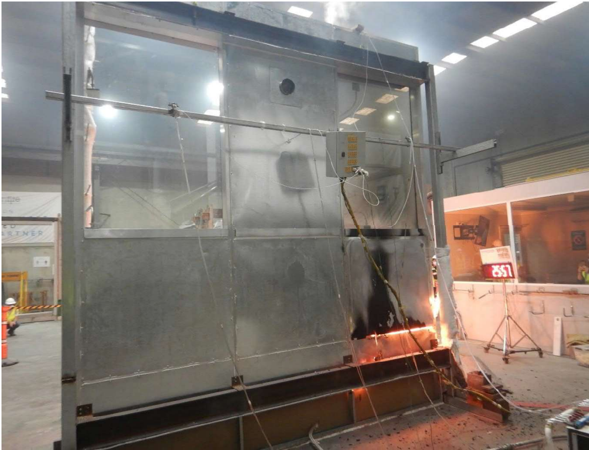
Figure 32 The specimen 25 minutes 57 seconds into the test (burner output at 300 kW) – unexposed side.
