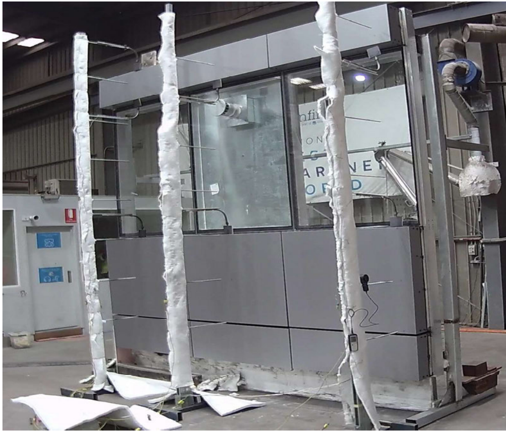
Figure 20 The specimen (angled - exposed side) before the reaction to fire test
