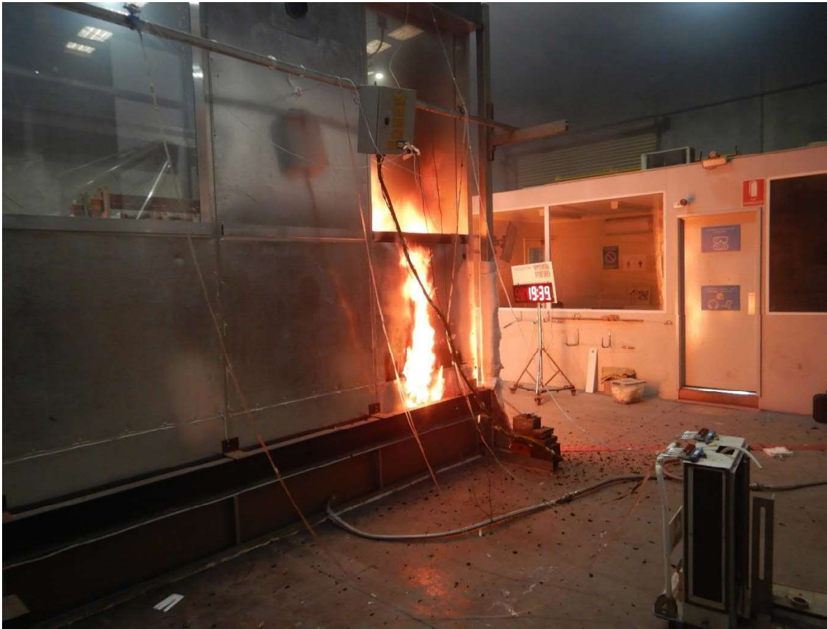
Figure 28 The specimen (unexposed side view) 19 minutes 39 seconds into the test (burner output at 300 kW).
