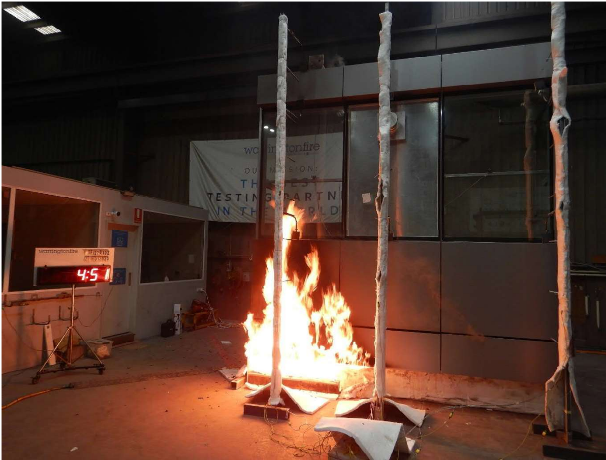
Figure 23 The specimen 4 minutes 51 seconds into the test (burner output at 300 kW)
