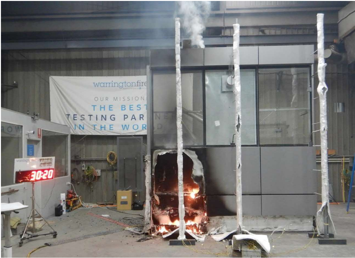
Figure 35 The specimen 30 minutes 20 seconds into the test (burner off).
