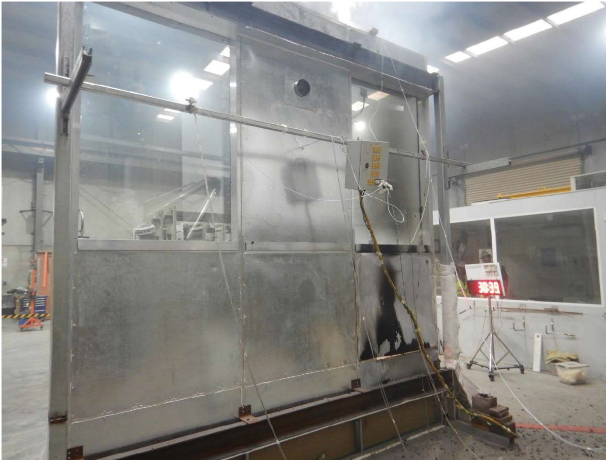
Figure 36 The specimen 30 minutes 39 seconds into the test (burner off) – unexposed side.
