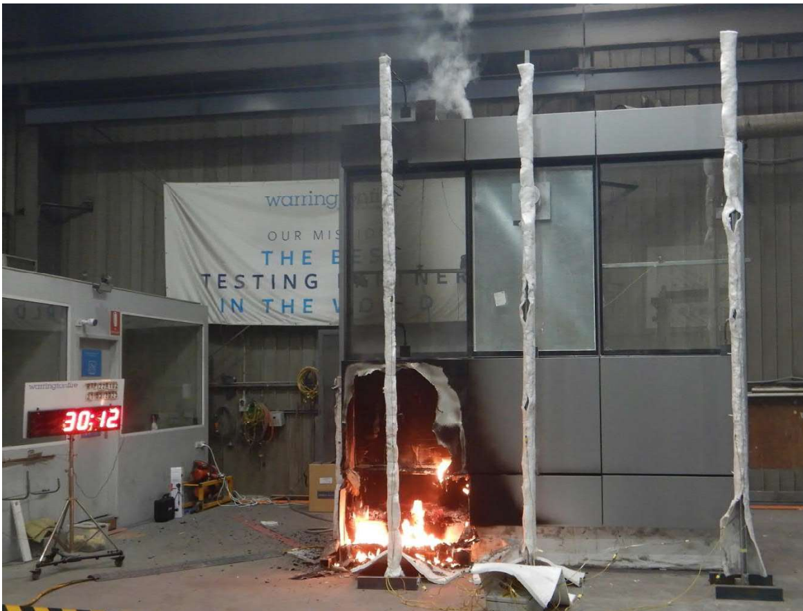
Figure 34 The specimen 30 minutes 12 seconds into the test – just after burner is turned off.
