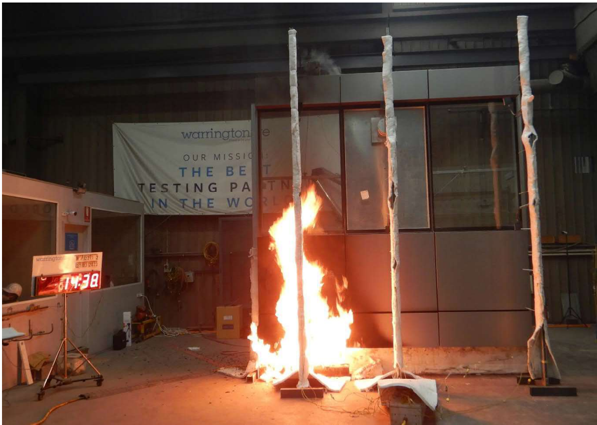
Figure 25 The specimen 14 minutes 38 seconds into the test (burner output at 300 kW)
