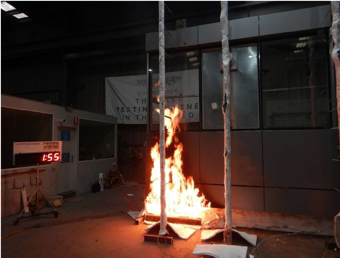
Figure 22 The specimen 1 minute 55 seconds into the test (burner output at 300 kW)
