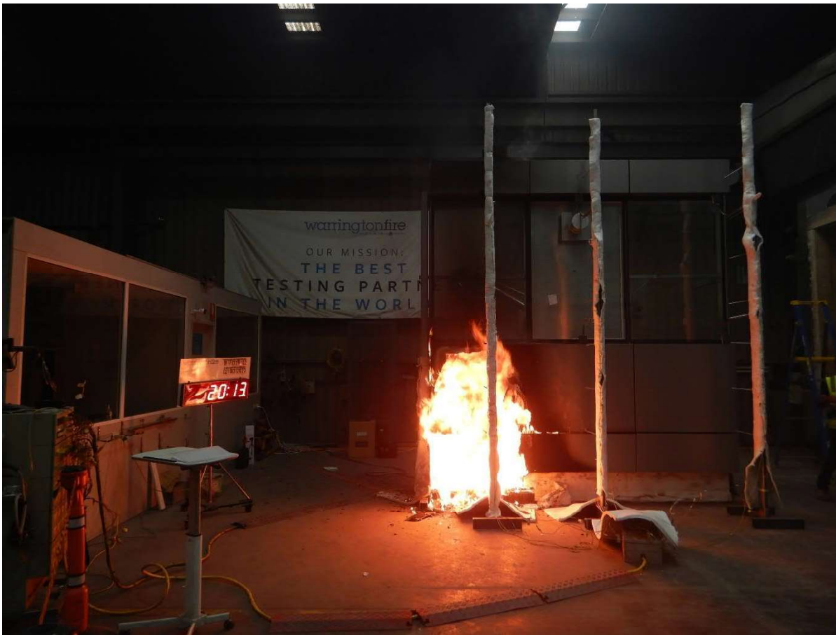
Figure 29 The specimen 20 minutes 13 seconds into the test (burner output at 300 kW).
