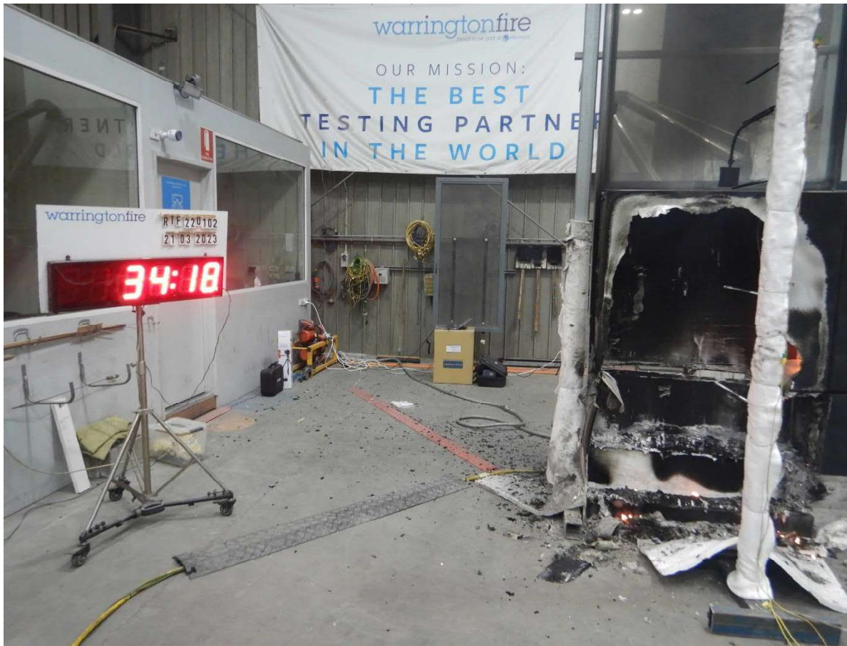
Figure 38 The specimen 34 minutes 18 seconds into the test (burner off).
