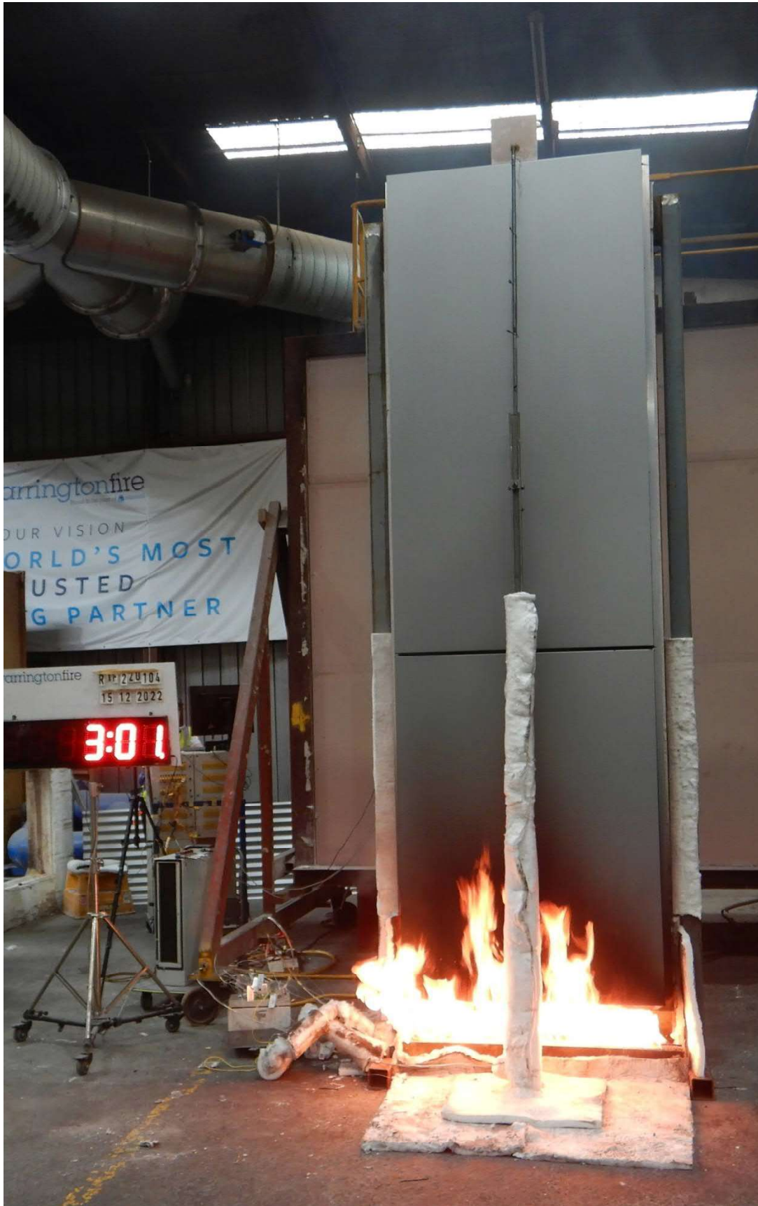
Figure 10 The specimen 3 minutes 1 second into the test (burner output at 100 kW)
