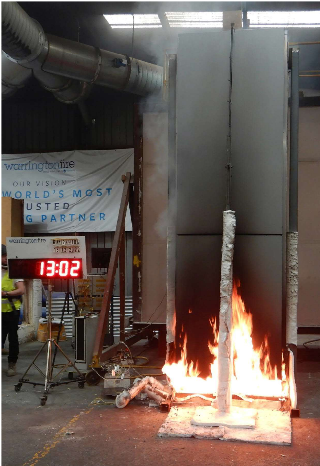
Figure 11 The specimen 13 minutes 2 seconds into the test (burner output at 100 kW)
