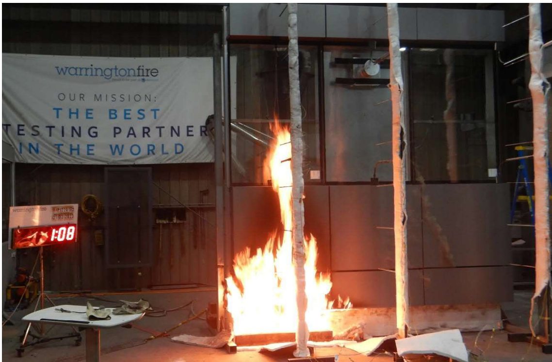
Figure 23 The specimen 1 minute 8 seconds into the test (burner output at 300 kW)
