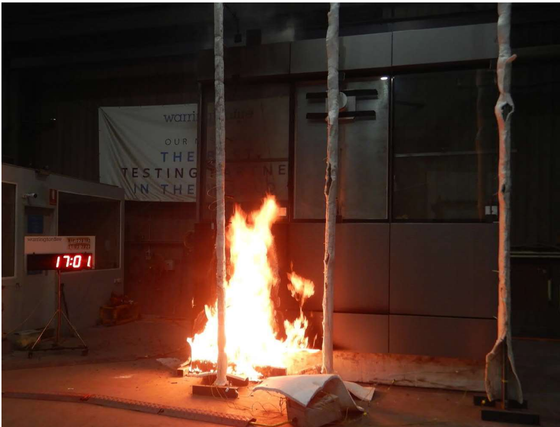
Figure 27 The specimen 17 minutes 1 second into the test (burner output at 300 kW)
