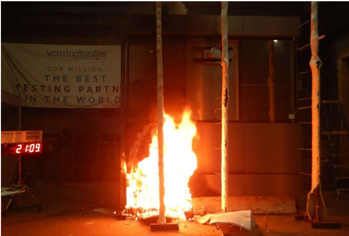
Figure 31 The specimen 28 minutes 1 seconds into the test (burner output at 300 kW).
