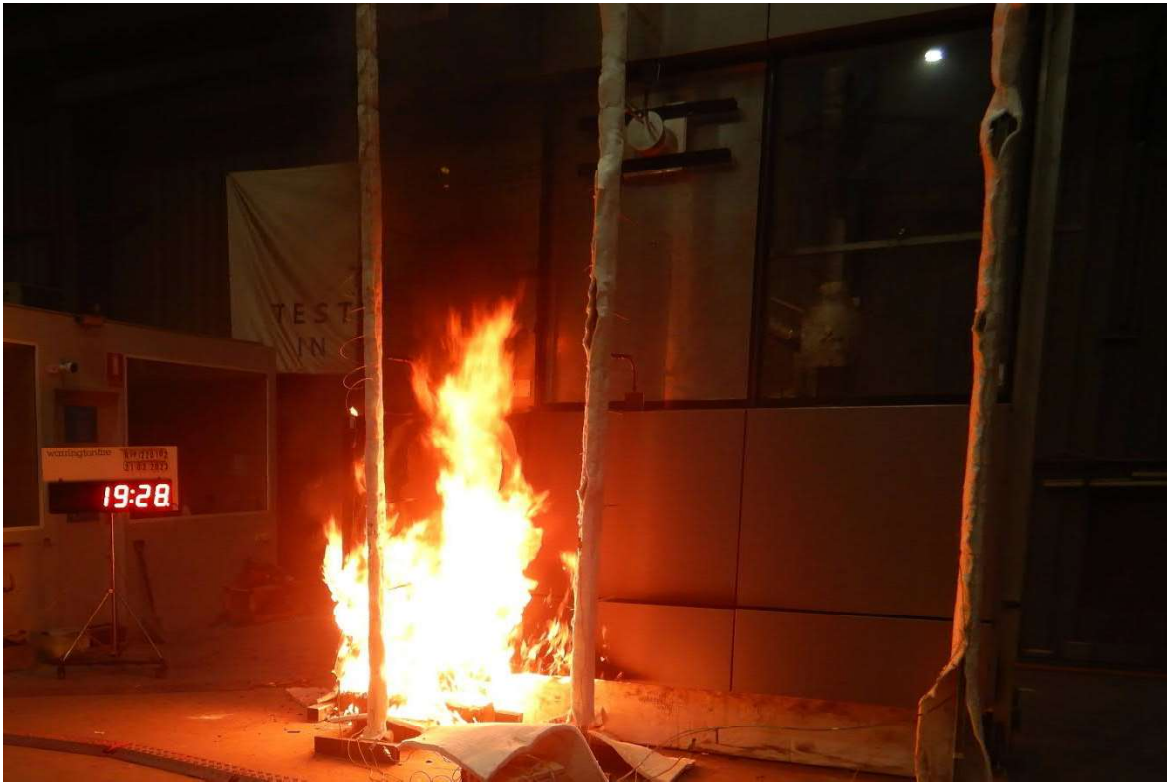
Figure 30 The specimen 25 minutes 39 seconds into the test (burner output at 300 kW).
