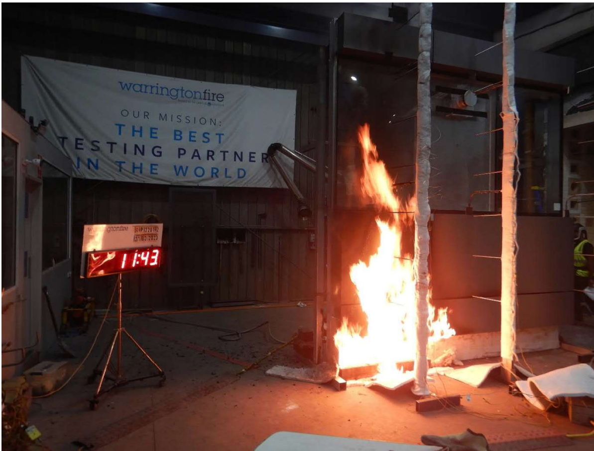
Figure 25 The specimen 11 minutes 43 seconds into the test (burner output at 300 kW)
