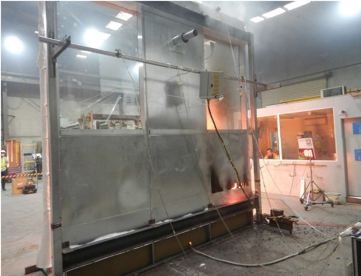
Figure 28 The specimen 17 minutes 17 seconds into the test (burner output at 300 kW) – unexposed side.
