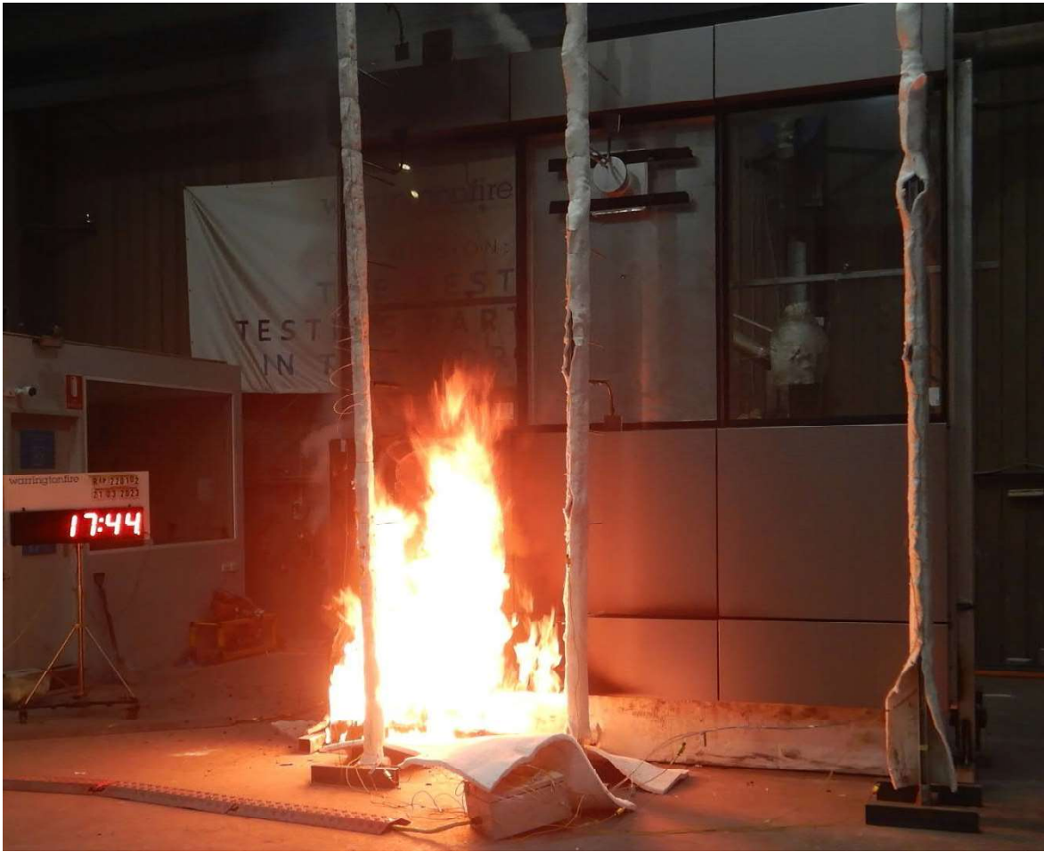
Figure 29 The specimen 17 minutes 44 seconds into the test (burner output at 300 kW).
