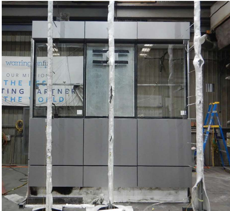
Figure 20 The specimen (exposed side) before the reaction to fire test
