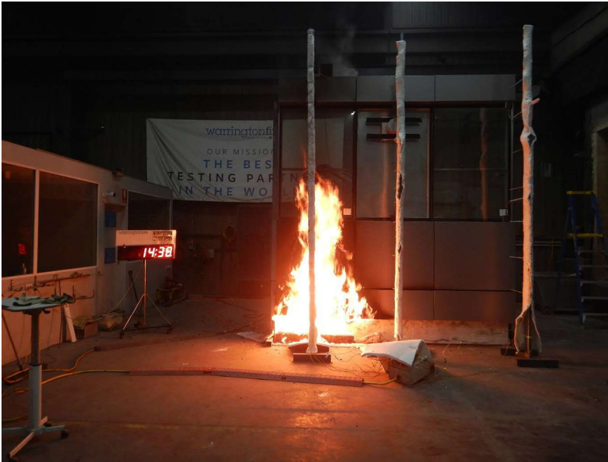
Figure 26 The specimen 14 minutes 38 seconds into the test (burner output at 300 kW)
