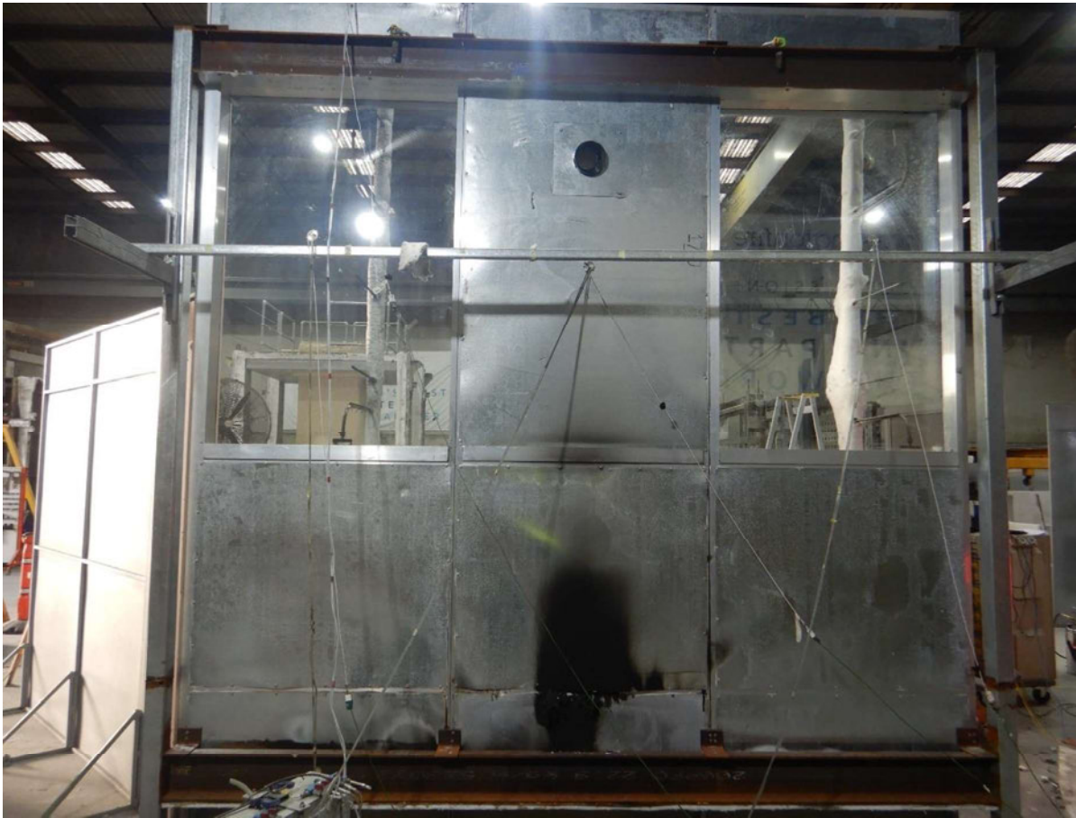
Figure 57 The specimen at the end of test – unexposed side.
