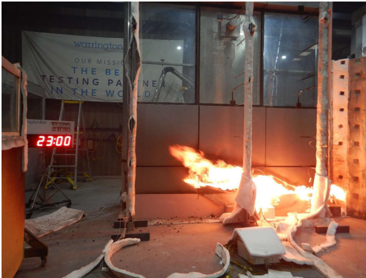
Figure 40 The specimen 23 minutes into the test (burner output at 300 kW and wind on).
