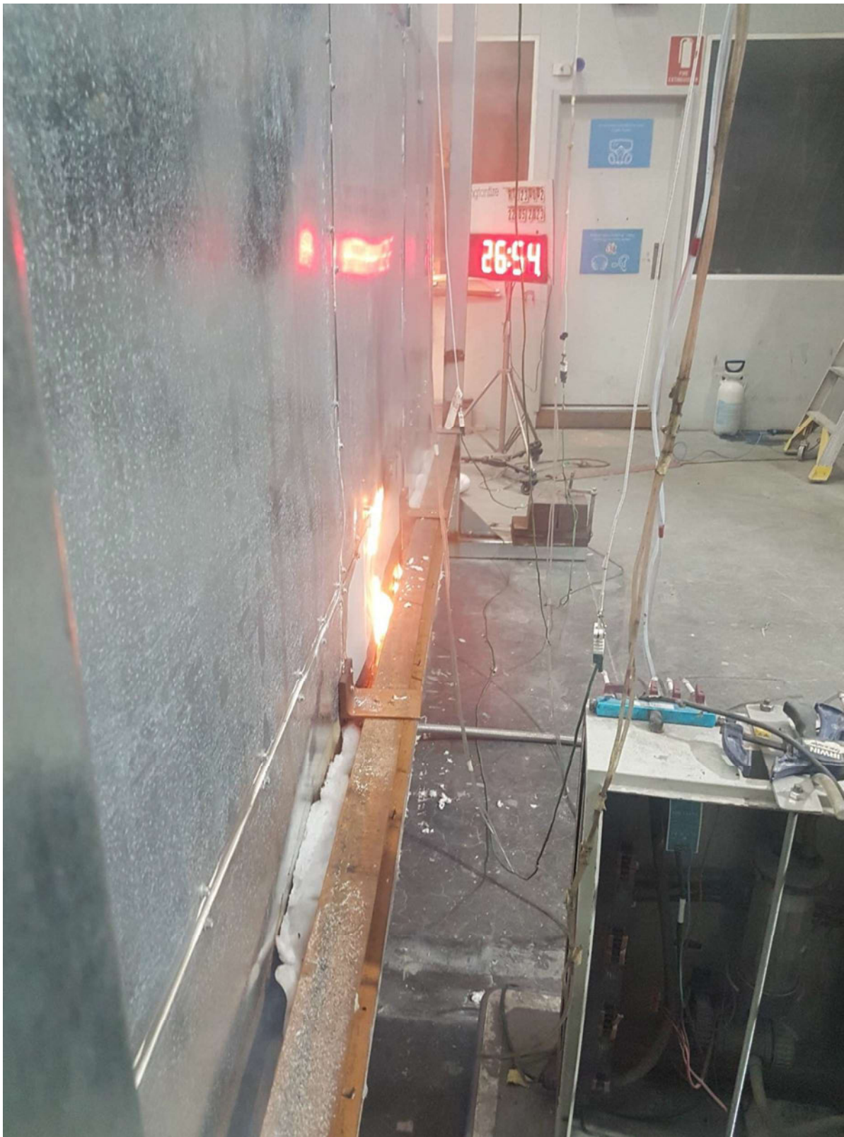
Figure 42 The specimen 26 minutes 54 seconds into the test (burner output at 300 kW and wind on) – unexposed side.
