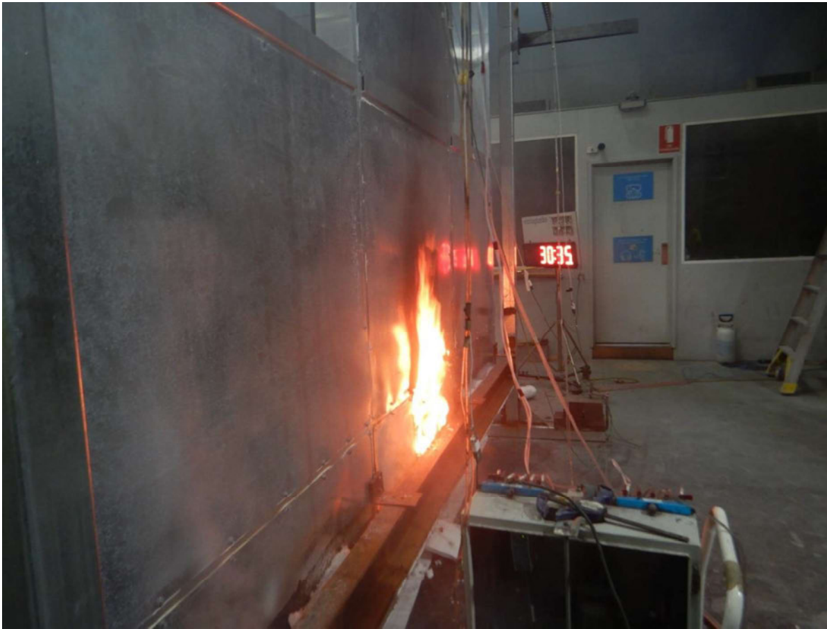
Figure 52 The specimen 30 minutes 35 seconds into the test –burner off – unexposed side.
