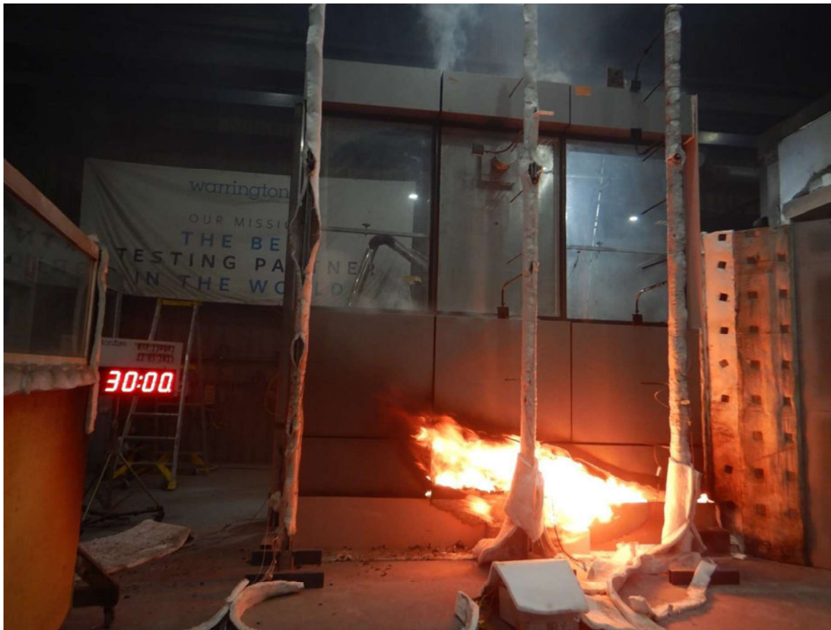
Figure 49 The specimen 30 minutes into the test (burner output at 300 kW and wind on).
