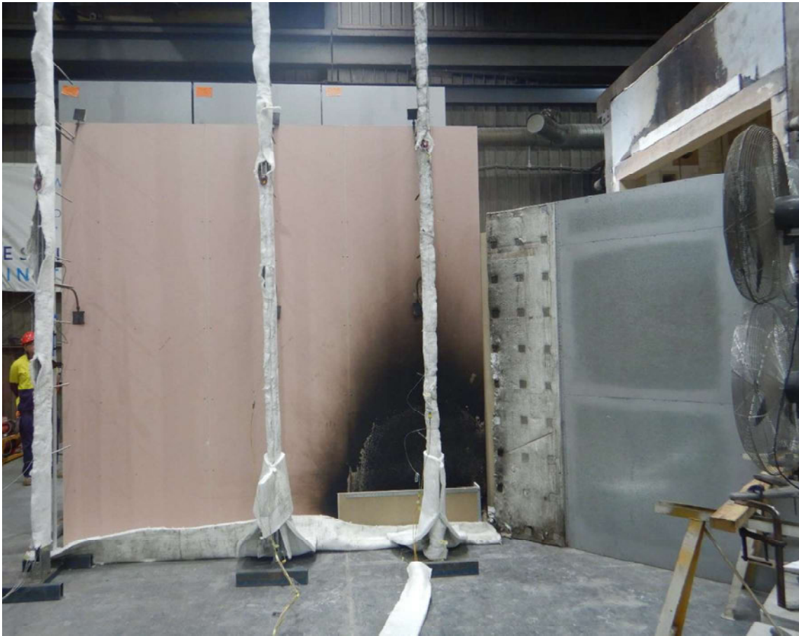
Figure 5 Photograph of baseline setup – 1.5 mm MIMS thermocouples were measuring 60 mm from the plasterboard.
