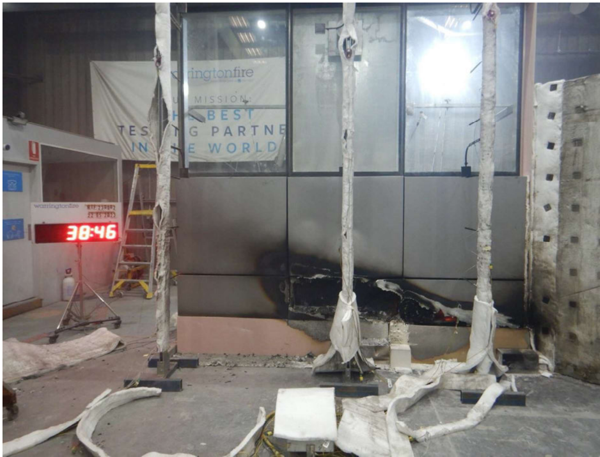
Figure 54 The specimen 38 minutes 46 seconds into the test (burner off).
