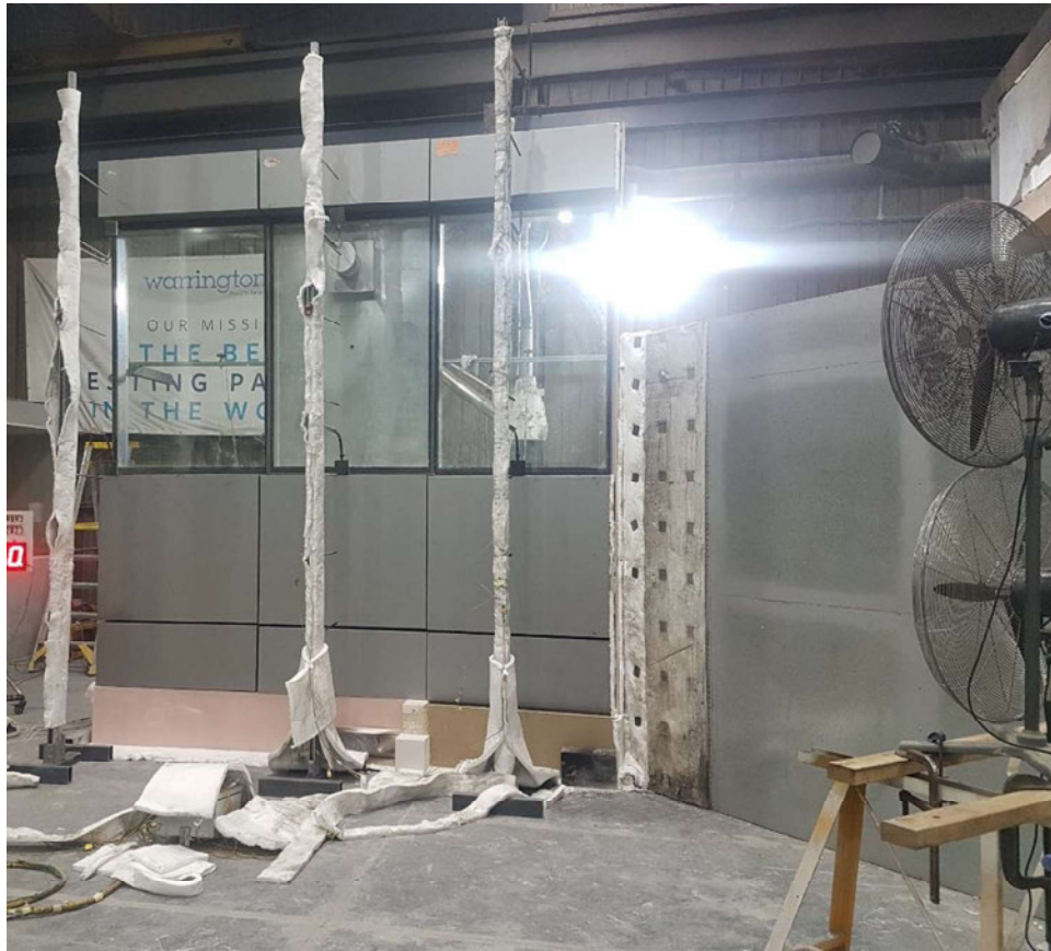
Figure 29 The specimen and test setup (angled - exposed side) before the reaction to fire test
