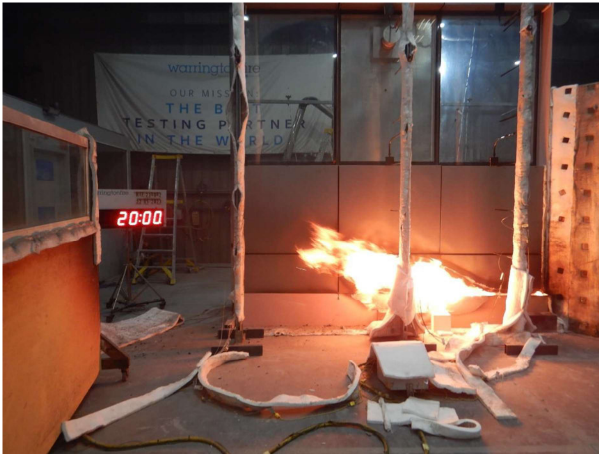
Figure 39 The specimen 20 minutes into the test (burner output at 300 kW and wind on).
