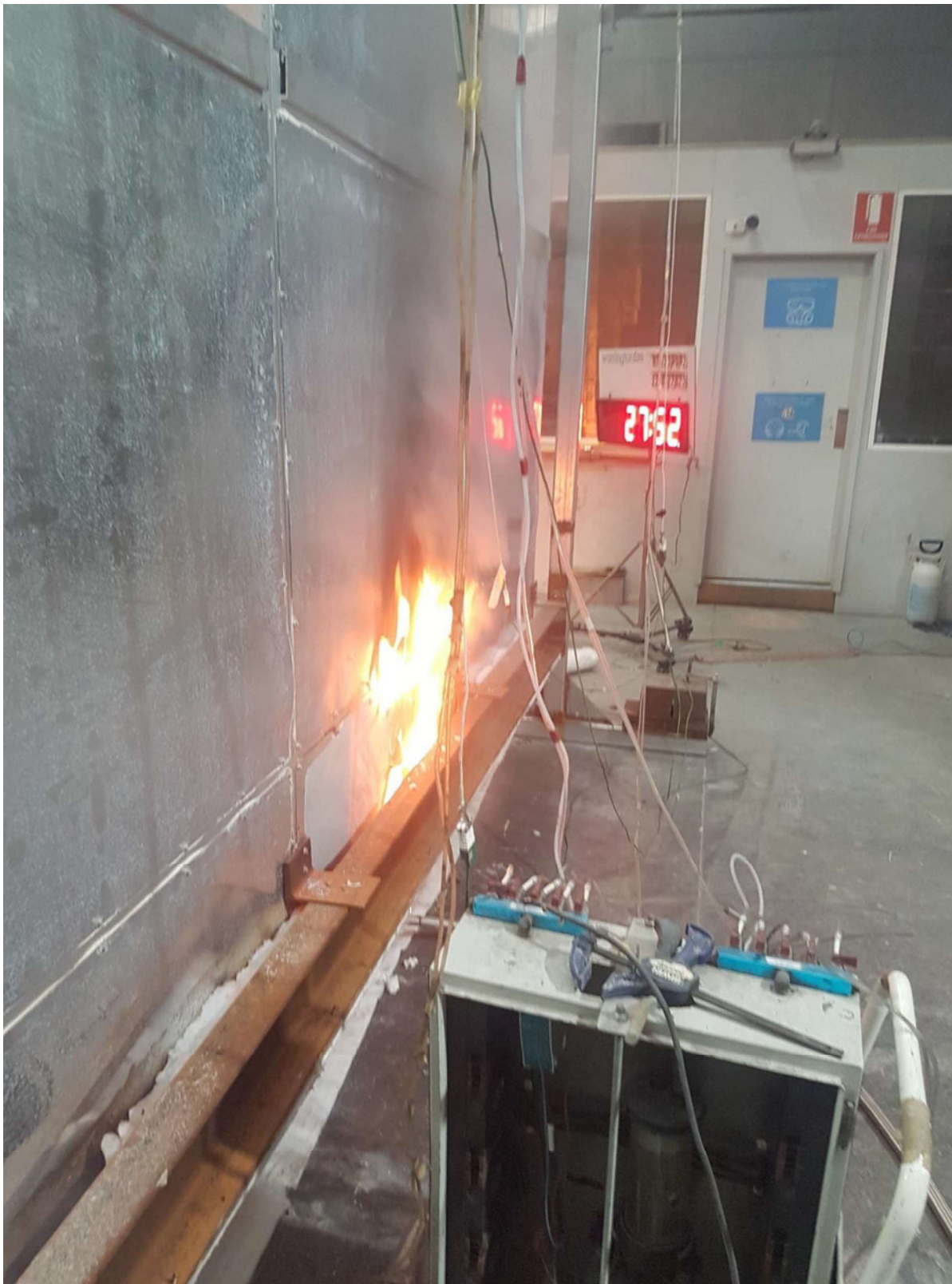
Figure 46 The specimen 27 minutes 52 seconds into the test (burner output at 300 kW and wind on) – unexposed side.
