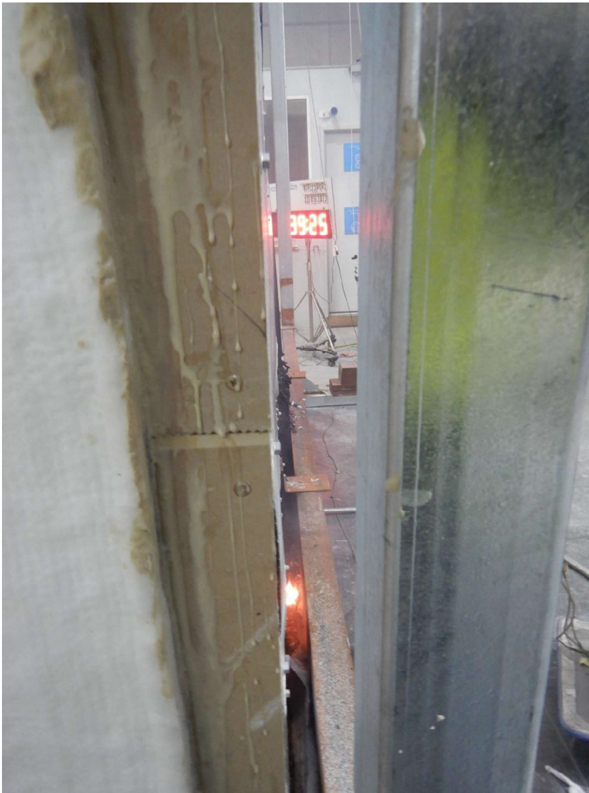
Figure 55 The specimen 39 minutes 25 seconds into the test – just after burner is turned off – unexposed side.
