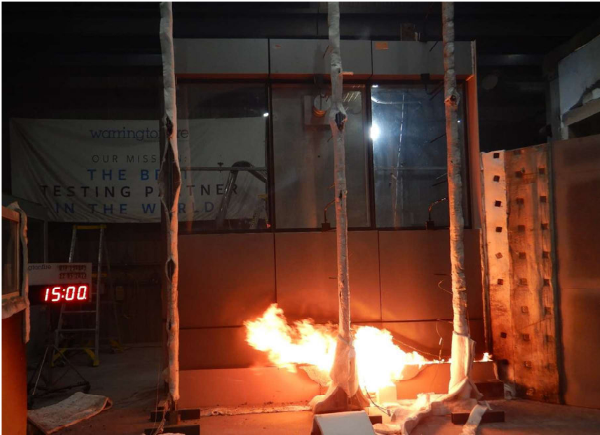
Figure 37 The specimen 15 minutes into the test (burner output at 300 kW and wind on).
