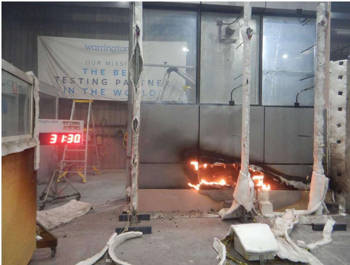
Figure 53 The specimen 31 minutes 30 seconds into the test (burner off).
