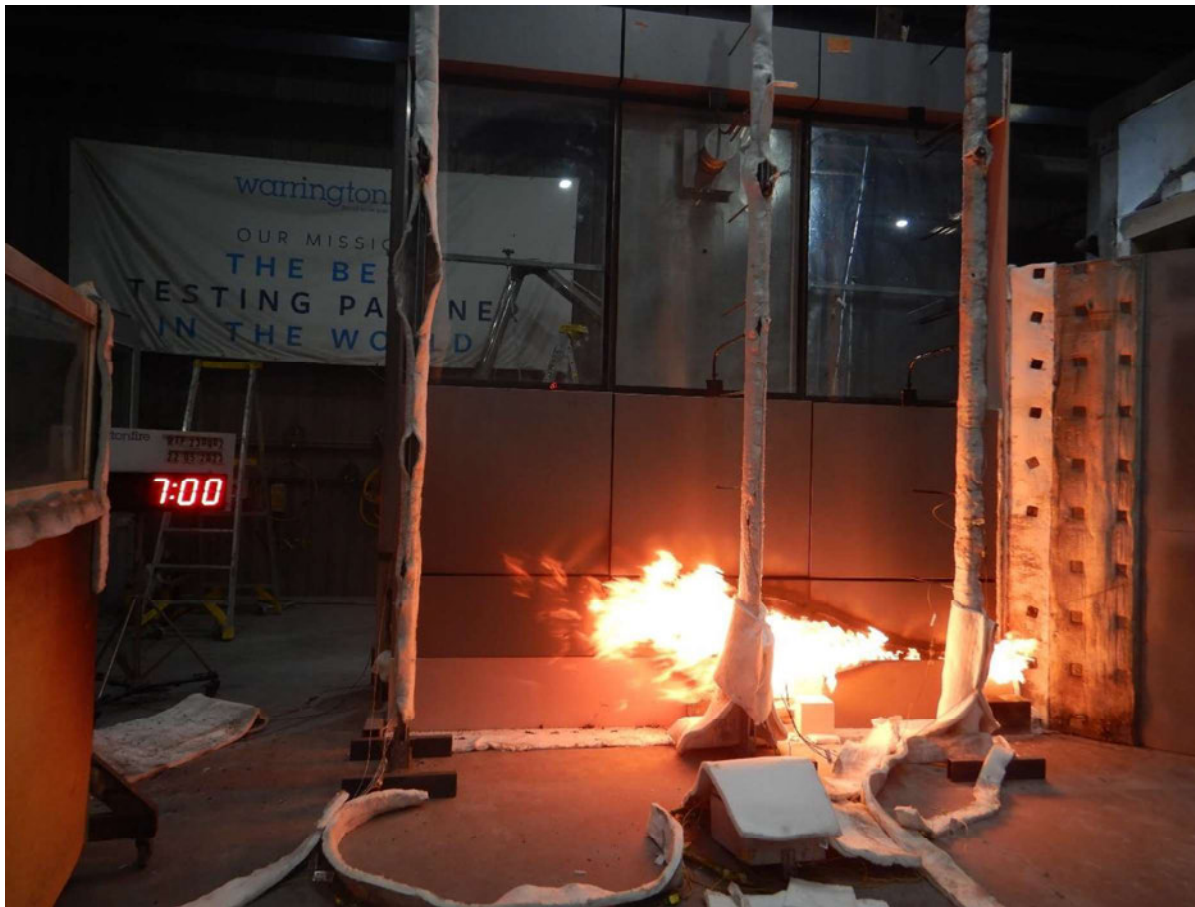
Figure 34 The specimen 7 minutes into the test (burner output at 300 kW and wind on)
