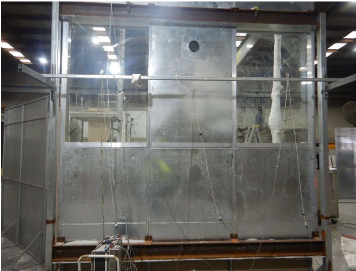
Figure 31 The specimen before the reaction to fire test - unexposed side.
