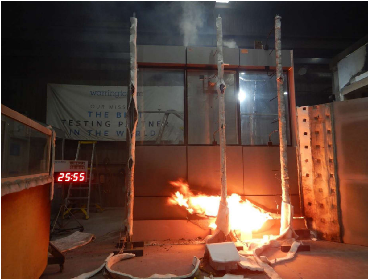
Figure 41 The specimen 25 minutes 55 seconds into the test (burner output at 300 kW and wind on).
