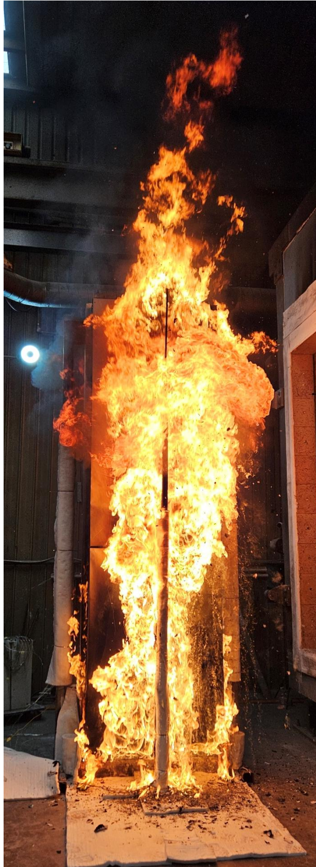
Figure 23 The specimen 17 minutes 52 seconds into the test (2 minutes 52 seconds after burner output was changed to 300 kW)
