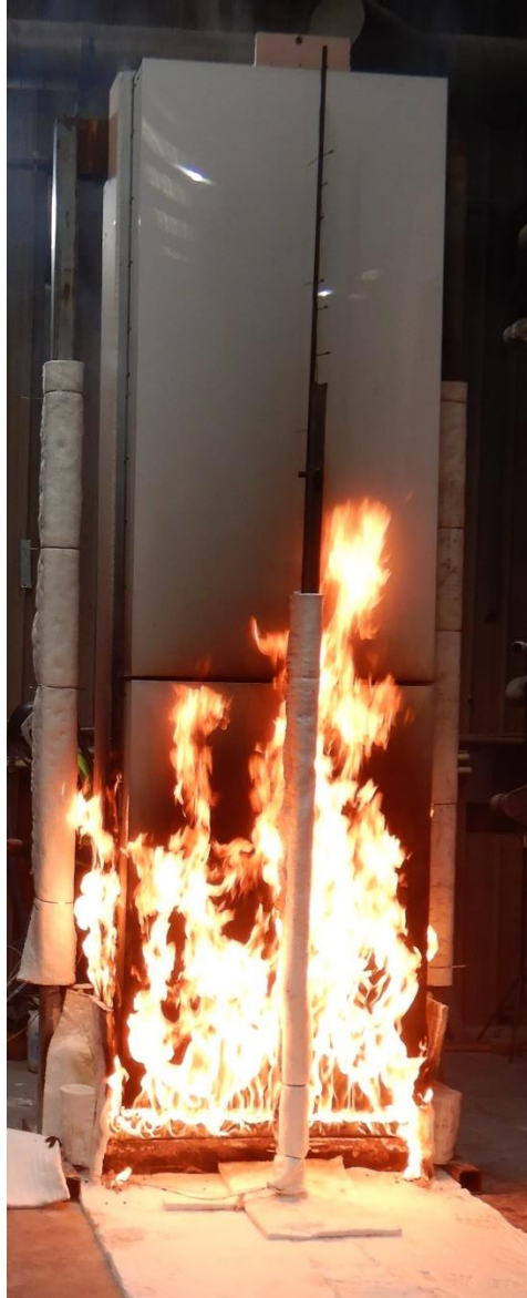
Figure 19 The specimen 15 minutes 41 seconds into the test (41 seconds after burner output was changed to 300 kW)
