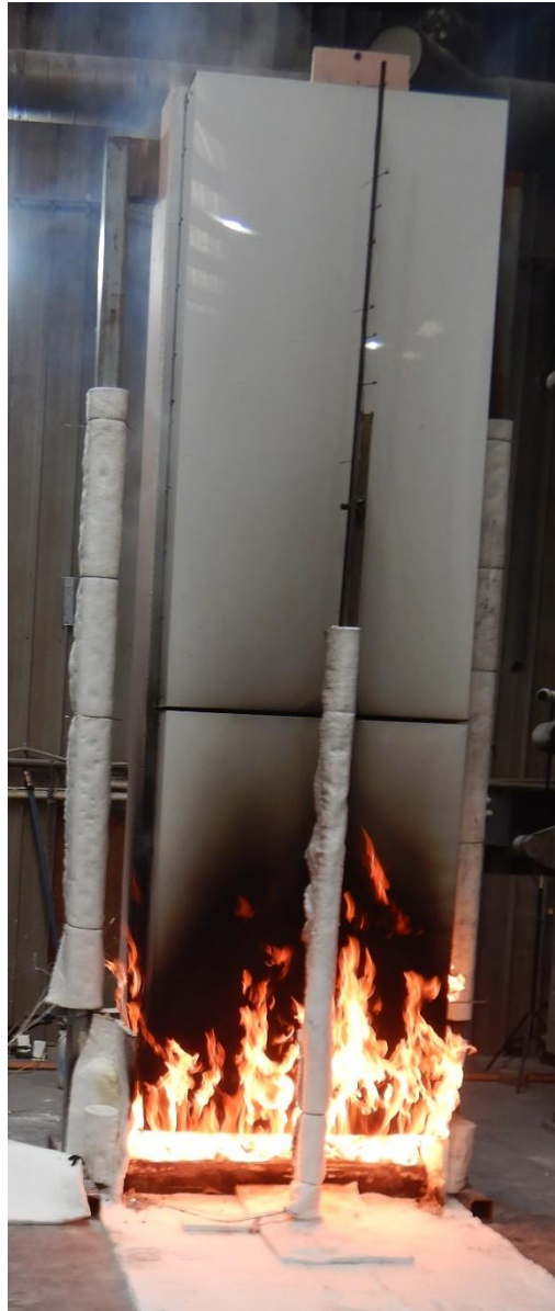
Figure 17 The specimen 14 minutes 45 seconds into the test (burner output at 100 kW)
