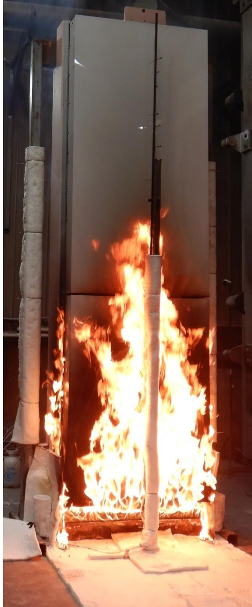
Figure 20 The specimen 15 minutes 56 seconds into the test (56 seconds after burner output was changed to 300 kW)
