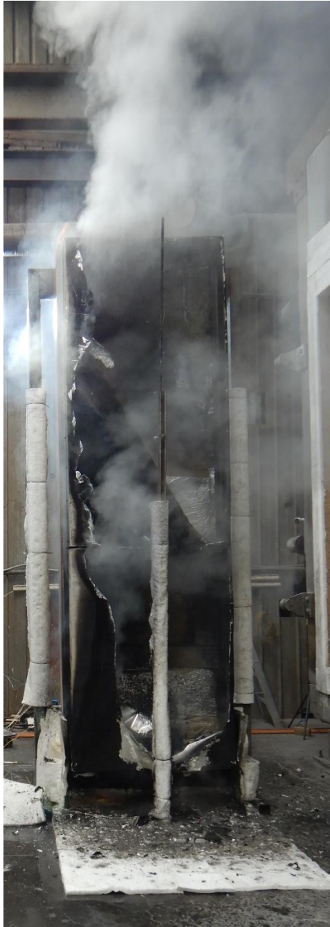
Figure 24 The specimen shortly after being sprayed with water
