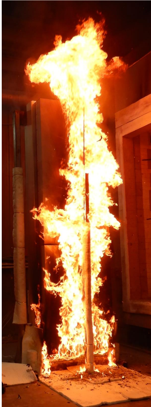
Figure 22 The specimen 17 minutes 45 seconds into the test (2 minutes 45 seconds after burner output was changed to 300 kW)
