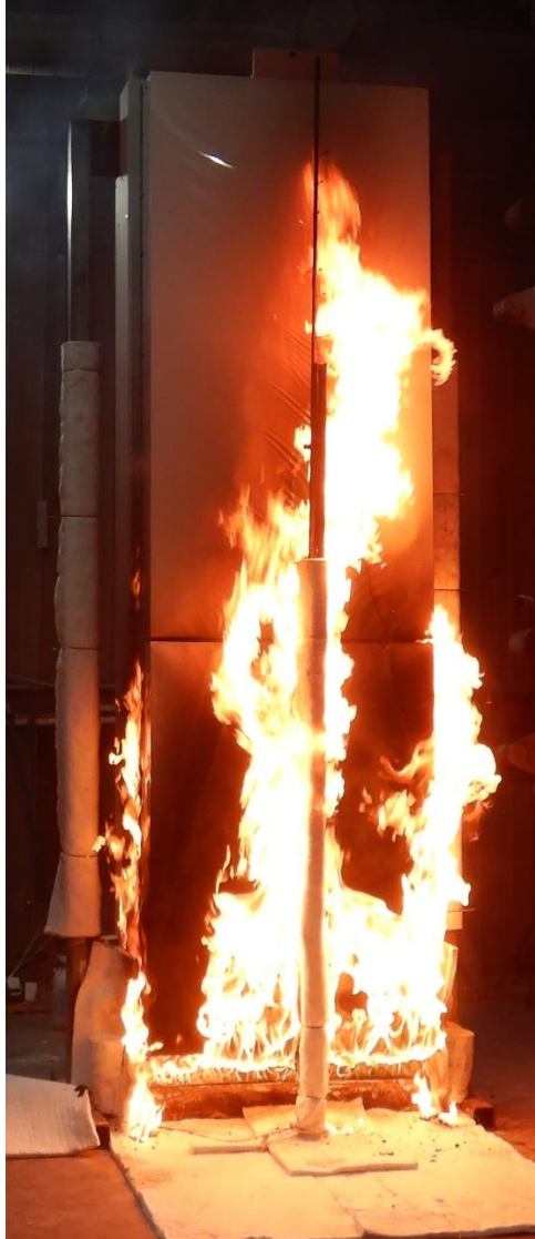
Figure 21 The specimen 16 minutes 55 seconds into the test (1 minute 55 seconds after burner output was changed to 300 kW)
