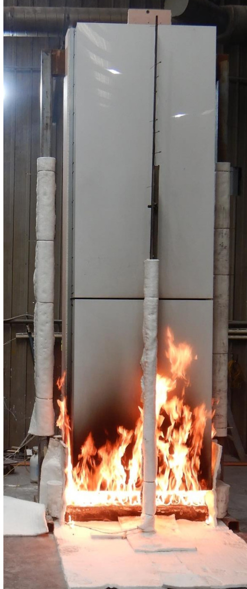
Figure 13 The specimen 3 minutes 11 seconds into the test (burner output at 100 kW)
