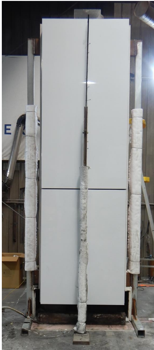
Figure 10 The specimen before the reaction to fire test
