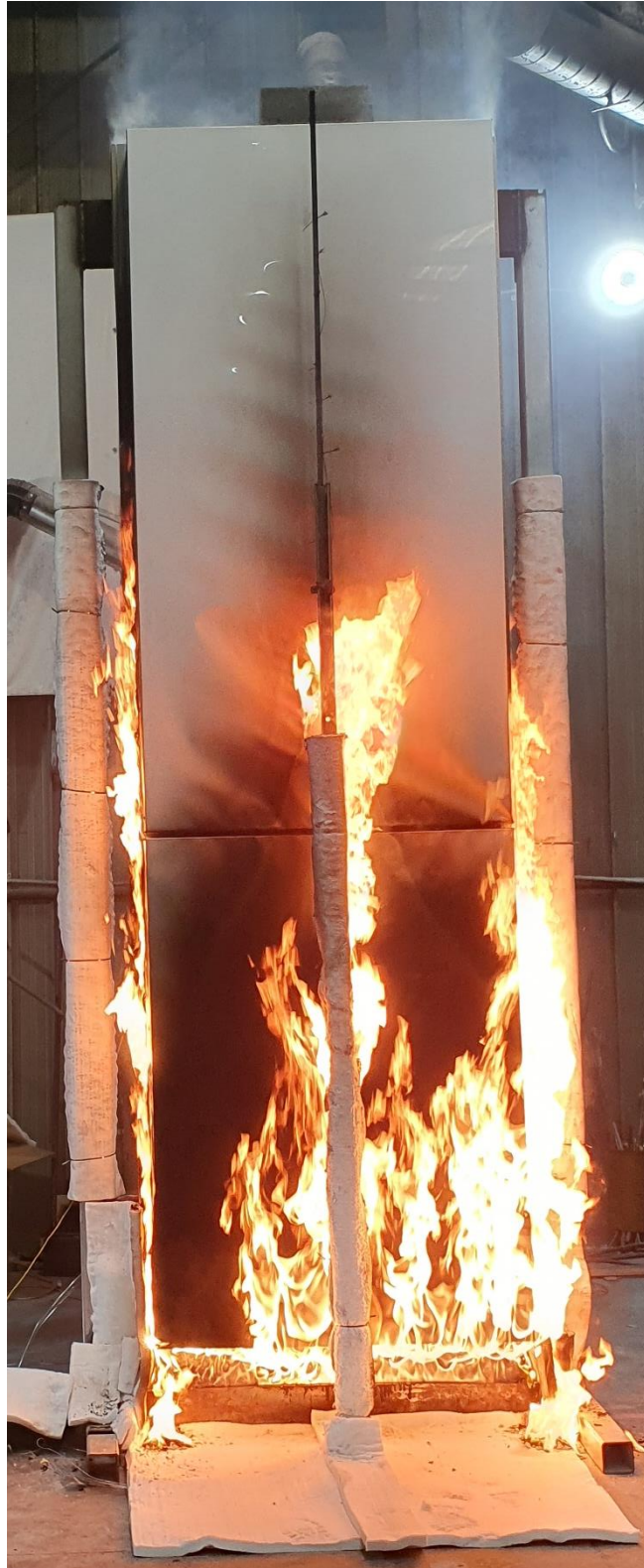
Figure 16 The specimen 13 minutes into the test (burner output at 200 kW)
