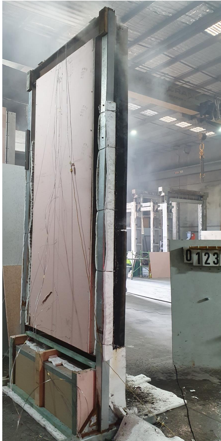
Figure 25 The specimen after the test – unexposed side.
