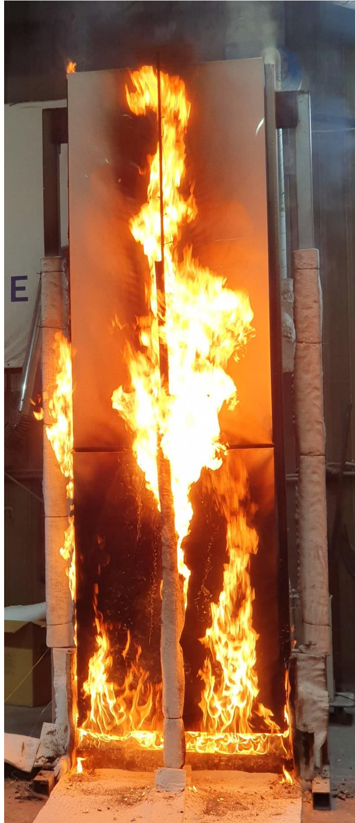
Figure 20 The specimen 20 minutes into the test (burner output at 200 kW)
