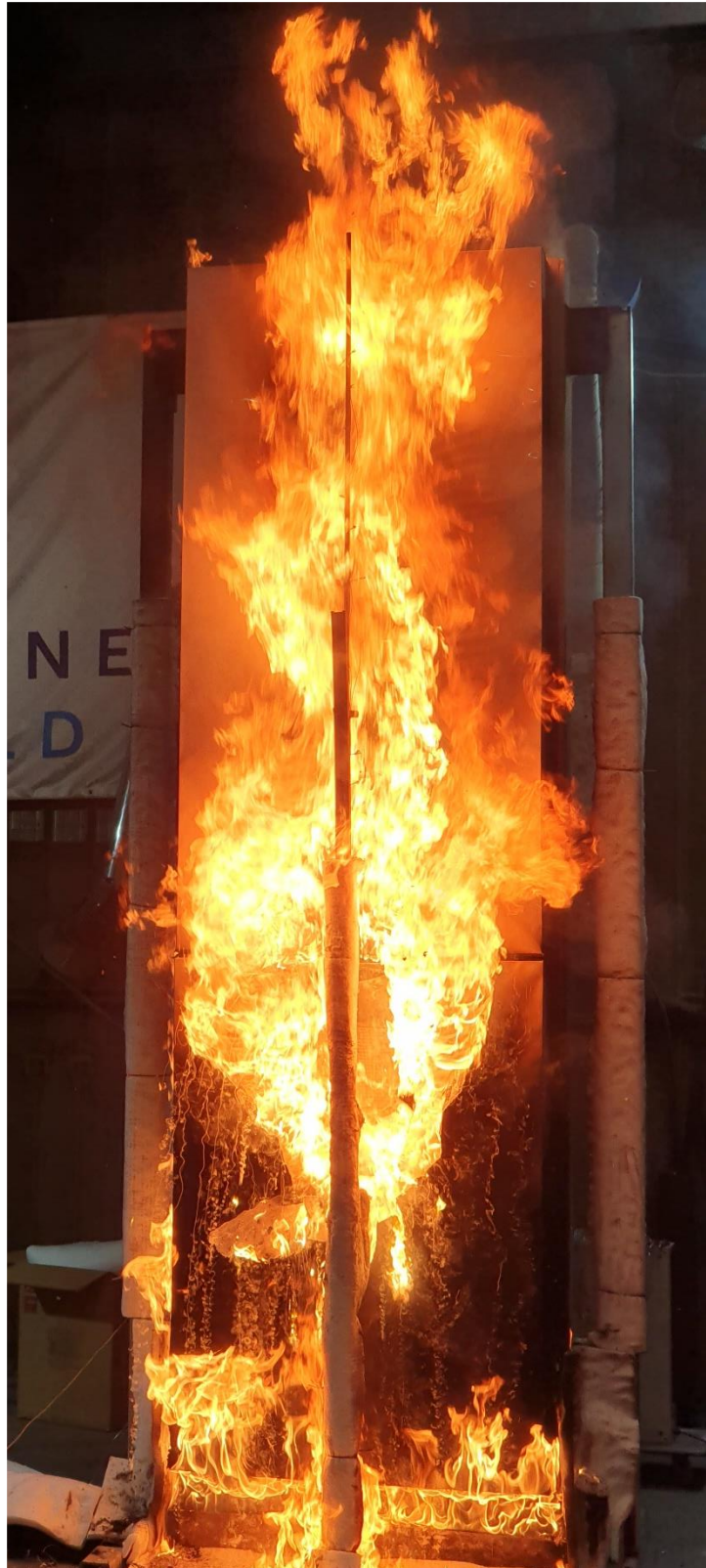
Figure 21 The specimen 20 minutes 33 seconds into the test (burner output at 200 kW)
