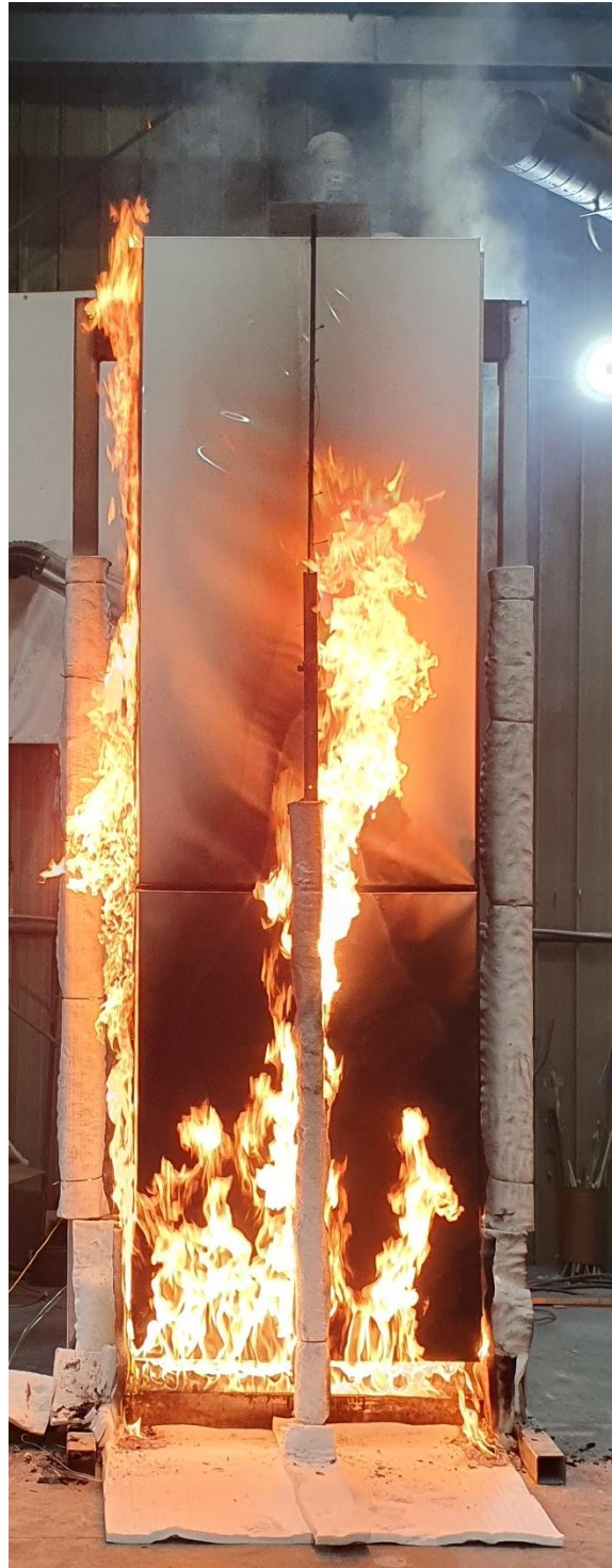
Figure 18 The specimen 17 minutes 30 seconds into the test (burner output at 200 kW)
