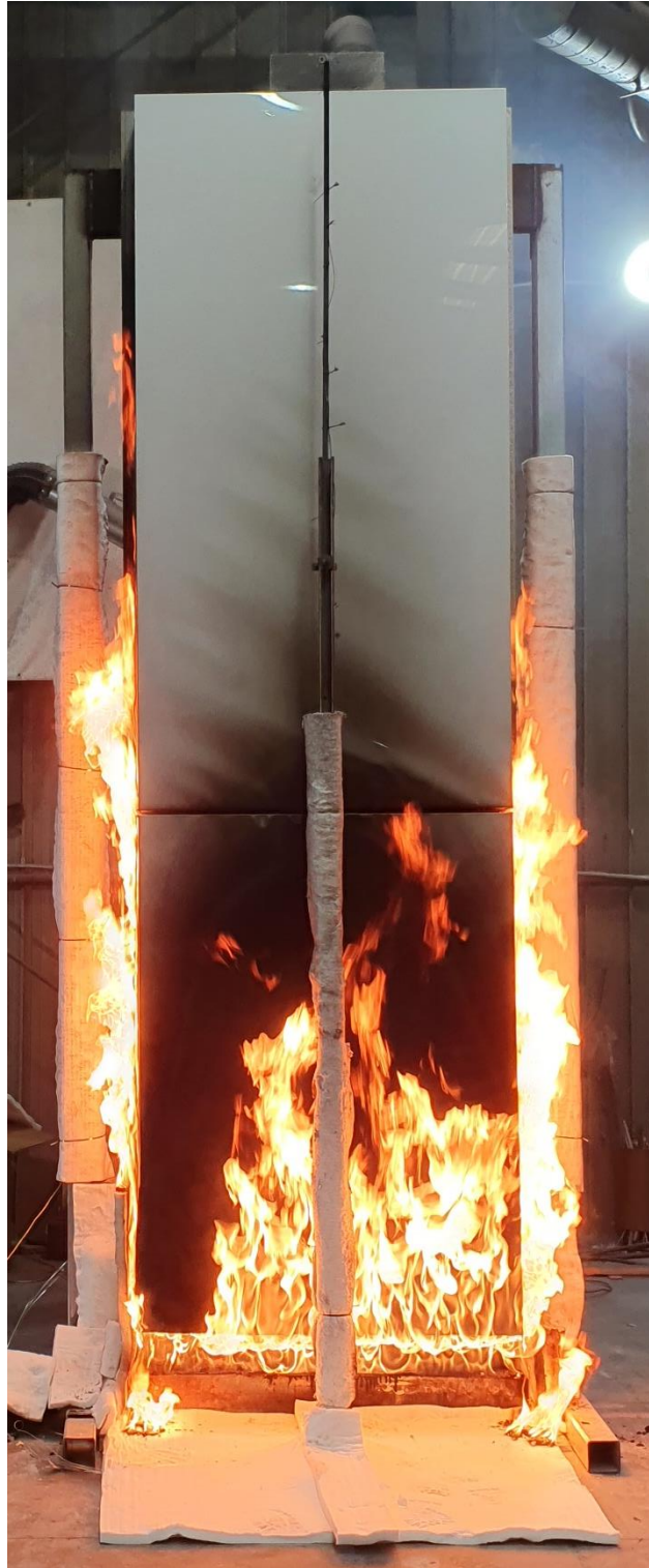
Figure 15 The specimen 10 minutes into the test (burner output at 200 kW)
