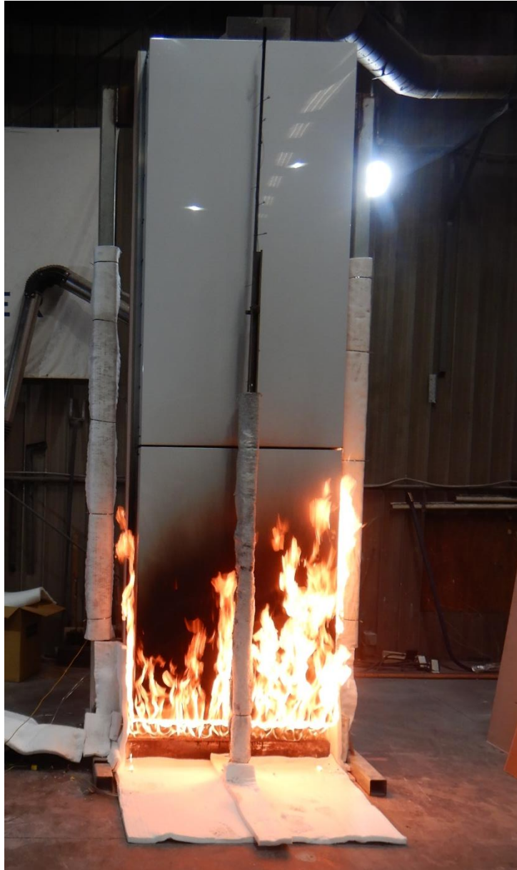
Figure 12 The specimen 2 minute 47 seconds into the test (burner output at 200 kW)
