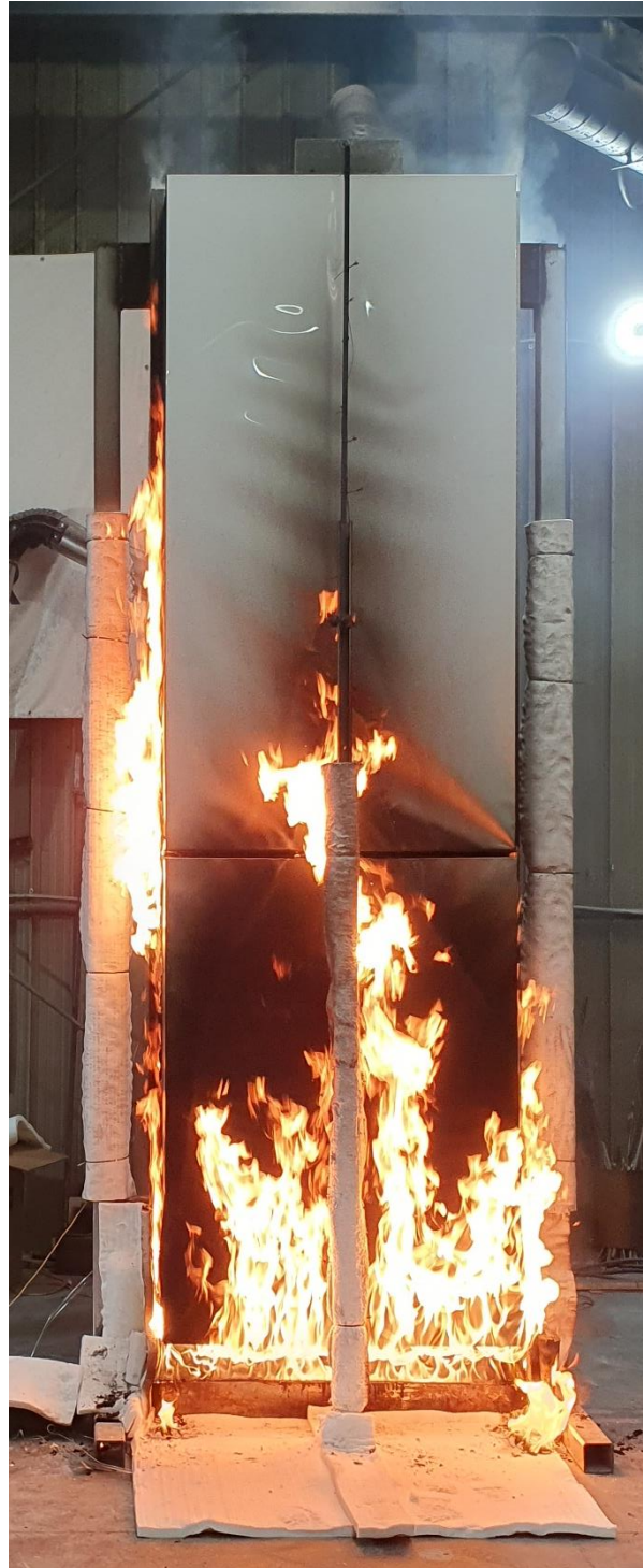
Figure 17 The specimen 15 minutes into the test (burner output at 200 kW)
