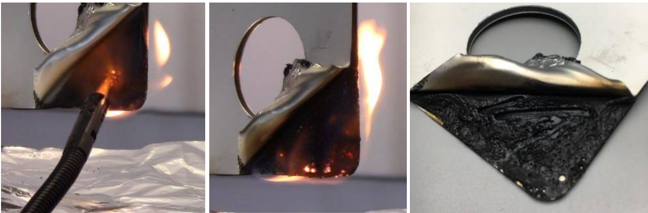
Figure 20 PE ACP with minor mineral filler content (not quantified but significantly < 70% mineral filler, Left -butane flame applied for 30 s, Centre – 20 s after butane flame removed, Right- damage – note core was probed post test to observe viscosity (all photos by CSIRO)
