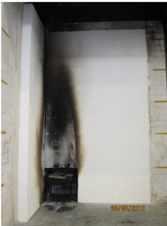
Figure 73. DIN 4102-20 (Draft) test rig (From BRE Global [118] )
