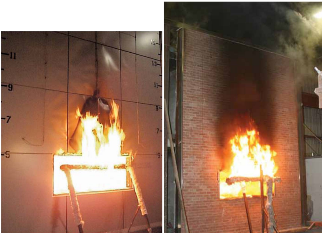
Figure 75. Front view of typical NFPA 285 test (from Hansbro [121] )
