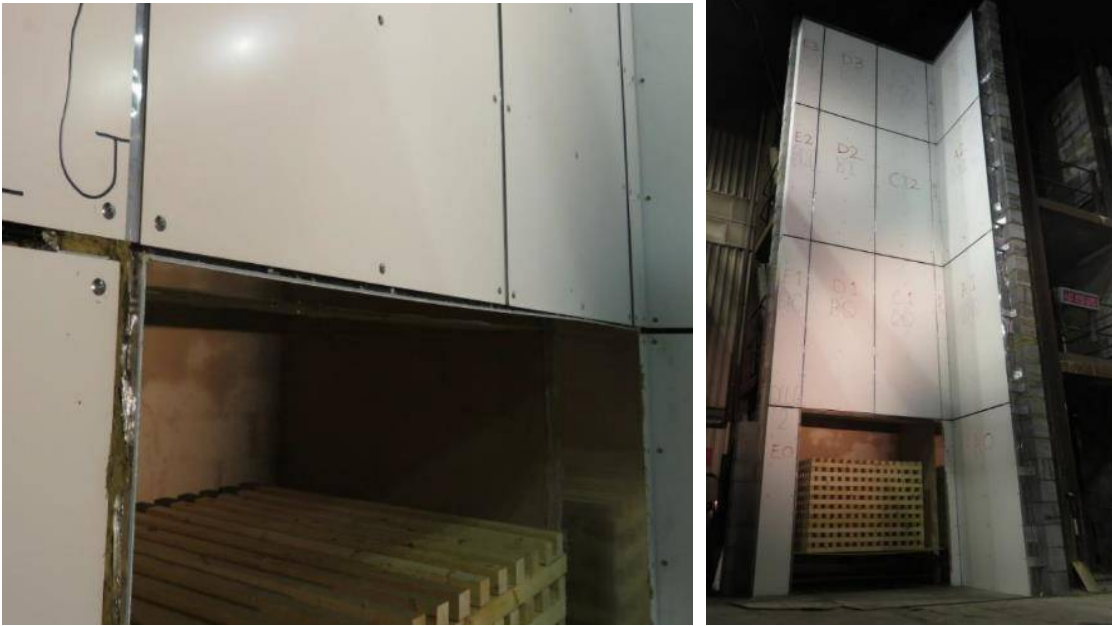
Figure 46. Left – Aluminium window pod, combustion chamber and ACP joints and fixing detail. Right – complete façade system prior to test (all photos taken from BRE Test report [51] )
