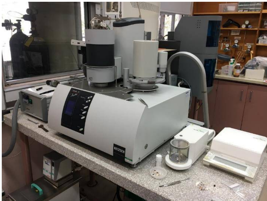
Figure 23. CSIRO's TGA-DSC which has been used in past ACP analysis (but we now use mostly ashing test with XRD). Photo by CSIRO
