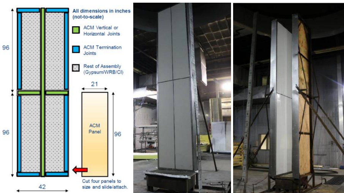
Figure 41. FM Global 16ft PPT test set up (all images taken from FM Global report [50] )
