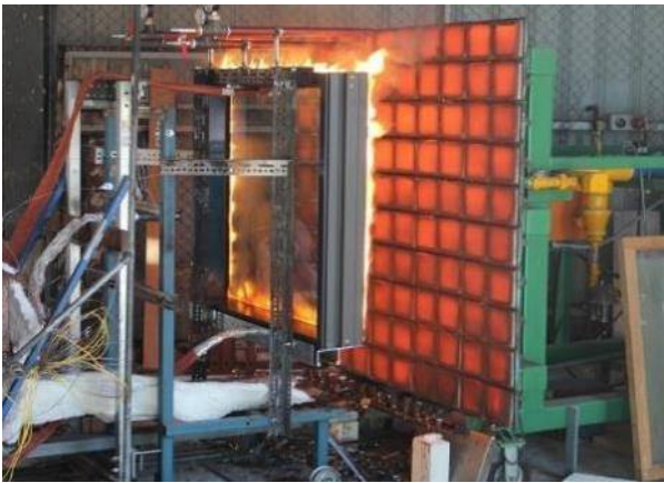
Figure 65. CSIRO pilot scale AS 1530.8.1 test (left), BAL radiant heat test profiles (right)
