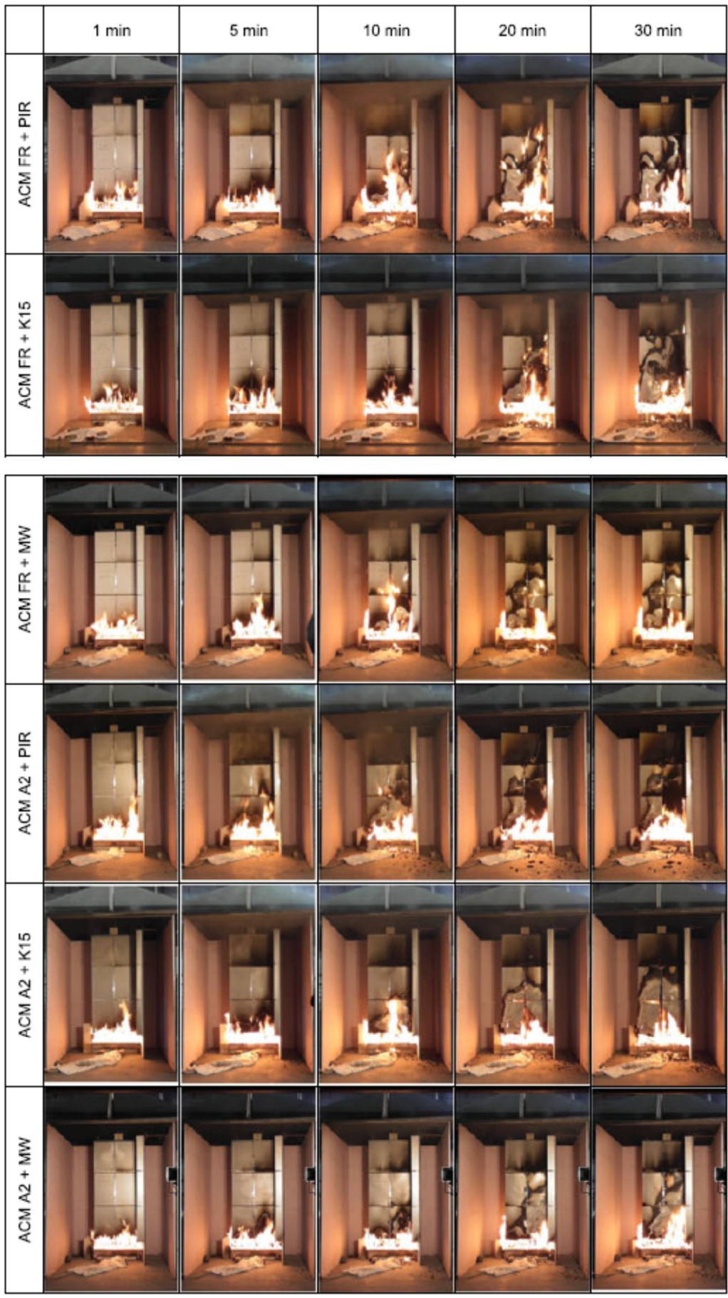
Figure 39. Test Photographs comparing ACM FR and ACM A2 tests by Guillaume et al [49]
