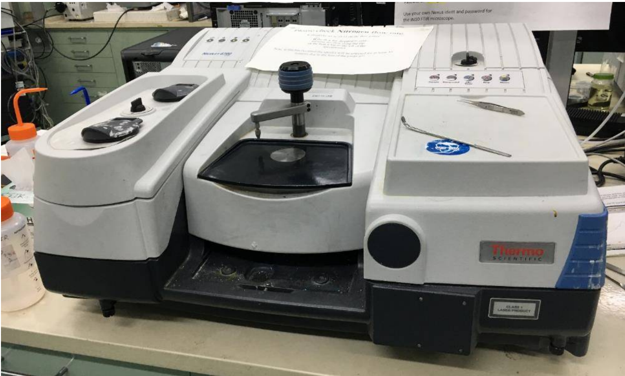
Figure 25. CSIRO FTIR with Diamond ATR accessory which has been used in past ACP analysis (but we now use mostly ashing test with XRD). We continue to use ATR-FTIR for analysis of other insulation and cladding materials. (Photo by CSIRO)
