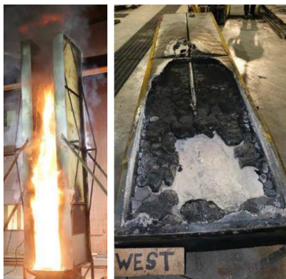
Figure 44. FM Global 16 ft PPT Tests 7 (ACP-FR/PIR2/WRB), left-peak fire size, right-damage (all photos taken from FM global report [50] )
