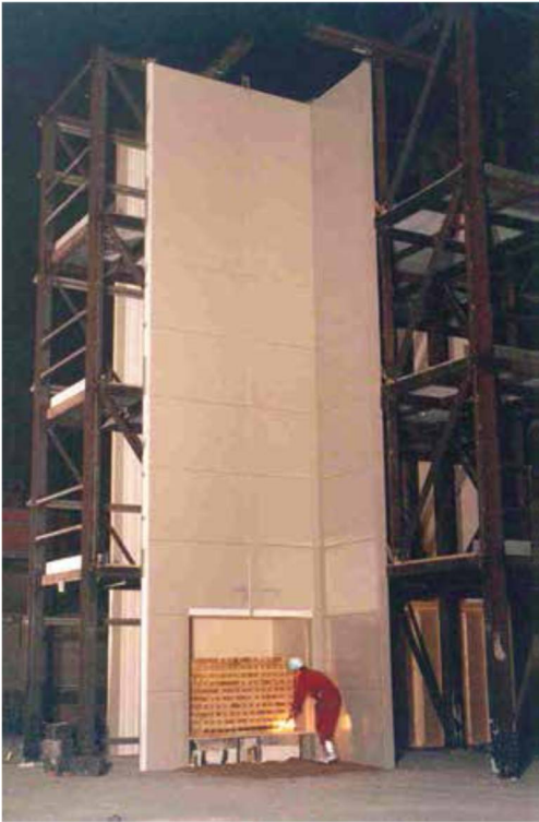
Figure 72. BS8414-2 test rig (from BRE report BR135 [116] )
