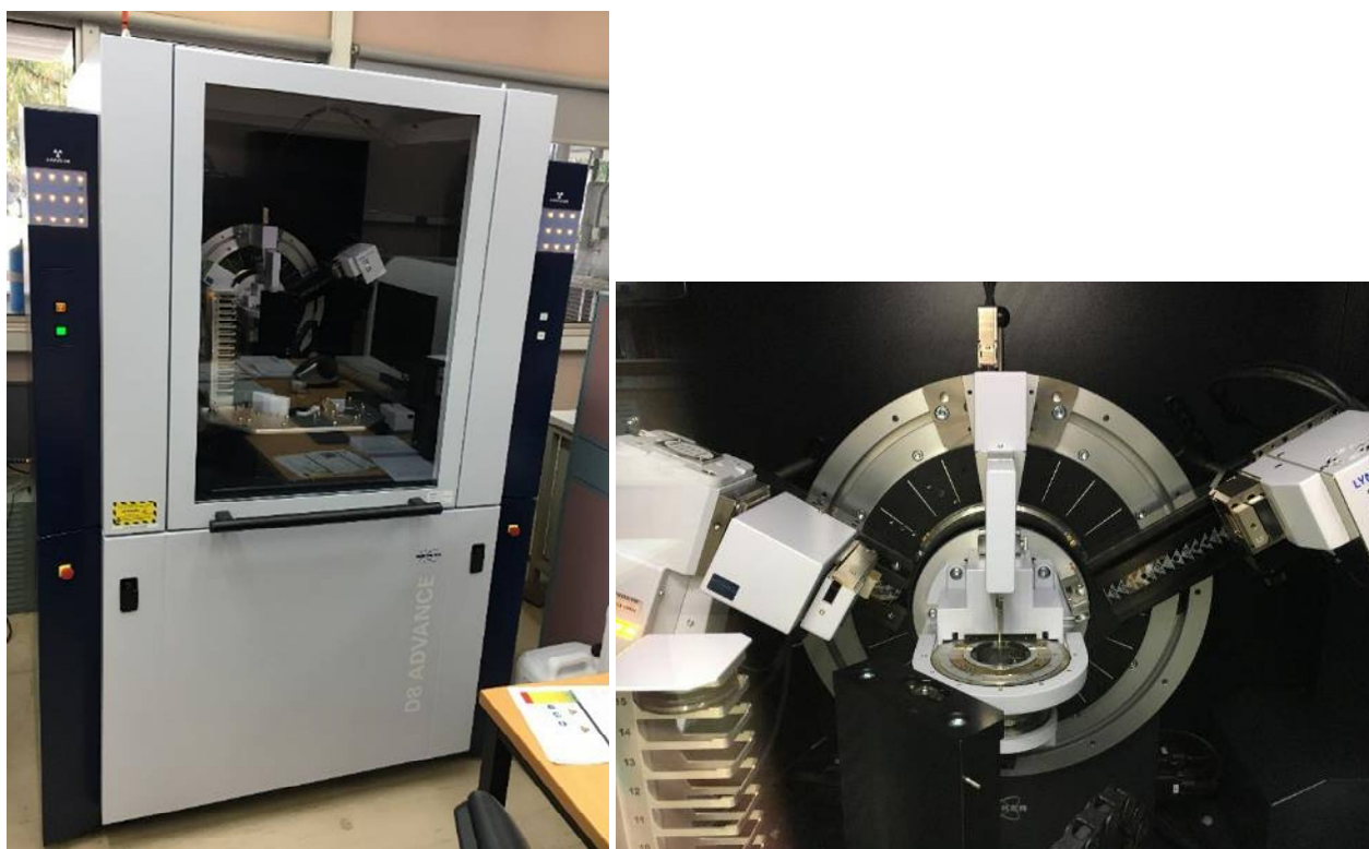
Figure 26 CSIRO's XRD instrument used for ACP analysis (photo by CSIRO)
