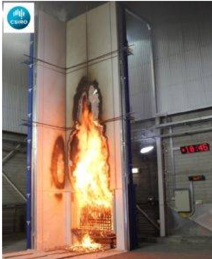
Figure 70. AS5113 thermocouple locations (left), CSIRO AS5113/BS8414 test rig (right)
