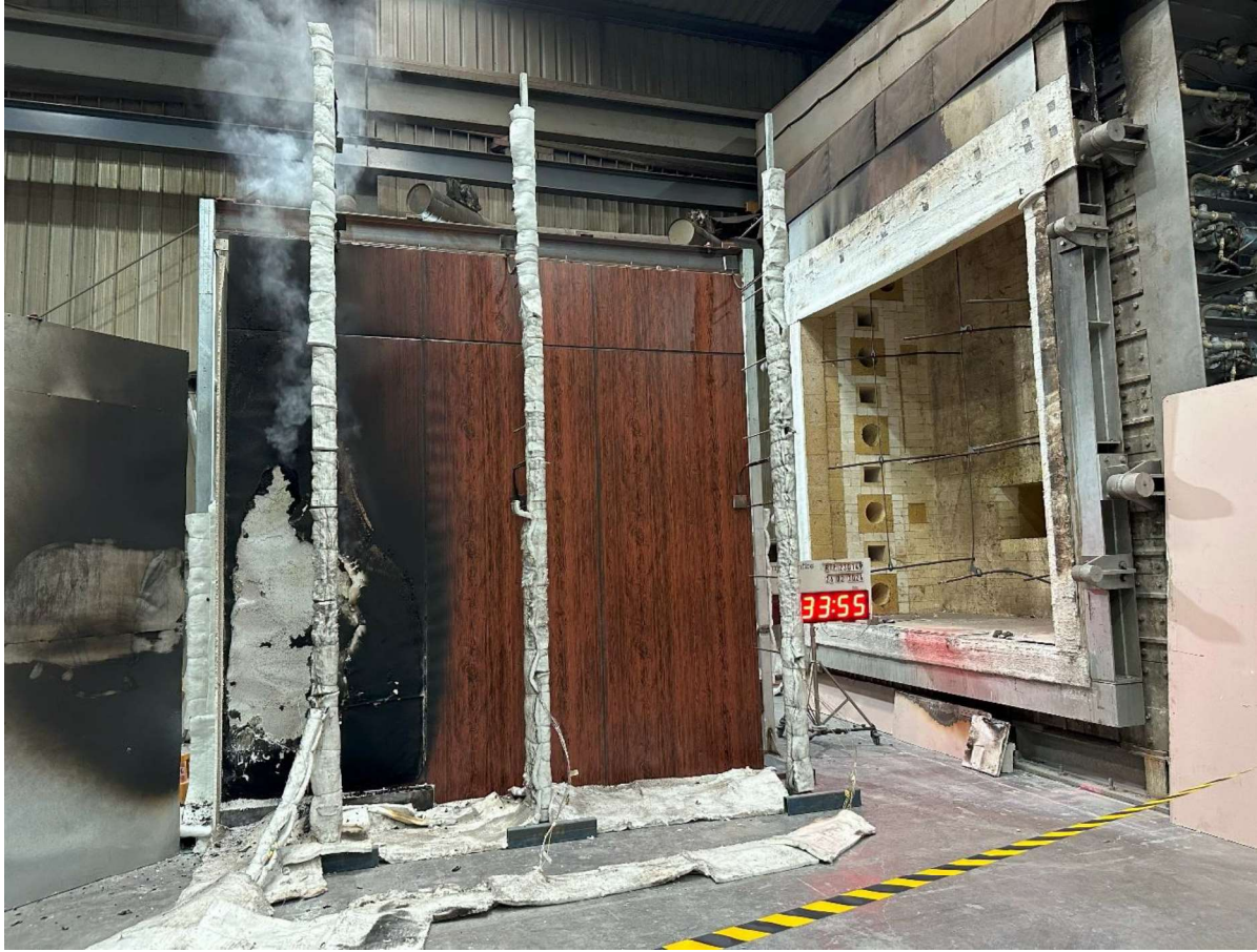
Figure 26 The specimen 33 minutes 55 seconds into the test (3 minutes 55 seconds after burner off).
