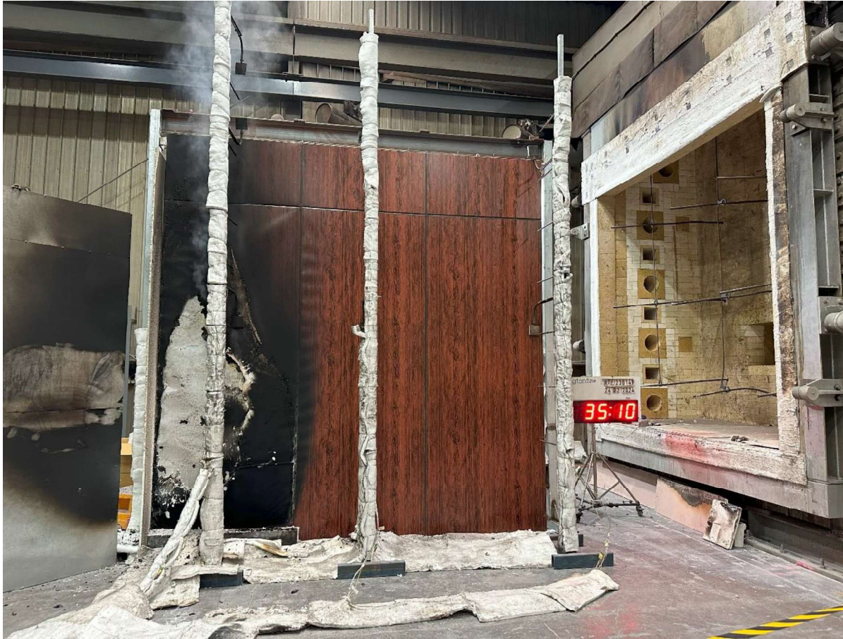
Figure 27 The specimen 35 minutes and 10 seconds into the test (5 minutes and 10 second after burner off).
