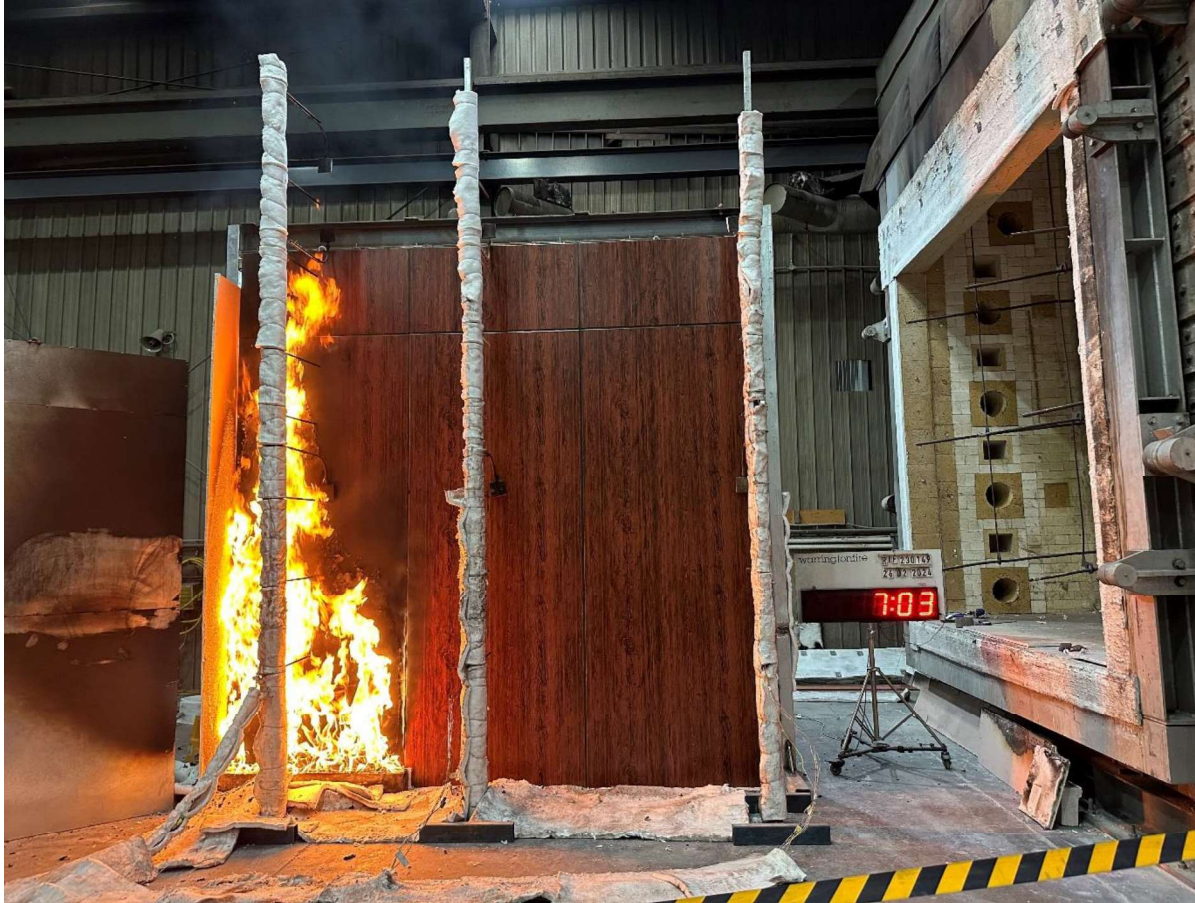
Figure 18 The specimen 7 minutes 3 seconds into the test (burner output at 300 kW)
