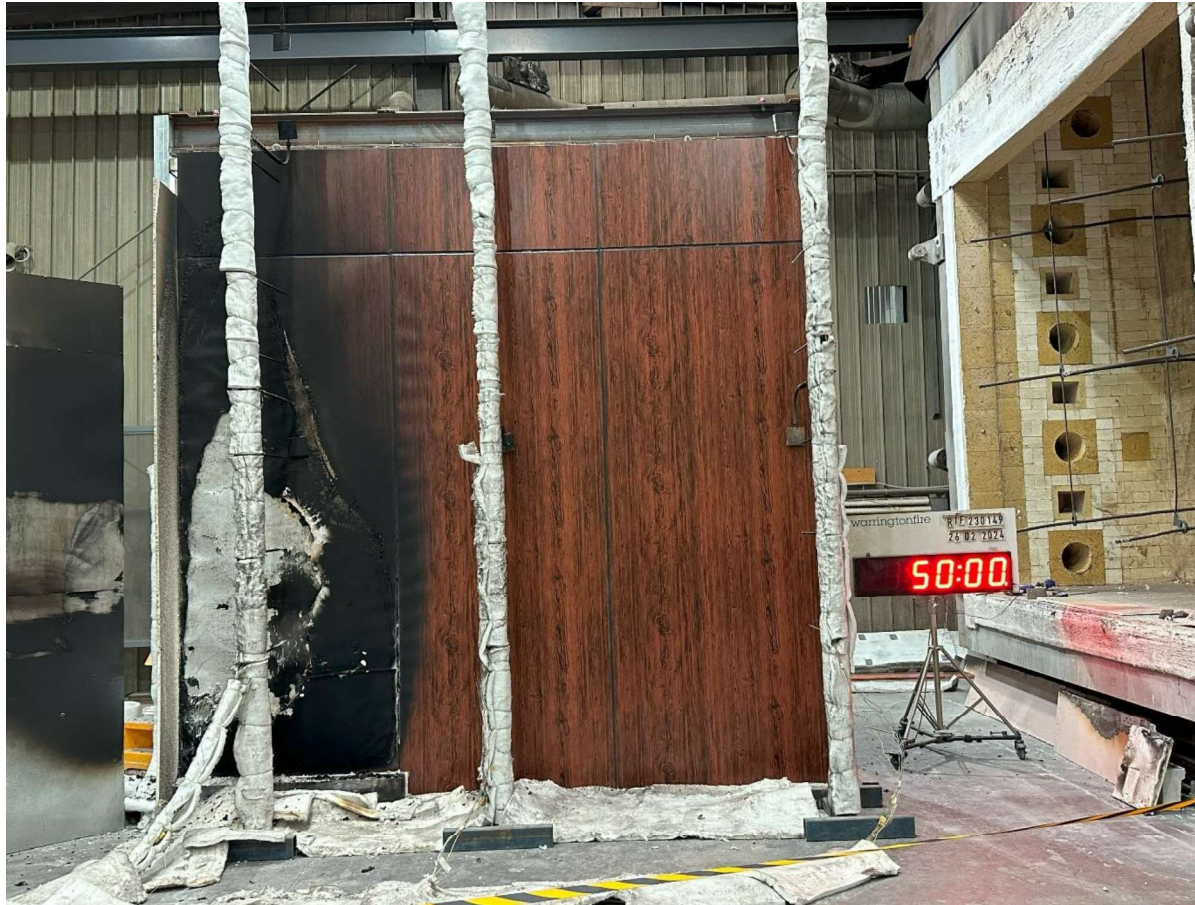
Figure 30 The specimen 50 minutes into the test (20 minutes after burner off).
