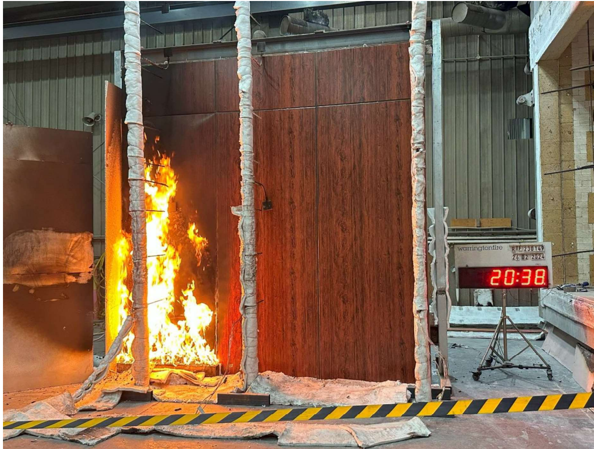
Figure 21 The specimen 20 minutes 38 seconds into the test (burner output at 300 kW).
