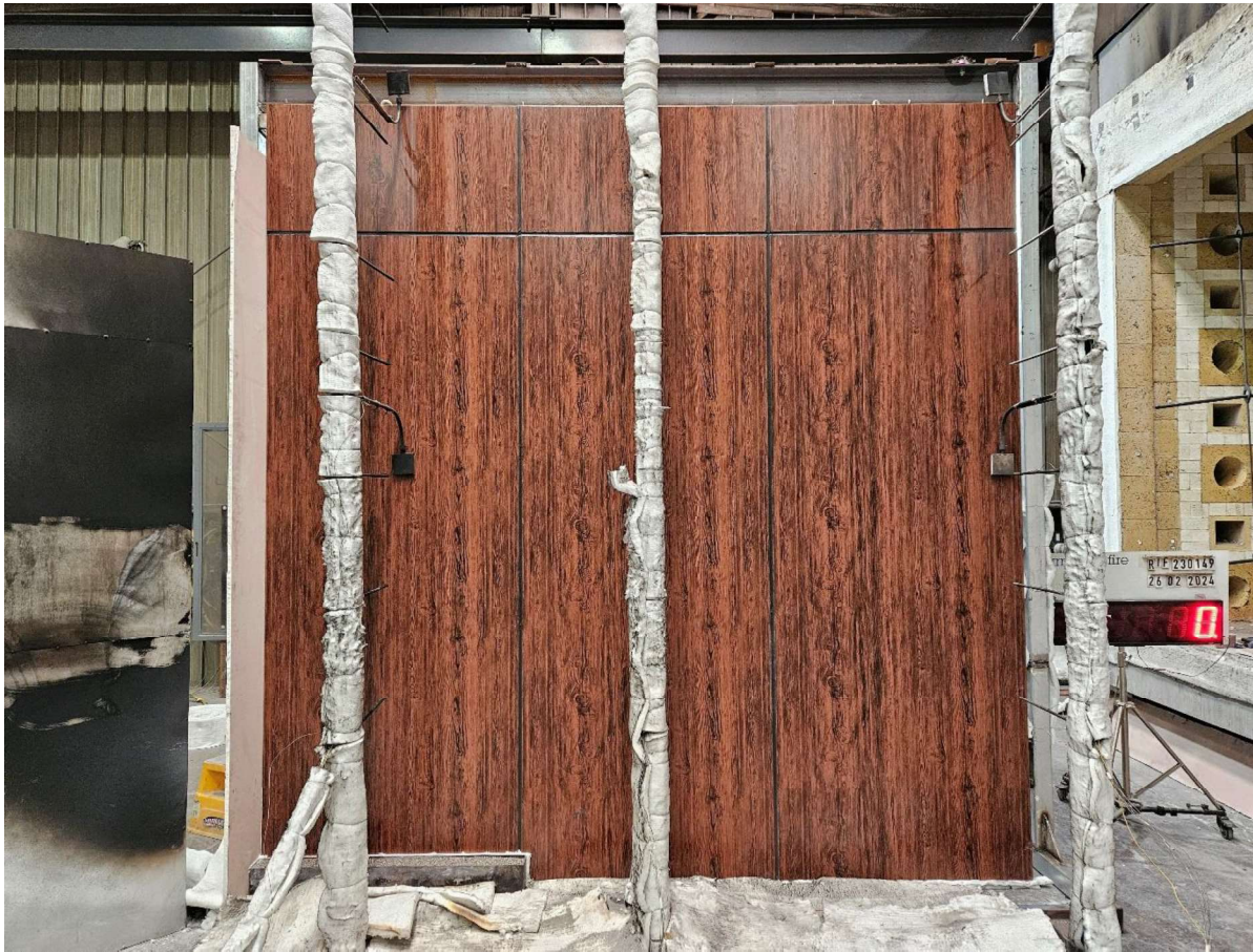
Figure 14 The specimen before the reaction to fire test - exposed side.
