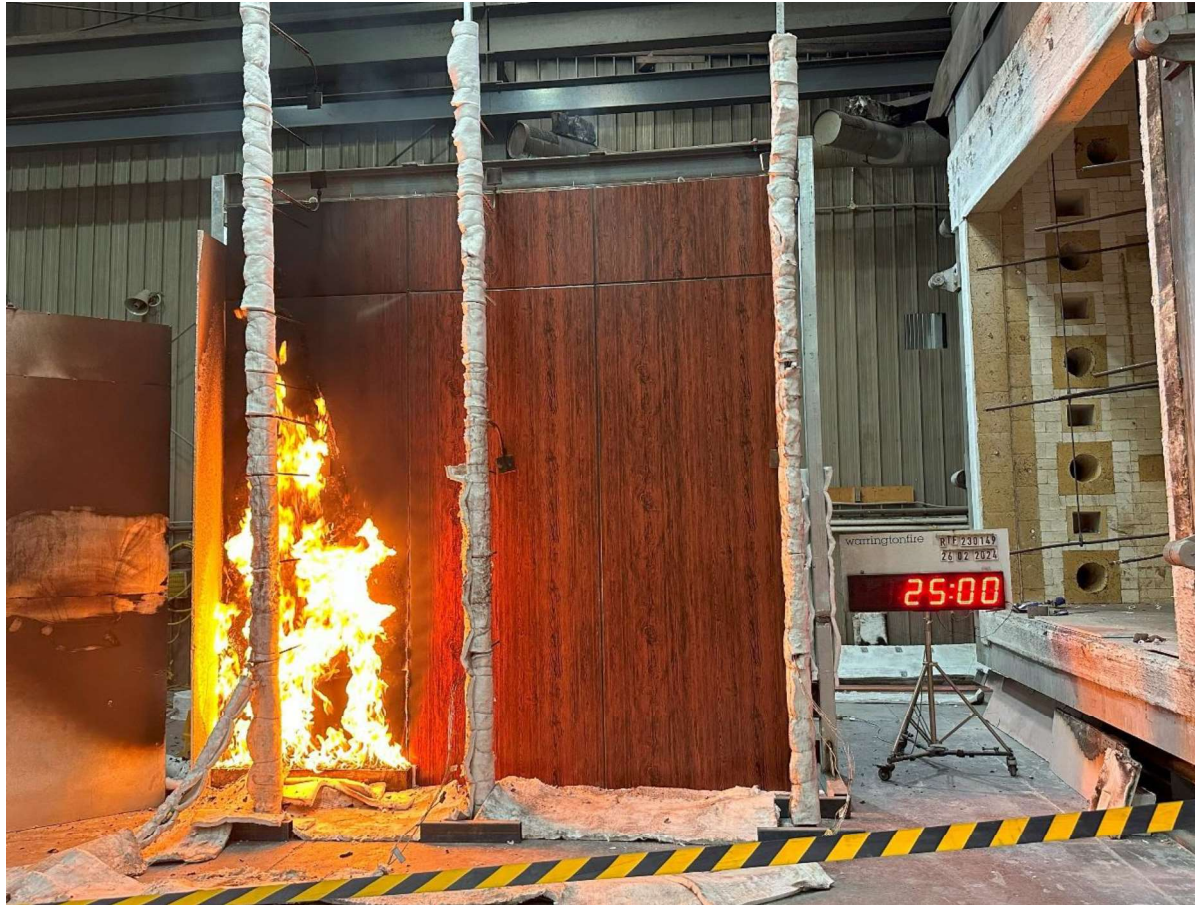
Figure 22 The specimen 25 minutes into the test (burner output at 300 kW).
