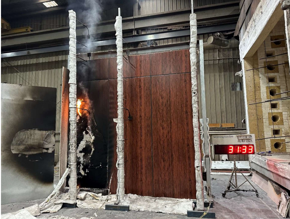
Figure 25 The specimen 31 minutes 33 seconds into the test (1 minute and 33 seconds after burner off).
