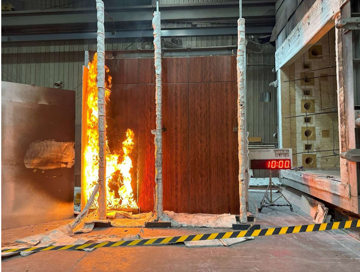
Figure 19 The specimen 10 minutes into the test (burner output at 300 kW)
