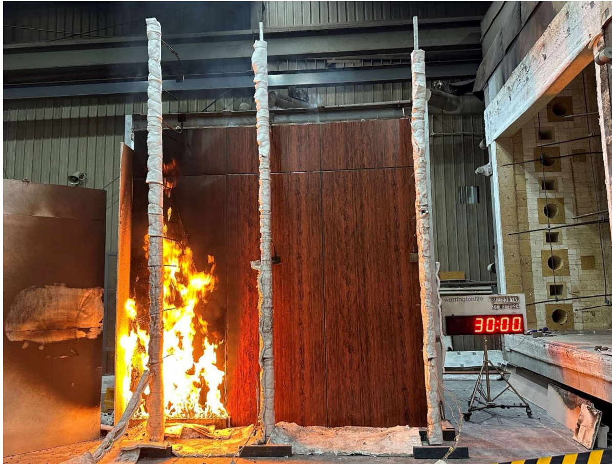
Figure 23 The specimen 30 minutes into the test (burner off).
