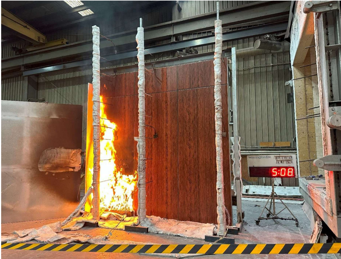
Figure 17 The specimen 5 minutes 8 seconds into the test (burner output at 300 kW)
