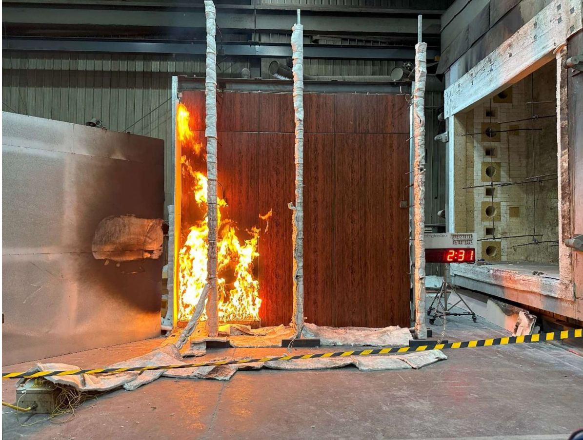
Figure 16 The specimen 2 minutes 31 seconds into the test (burner output at 300 kW)
