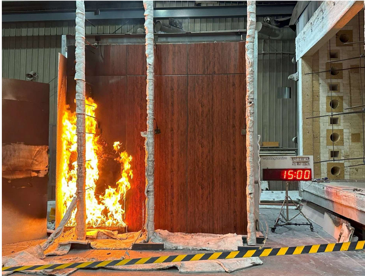
Figure 20 The specimen 15 minutes into the test (burner output at 300 kW).
