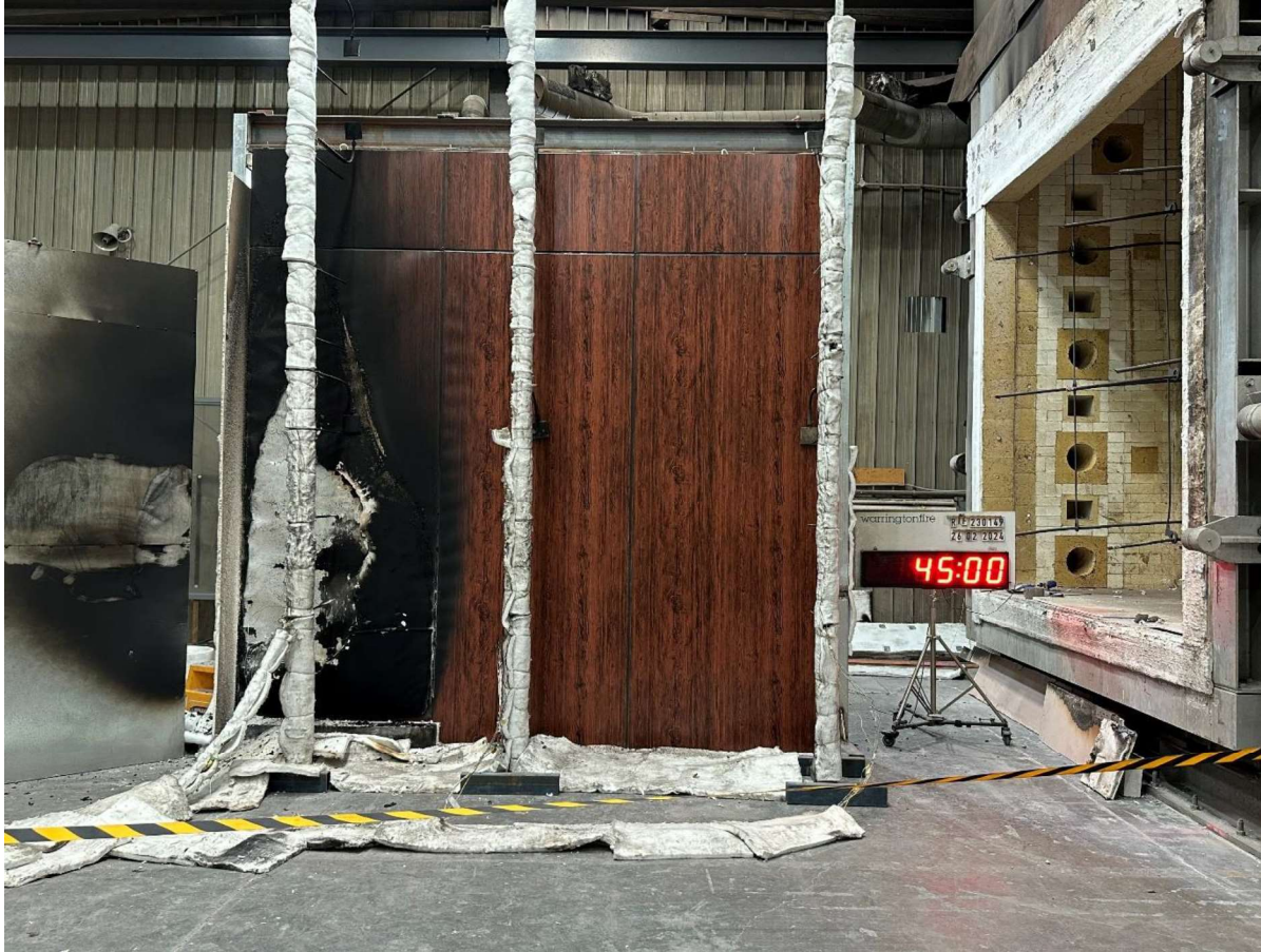
Figure 29 The specimen 45 minutes into the test (15 minutes after burner off).
