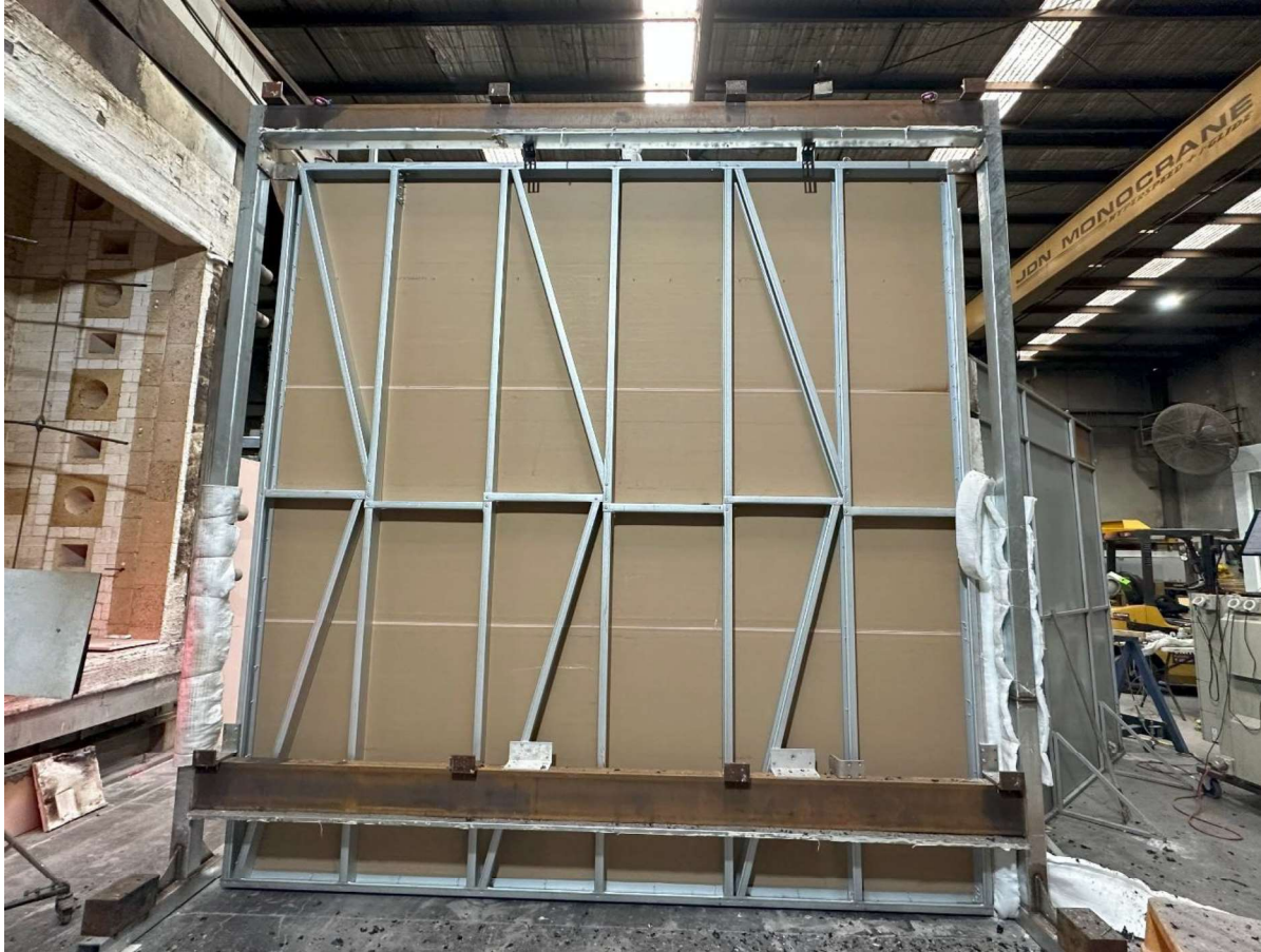
Figure 32 The unexposed side of the specimen at the end of test.
