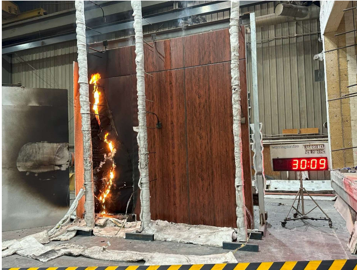
Figure 24 The specimen 30 minutes 9 seconds into the test (9 seconds after burner off).
