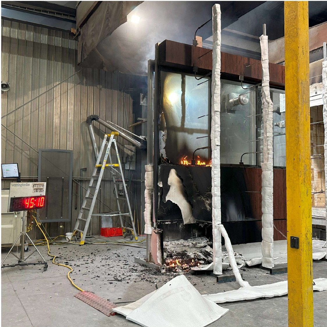
Figure 36 The specimen 45 minutes 10 seconds into the test (burner off)
