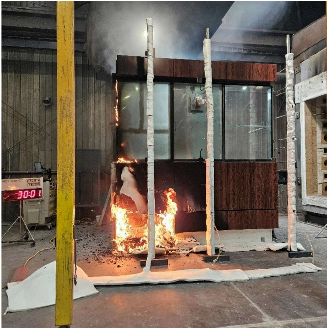
Figure 35 The specimen 30 minutes 01 second into the test (burner off)
