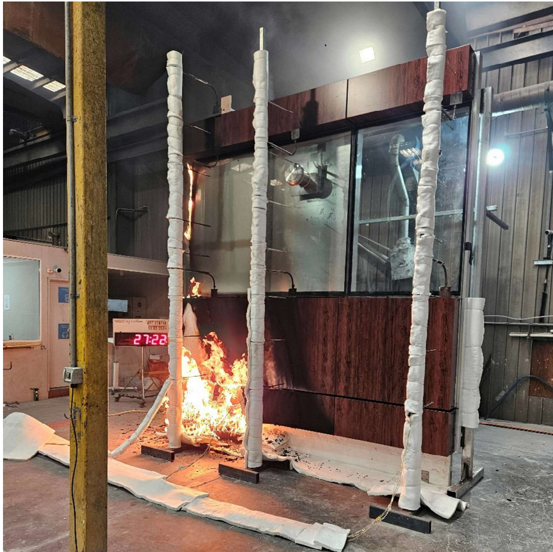
Figure 34 The specimen 27 minutes 22 seconds into the test (burner output at 300 kW)
