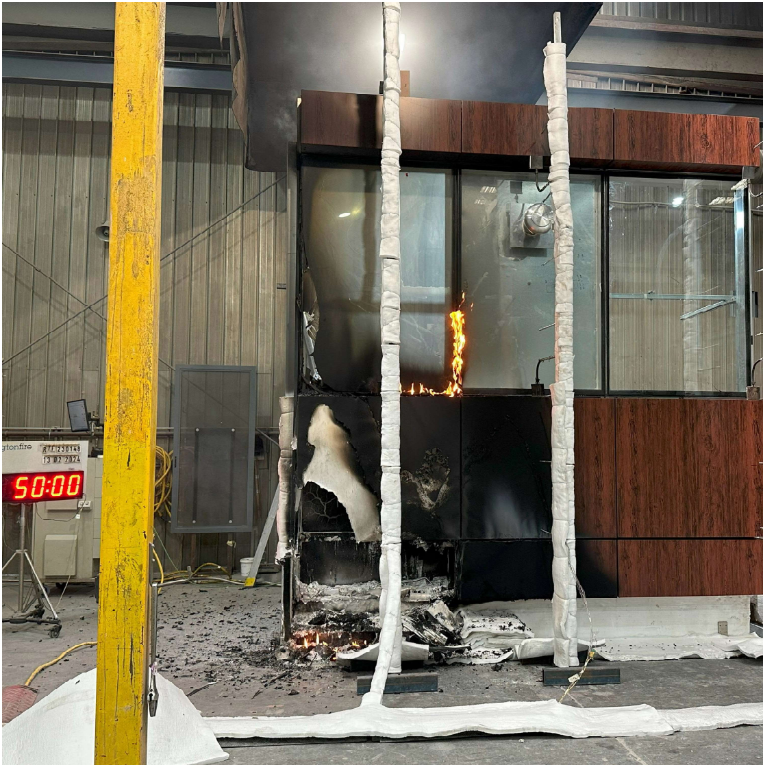
Figure 37 The specimen 50 minutes into the test (burner off)
