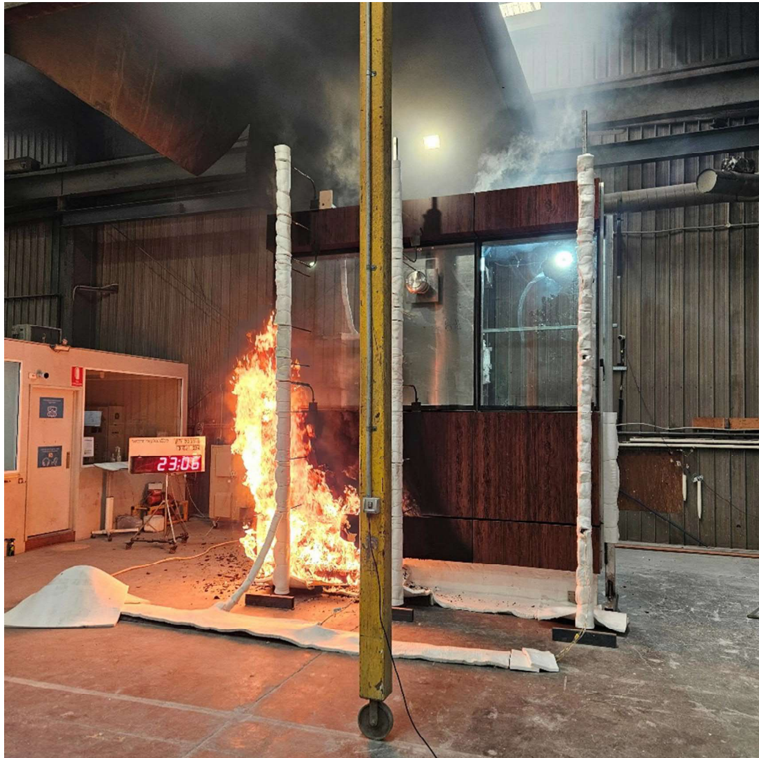
Figure 33 The specimen 23 minutes 6 seconds into the test (burner output at 300 kW)
