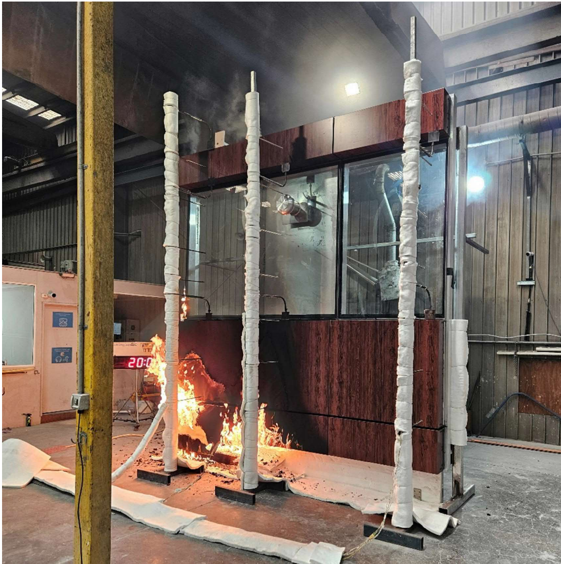
Figure 32 The specimen 20 minutes into the test (burner output at 300 kW)
