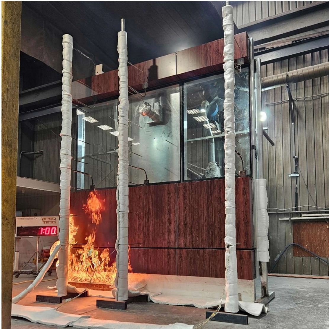
Figure 29 The specimen 1 minute into the test (burner output at 300 kW)
