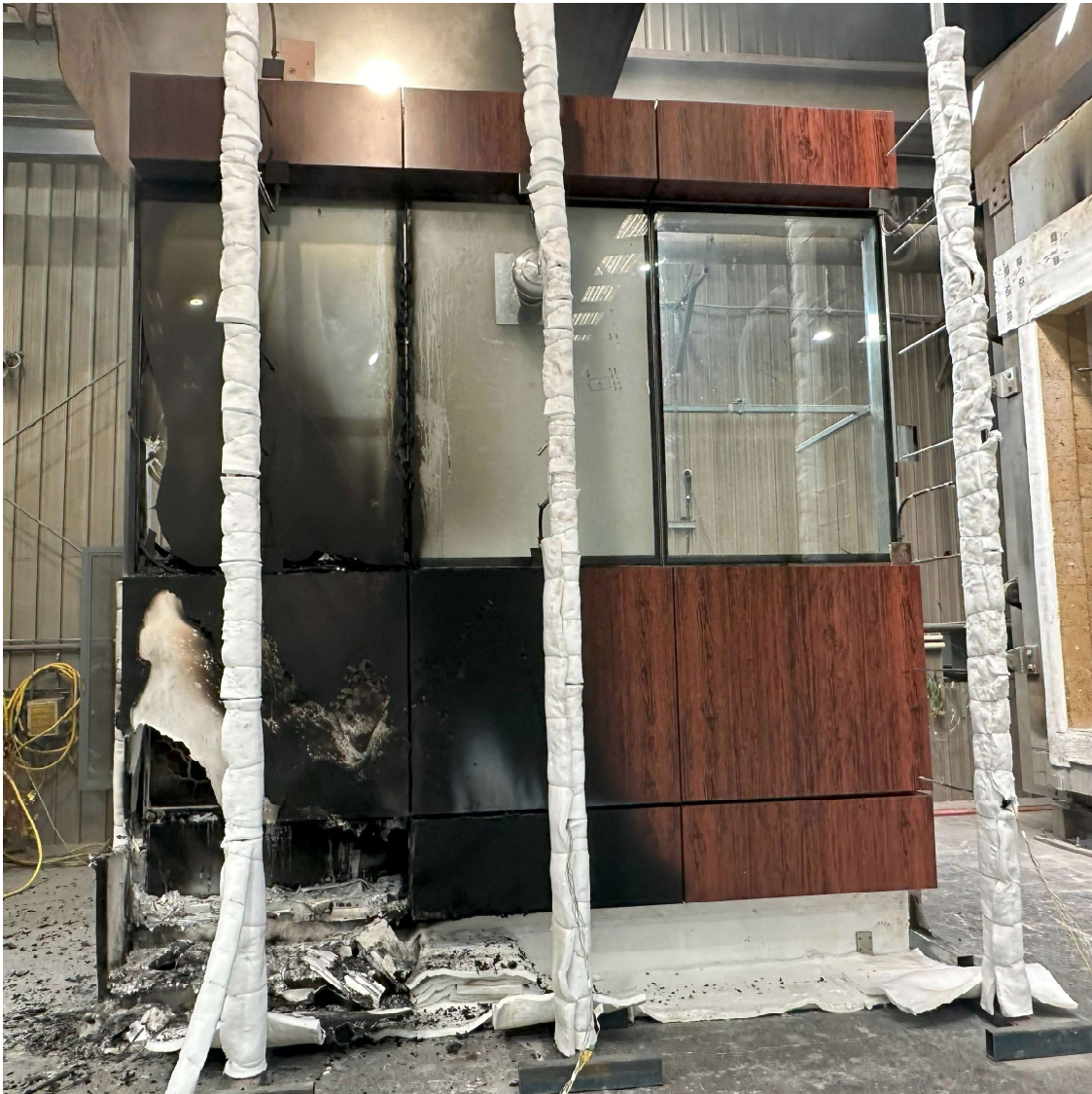
Figure 38 The specimen at end of test – exposed side
