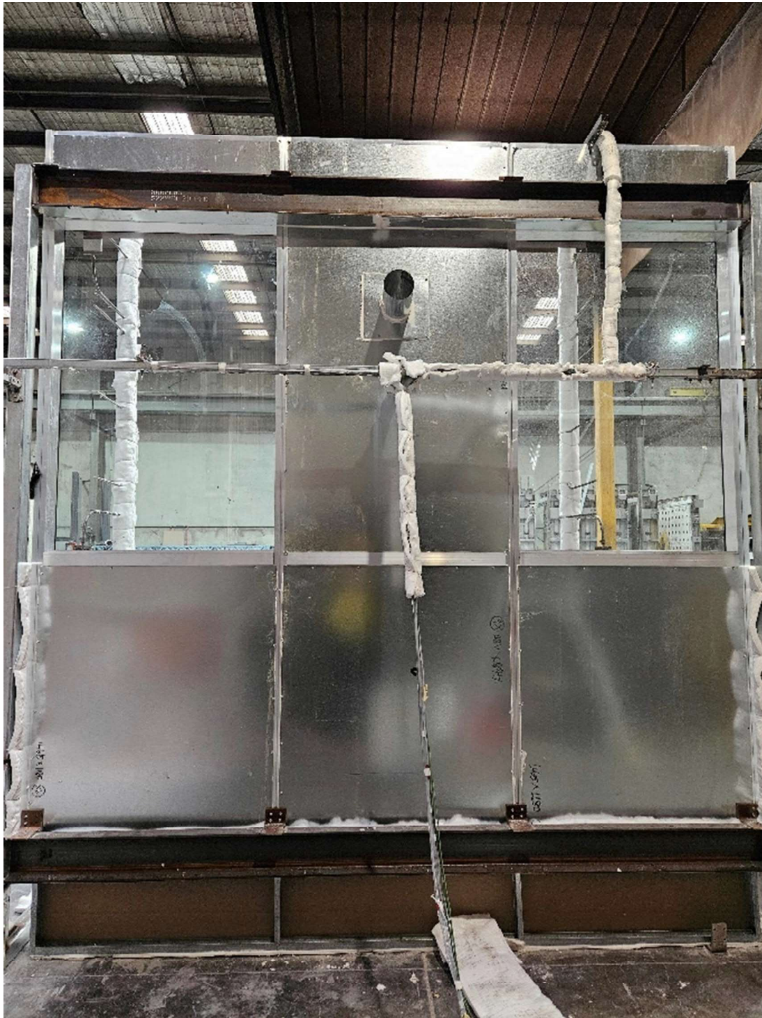
Figure 28 The specimen (unexposed side) before the reaction to fire test
