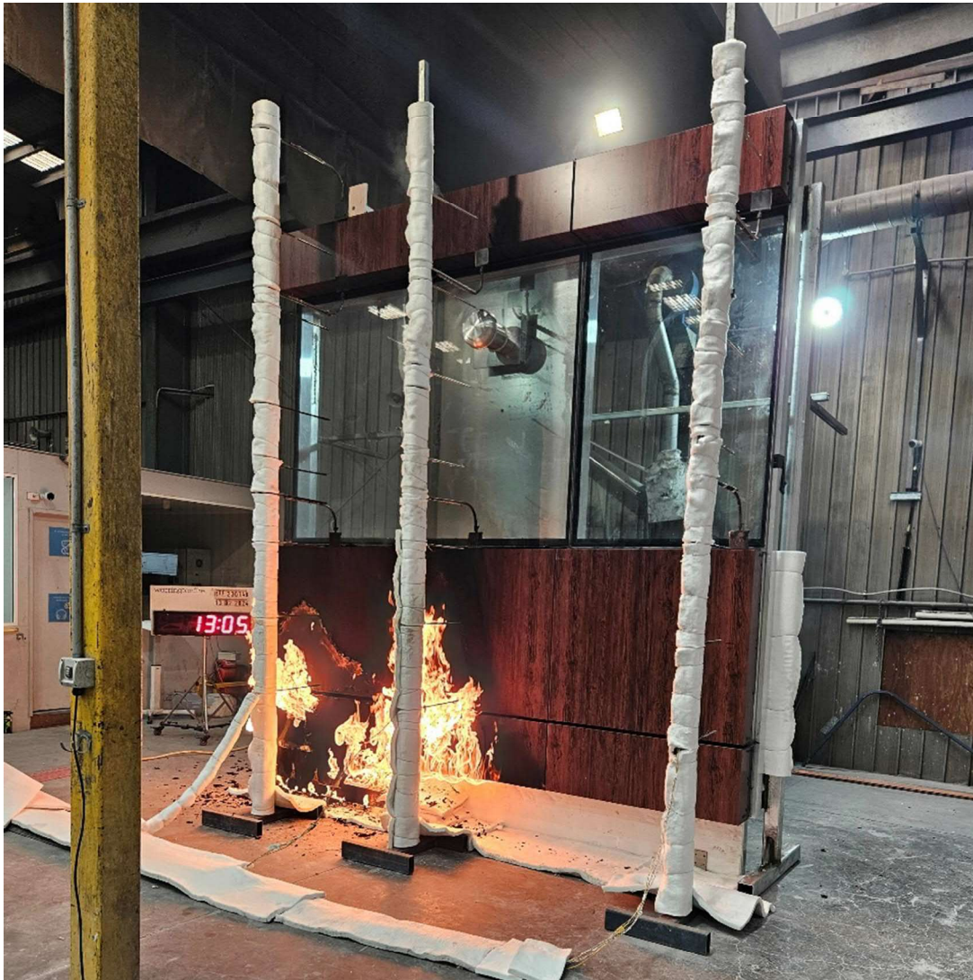
Figure 31 The specimen 13 minutes 5 seconds into the test (burner output at 300 kW)
