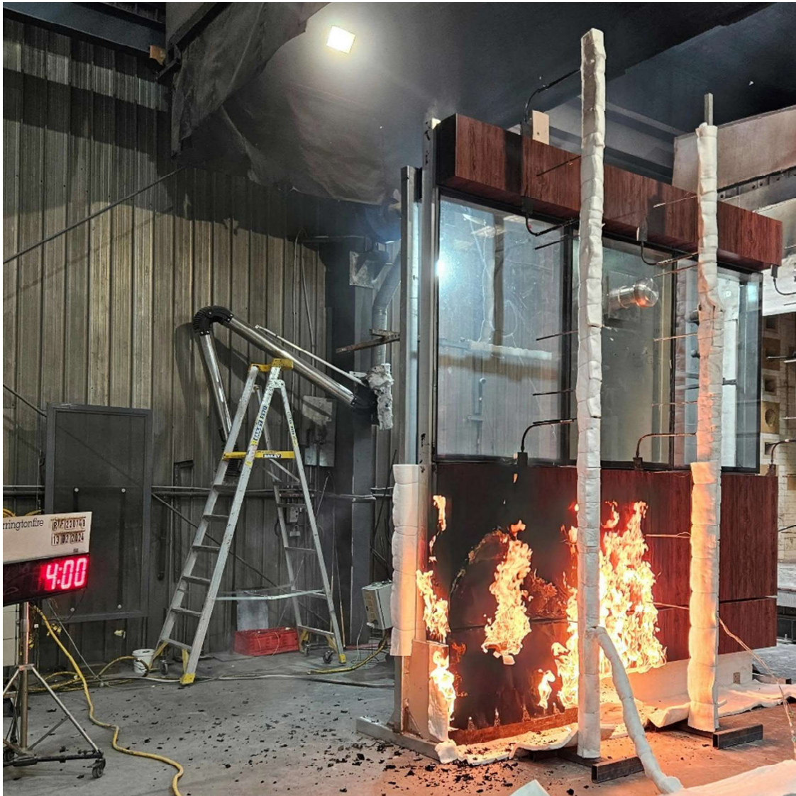
Figure 30 The specimen 4 minutes into the test (burner output at 300 kW)
