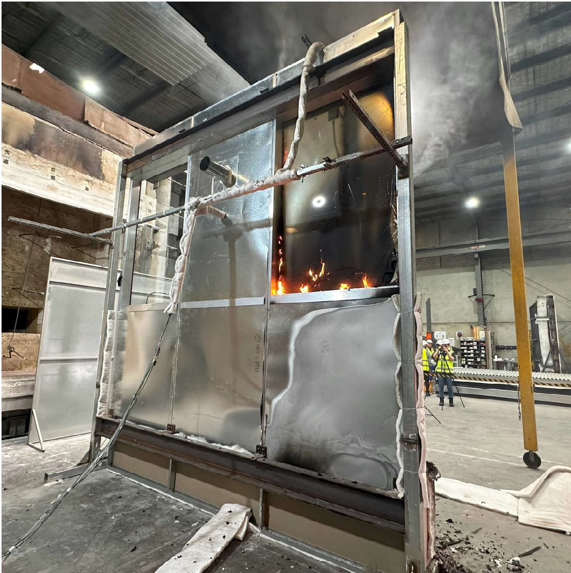
Figure 39 The specimen at end of test – unexposed side
