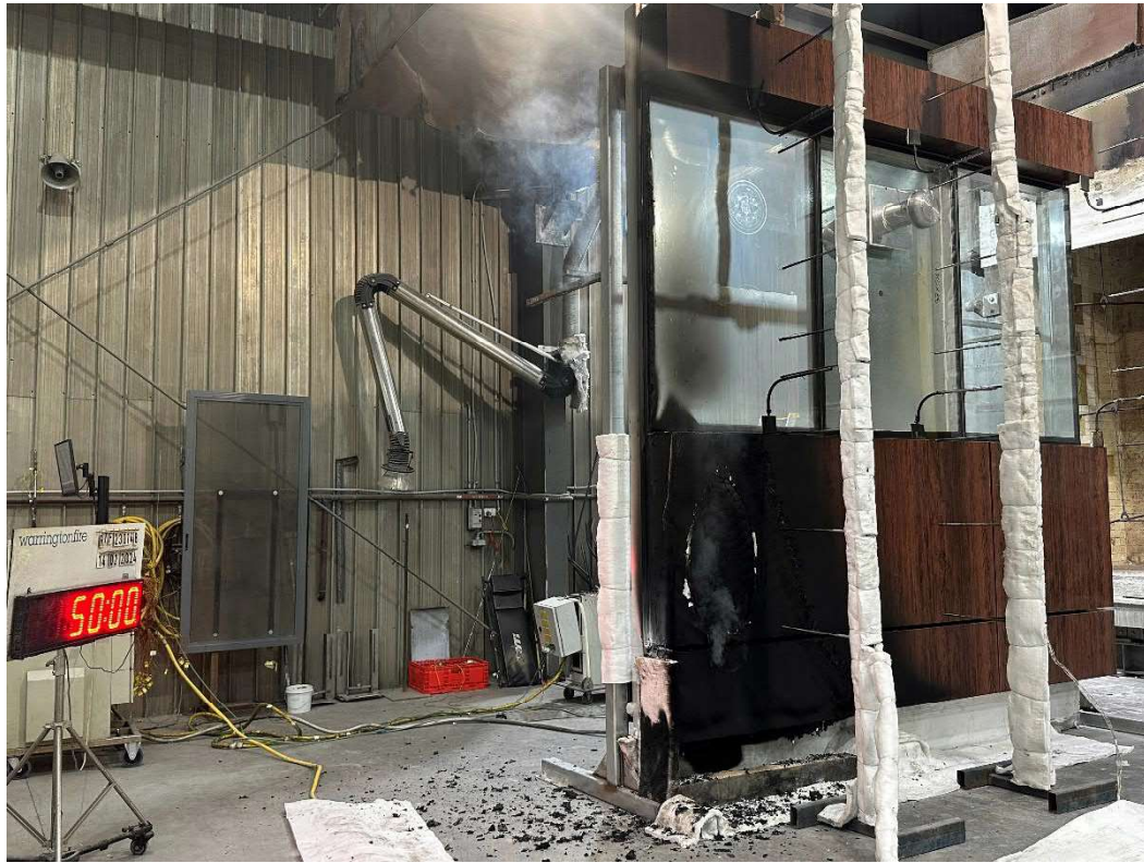
Figure 37 The specimen 50 minutes into the test (burner off)
