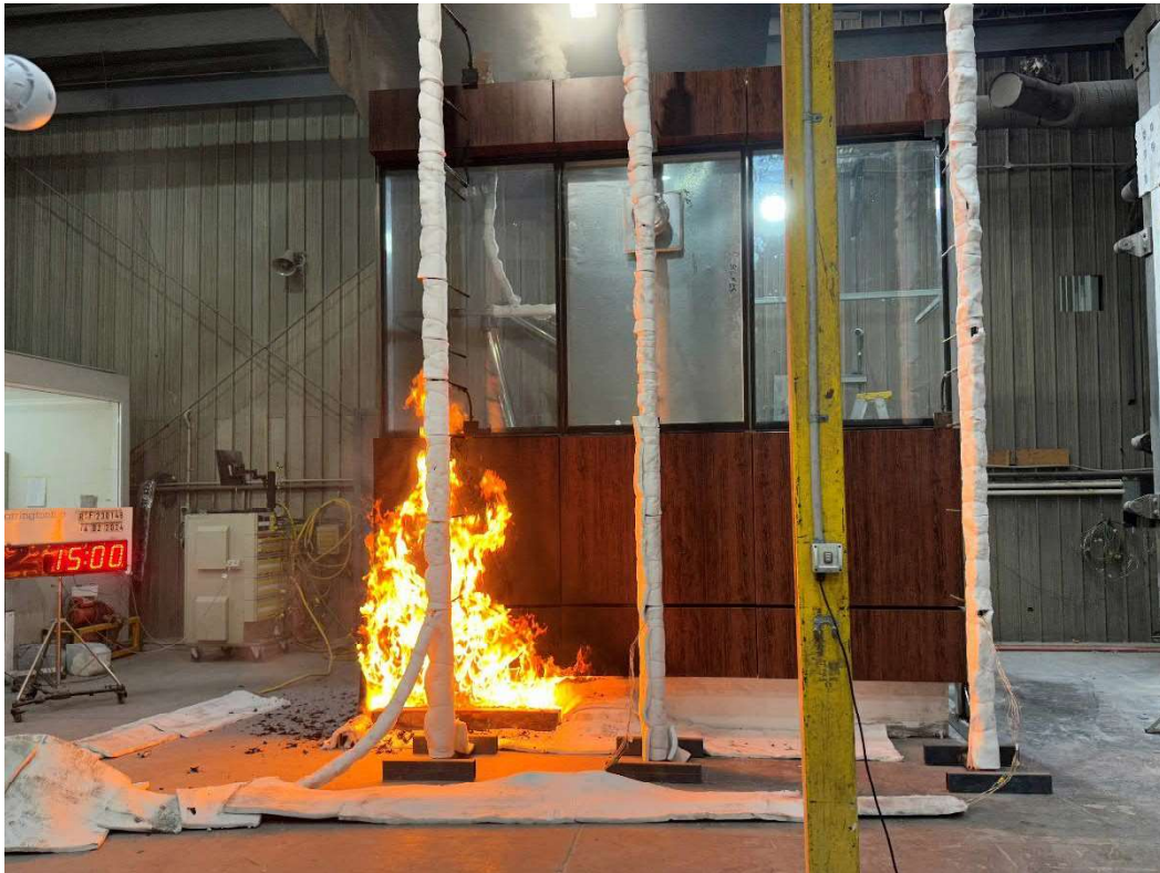
Figure 33 The specimen 15 minutes into the test (burner output at 300 kW)
