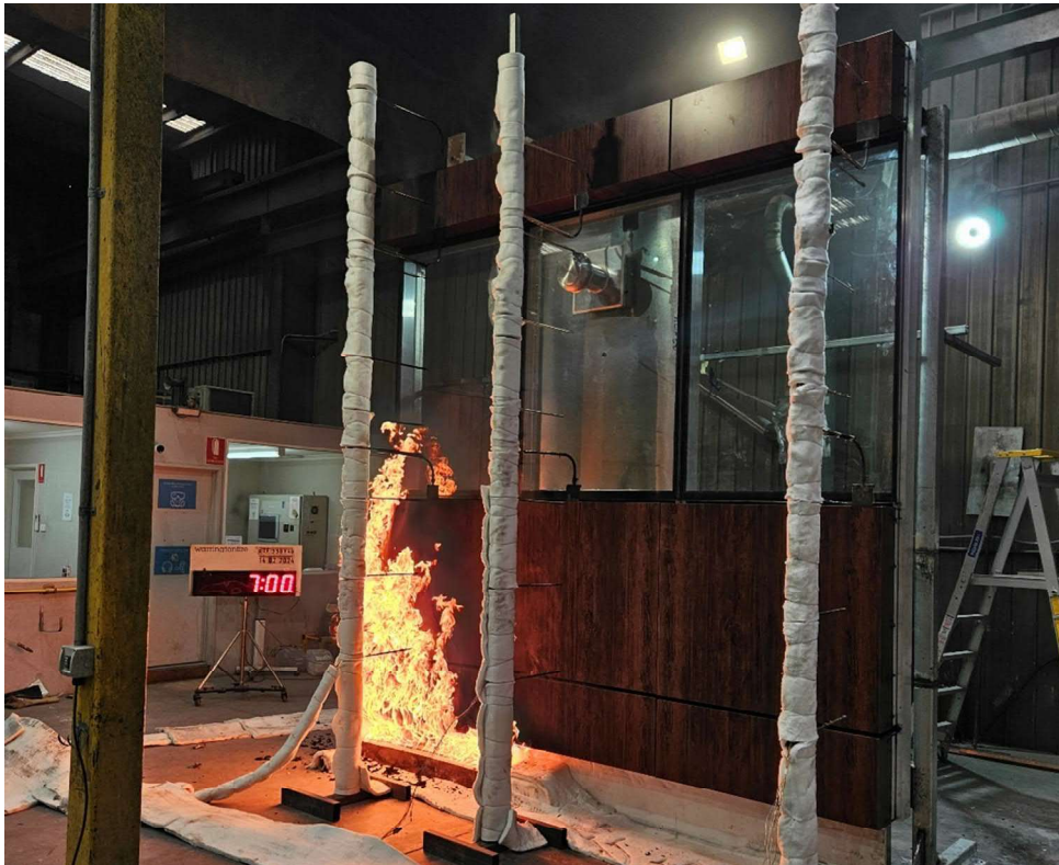
Figure 31 The specimen 7 minutes into the test (burner output at 300 kW)
