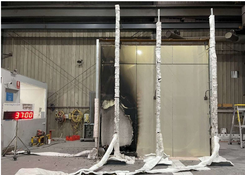
Figure 27 The specimen 37 minutes into the test (7 minutes after burner off)
