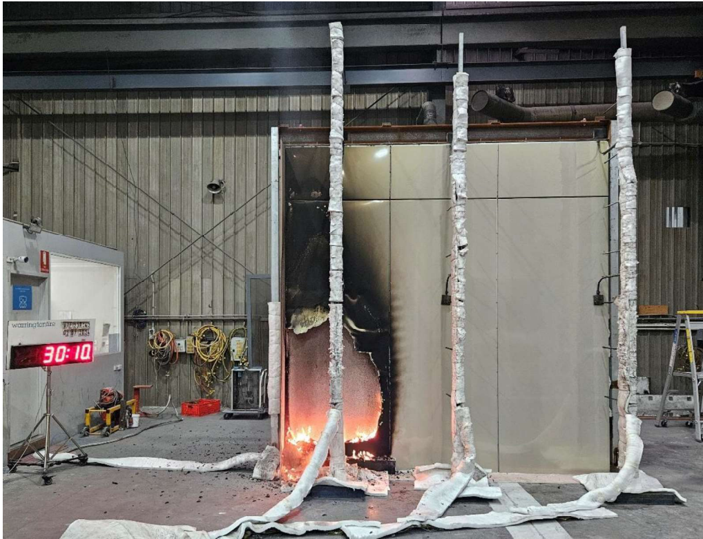
Figure 24 The specimen 30 minutes 10 seconds into the test (10 seconds after burner off)
