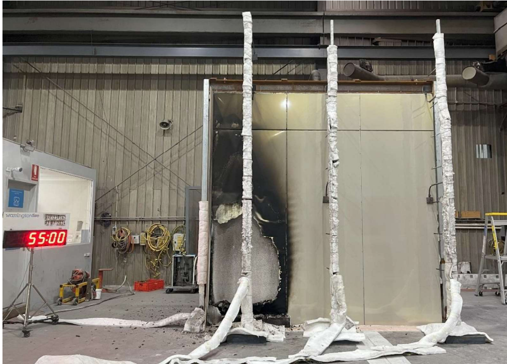
Figure 30 The specimen 55 minutes into the test (25 minutes after burner off)
