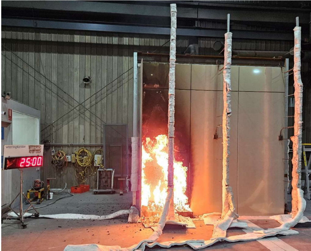
Figure 22 The specimen 25 minutes into the test (burner output at 300 kW)
