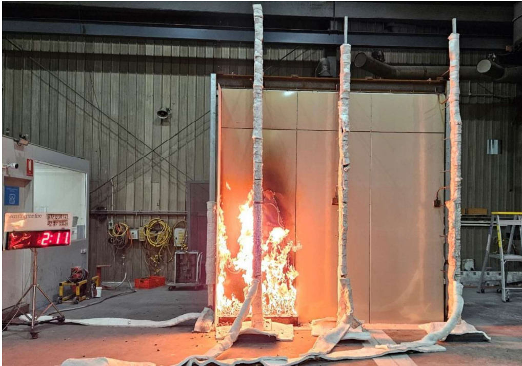
Figure 16 The specimen 2 minutes 11 seconds into the test (burner output at 300 kW)
