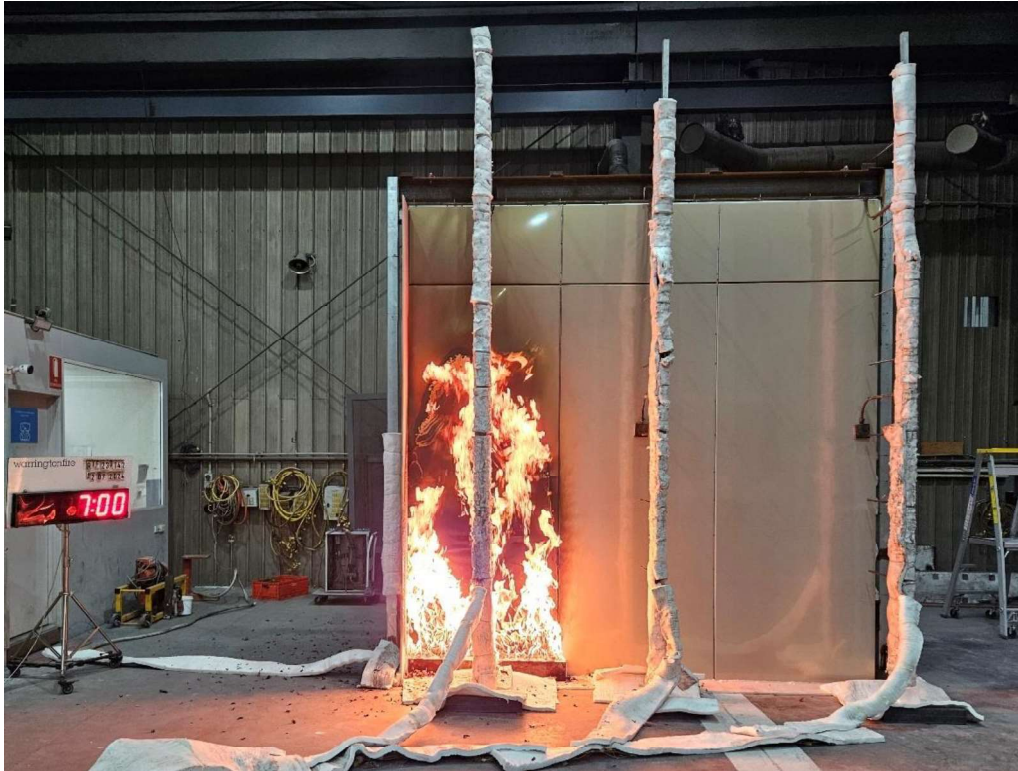
Figure 18 The specimen 7 minutes into the test (burner output at 300 kW)
