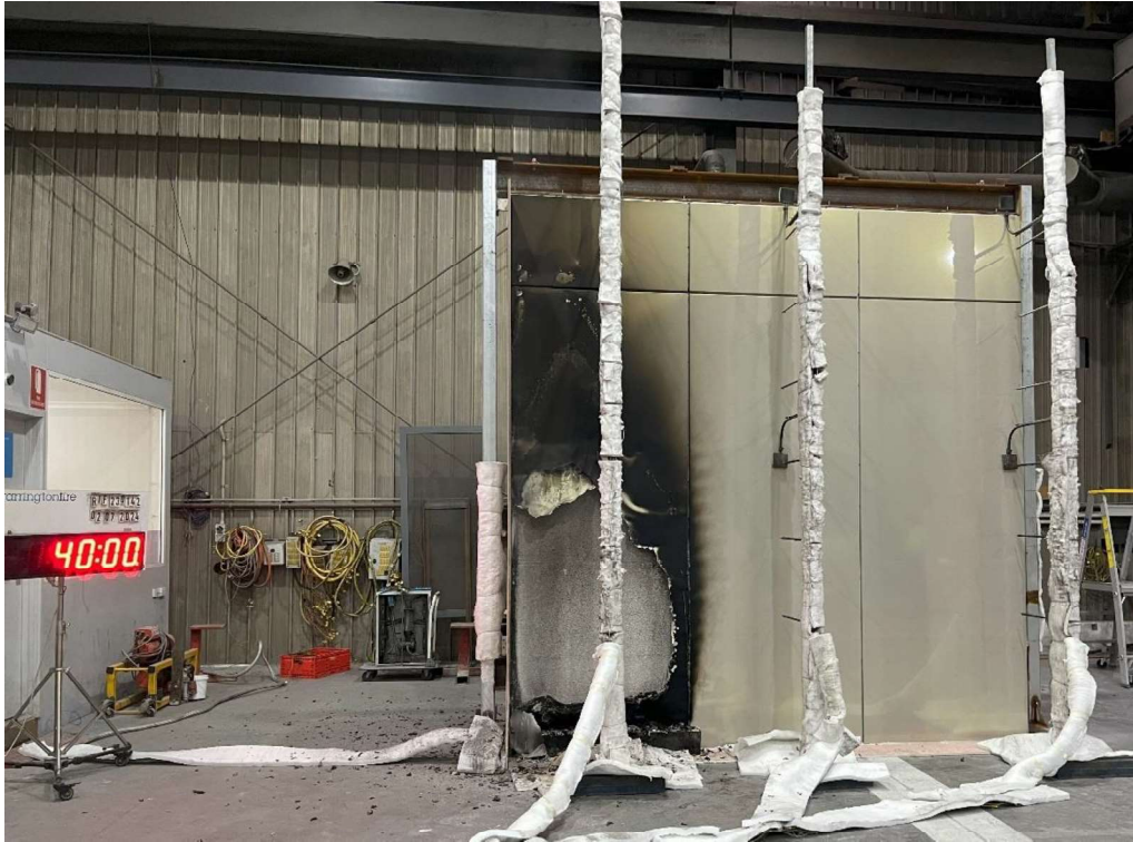
Figure 28 The specimen 40 minutes into the test (10 minutes after burner off)
