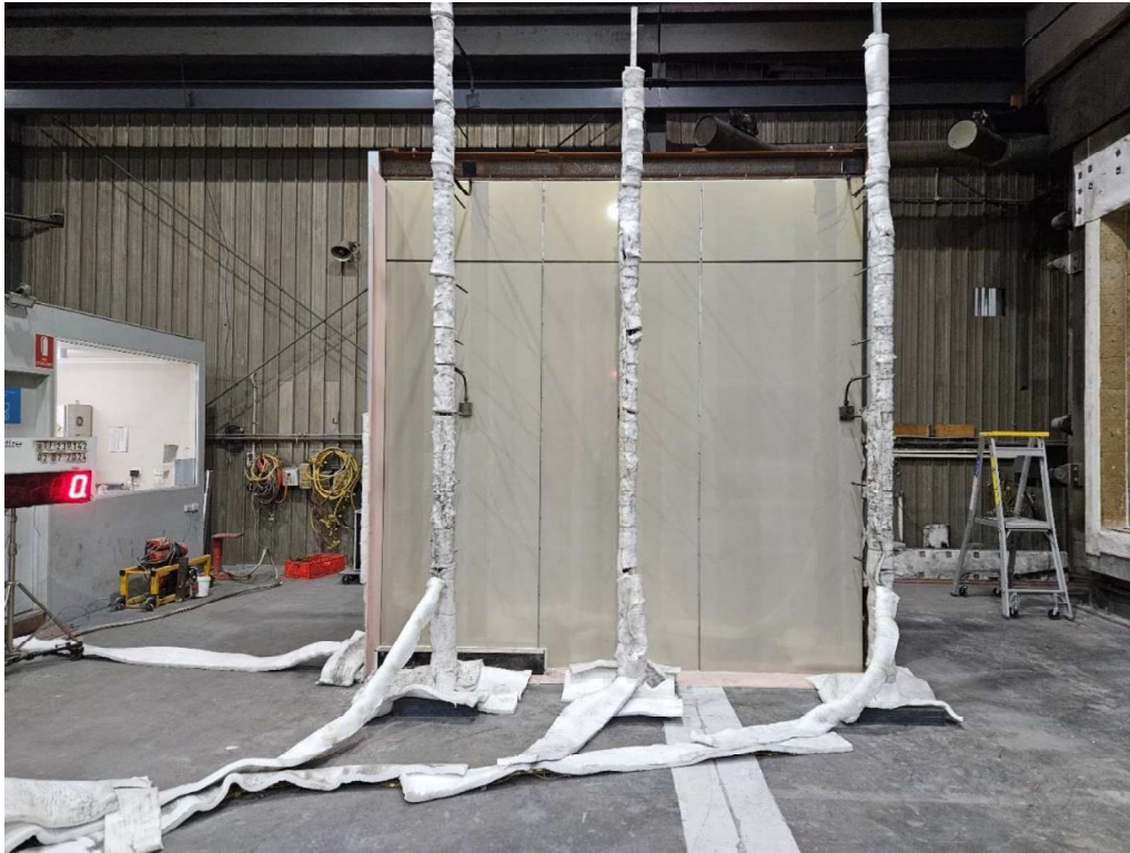
Figure 14 The specimen before the reaction to fire test - exposed side
