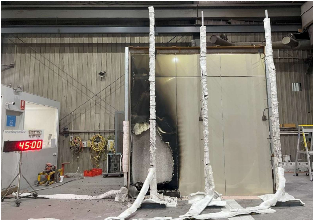
Figure 29 The specimen 45 minutes into the test (15 minutes after burner off)
