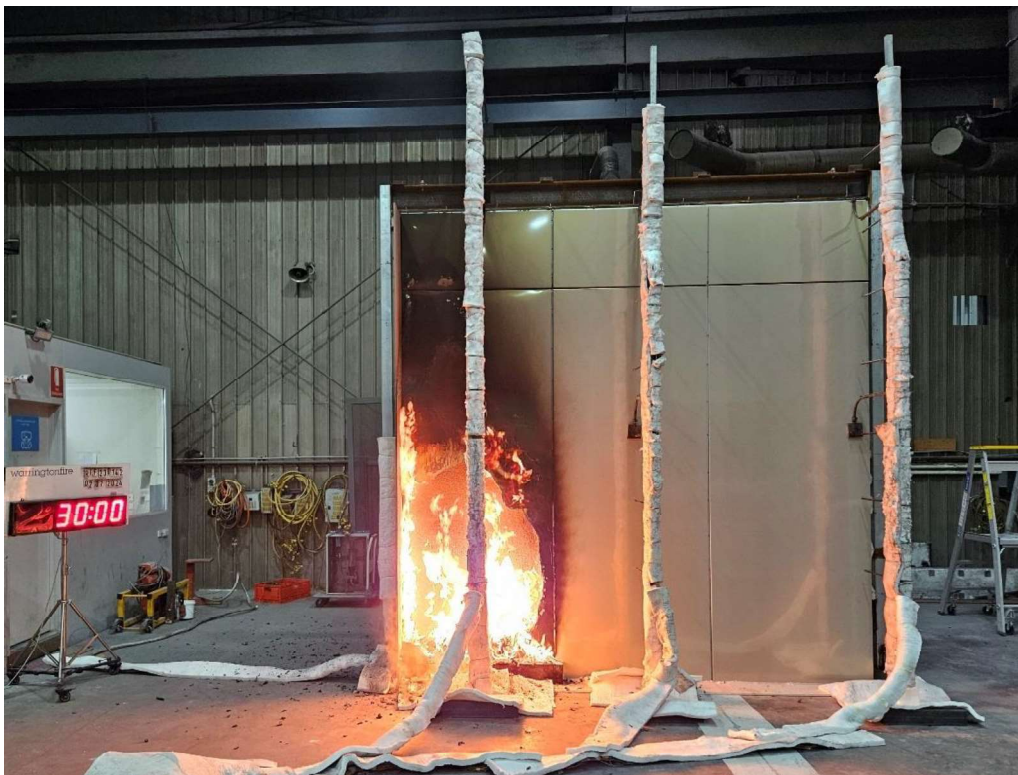
Figure 23 The specimen 30 minutes into the test (burner output at 300 kw)
