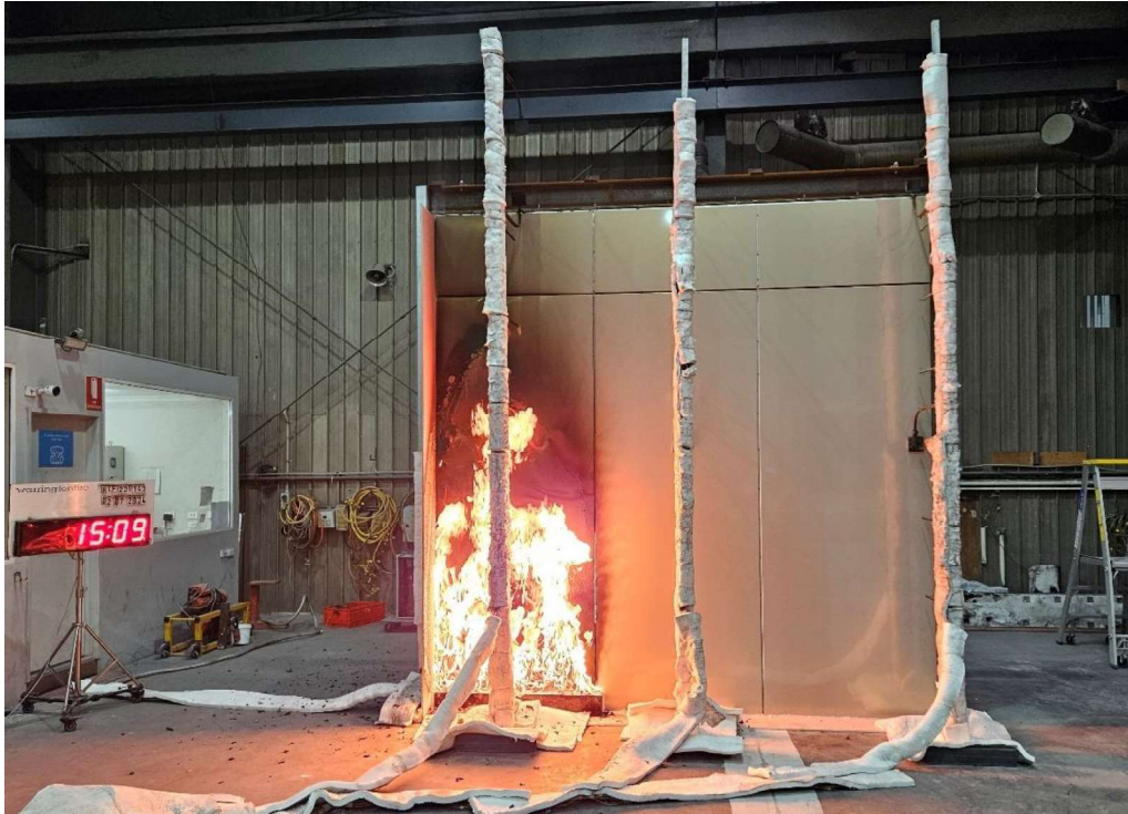
Figure 20 The specimen 15 minutes 9 seconds into the test (burner output at 300 kW)
