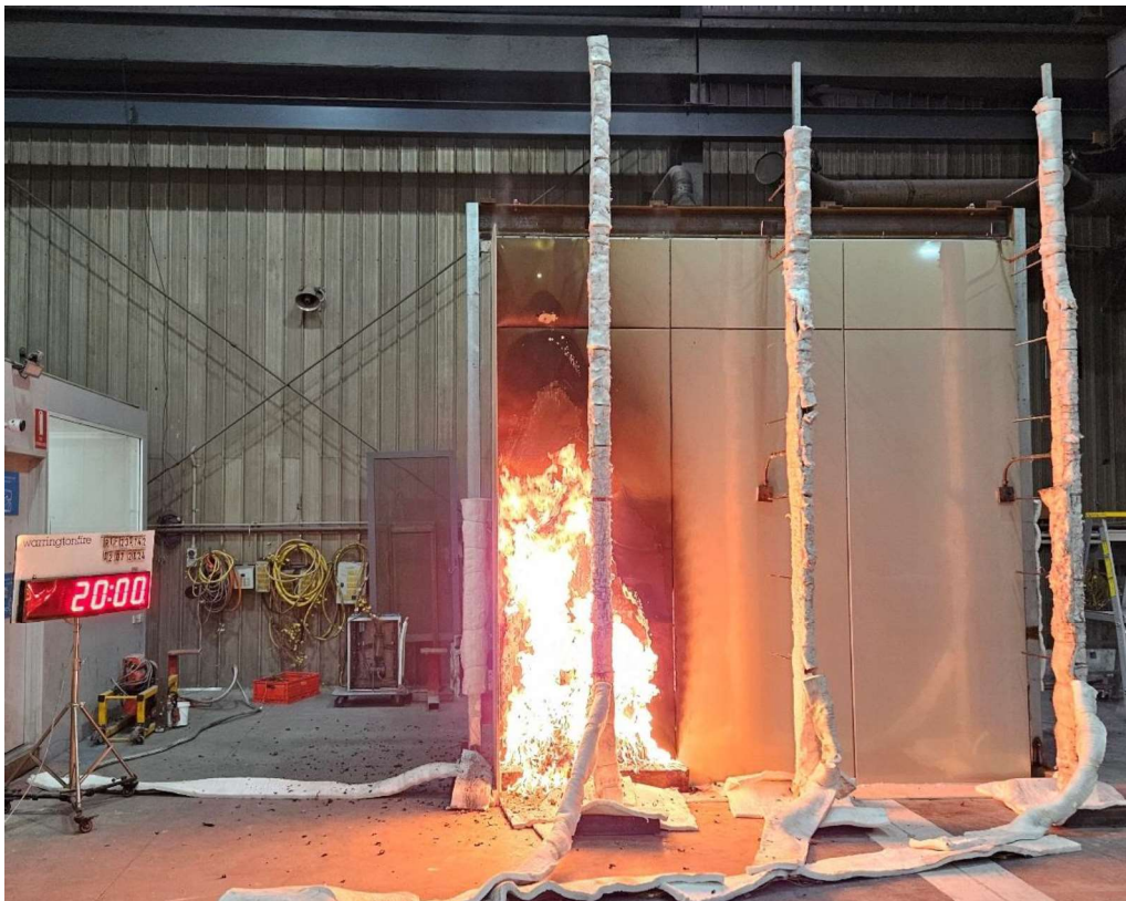
Figure 21 The specimen 20 minutes into the test (burner output at 300 kW)
