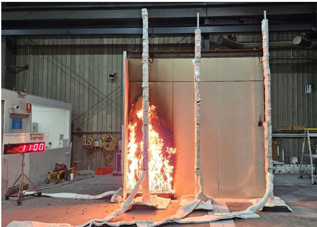
Figure 19 The specimen 11 minutes into the test (burner output at 300 kW)
