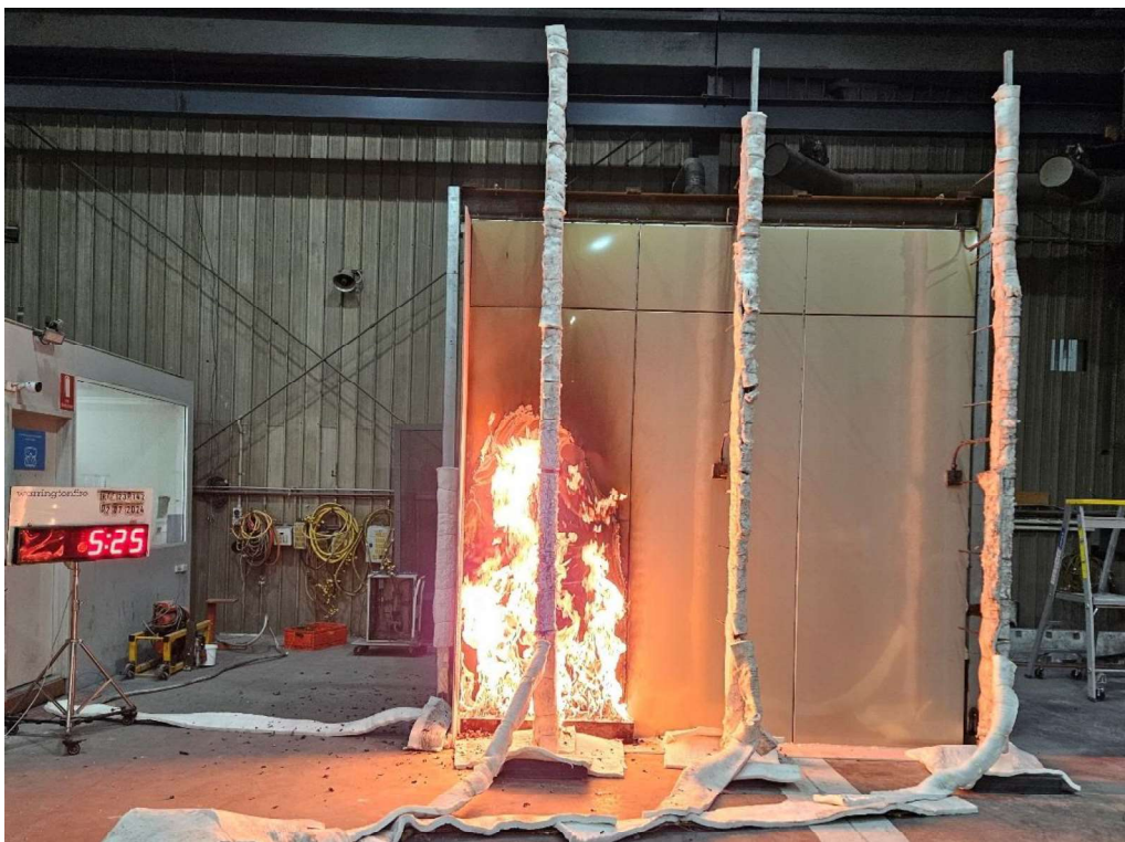
Figure 16 The specimen 2 minutes 11 seconds into the test (burner output at 300 kW)
