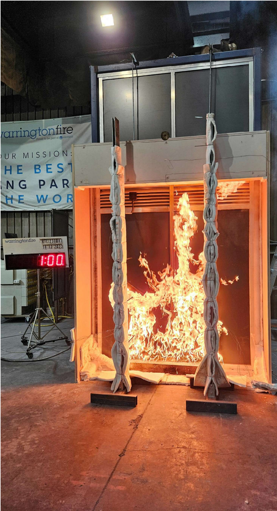
Figure 20 The specimen 1 minute into the test (burner output set to 300 kW for the duration of the test)
