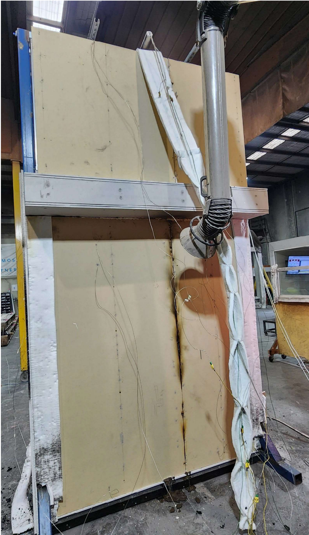
Figure 31 The specimen after the test – unexposed side.
