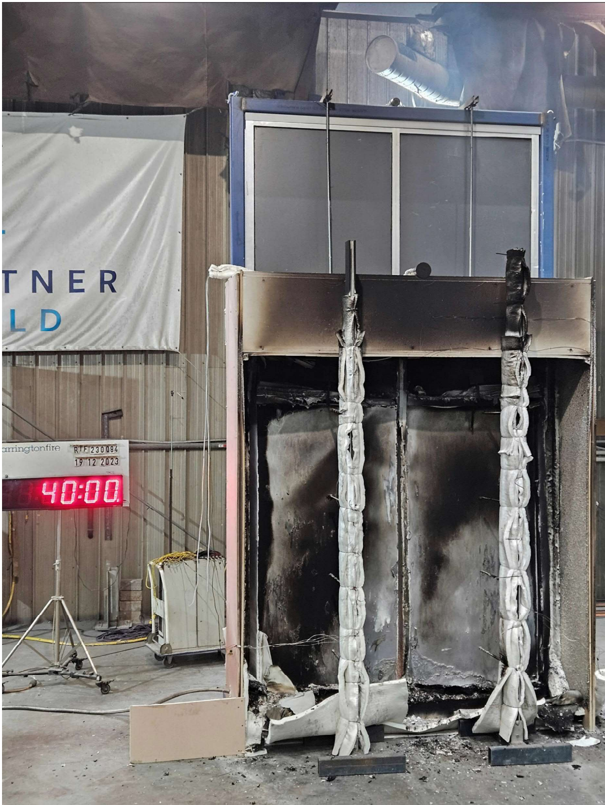
Figure 29 The specimen 10 minutes after the burner was turned off (40 minutes into the test)
