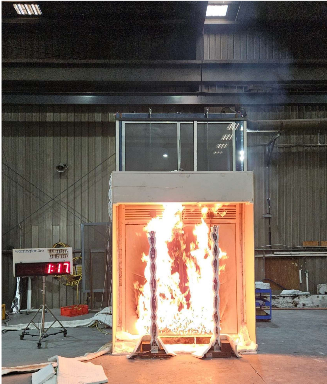
Figure 21 The specimen 1 minute 17 seconds into the test (burner output set to 500 kW)
