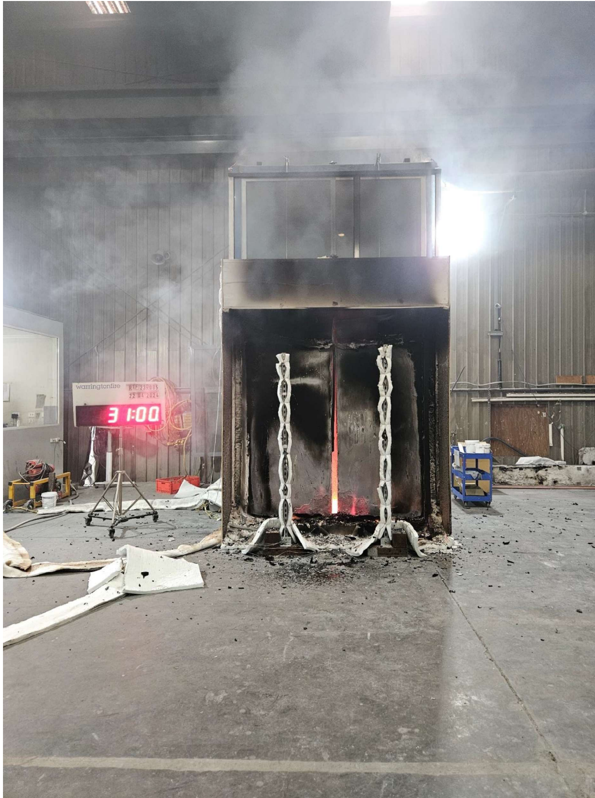
Figure 38 The specimen 1 minute after the burner was turned off (36 minutes into the test)
