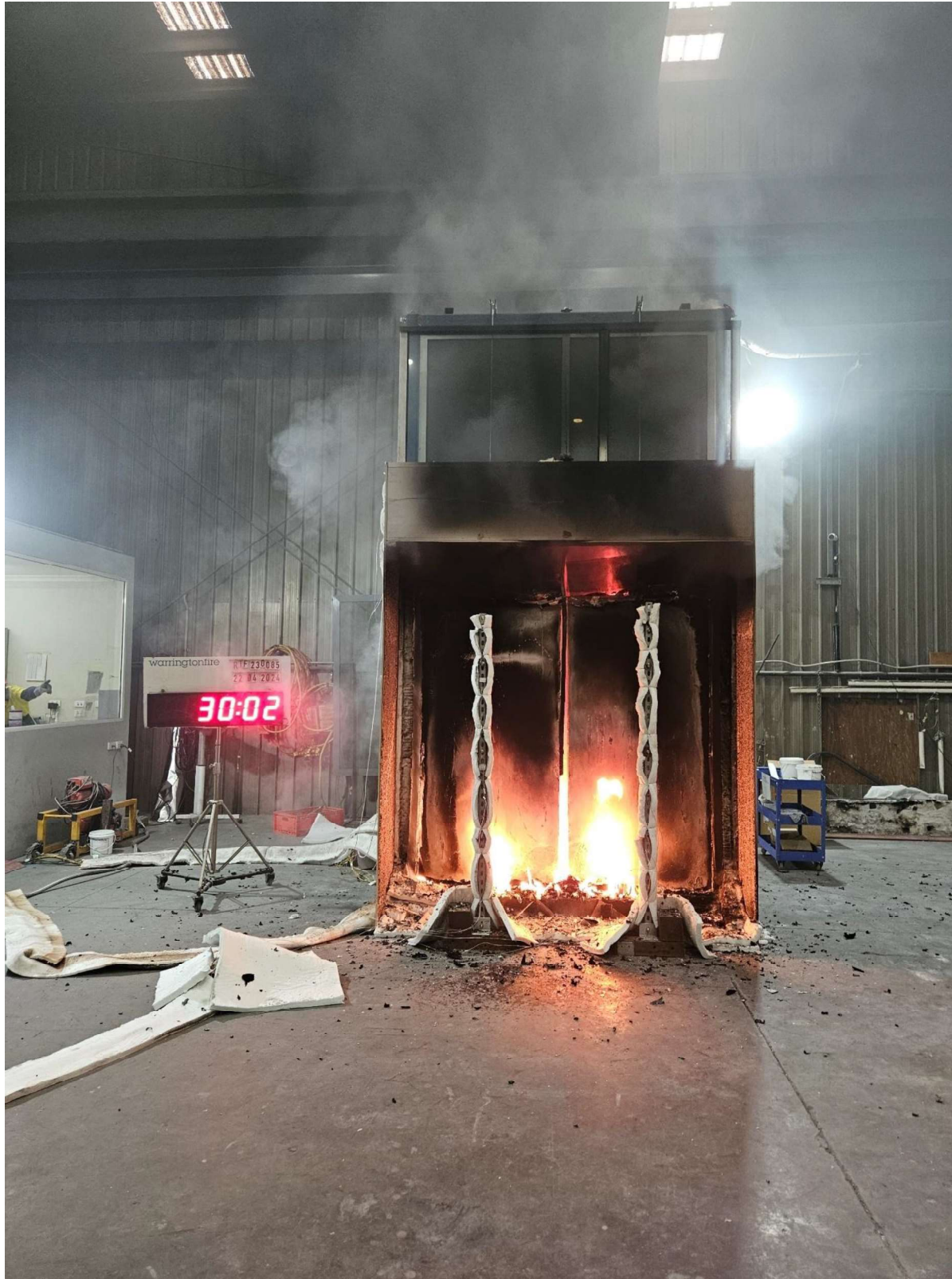
Figure 37 The specimen 2 seconds after the burner was turned off (30 minutes 2 seconds into the test)
