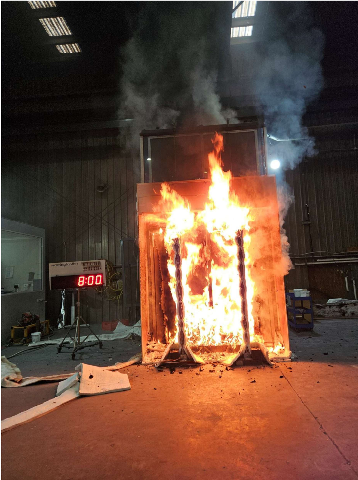
Figure 28 The specimen 8 minutes into the test
