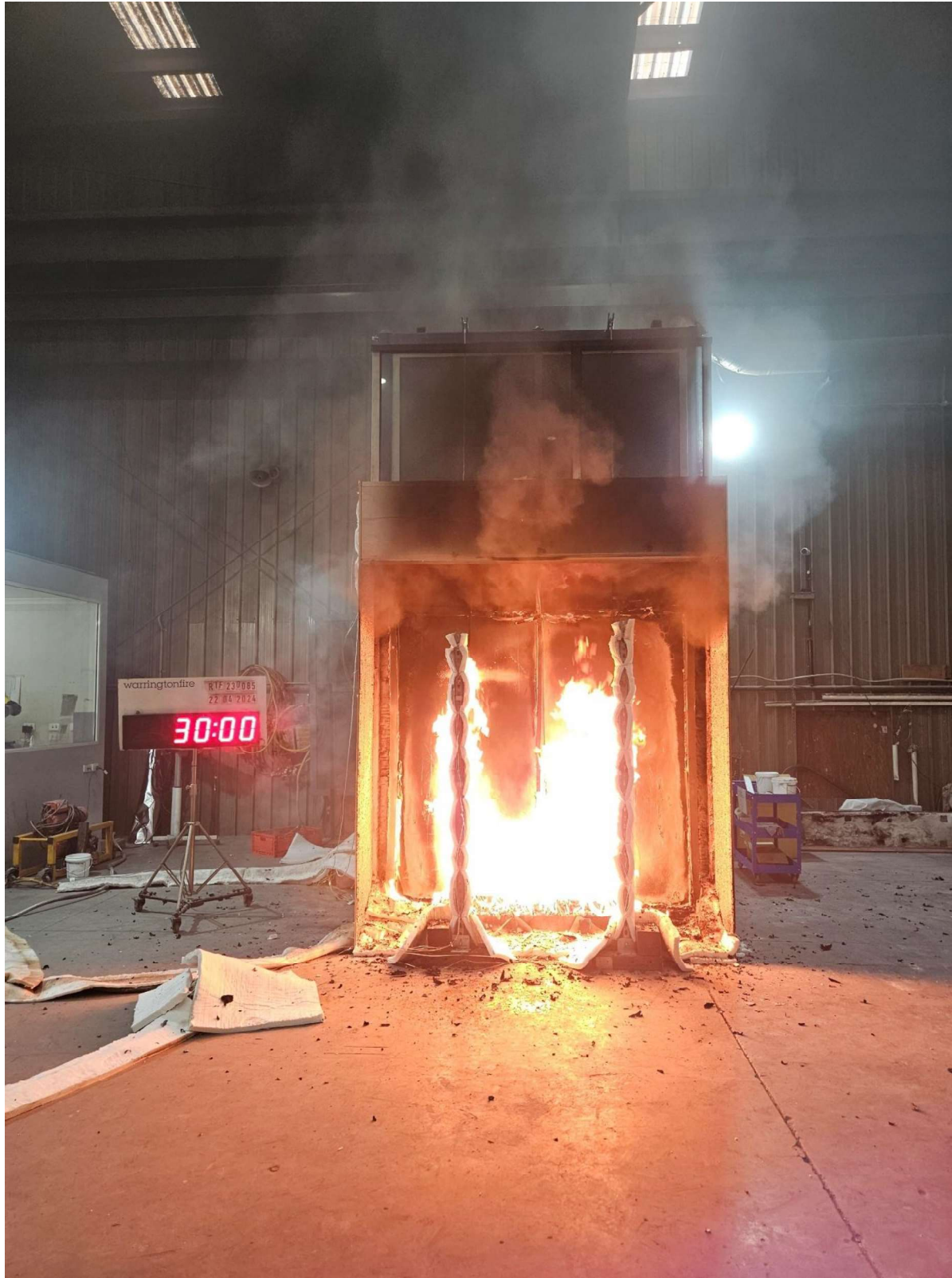
Figure 36 The specimen 30 minutes into the test – the burner was turned off.
