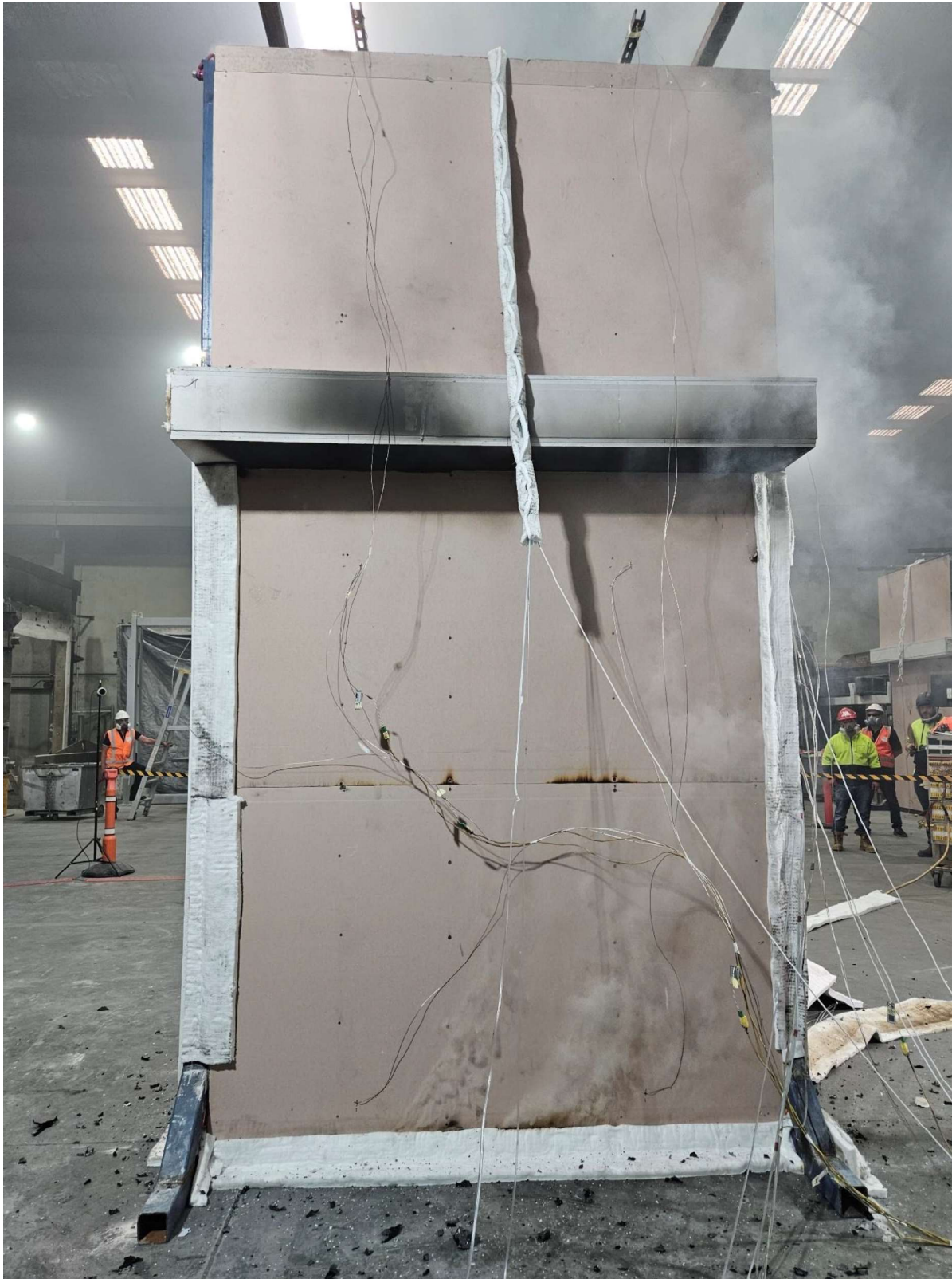
Figure 41 The specimen after the test – unexposed side.
