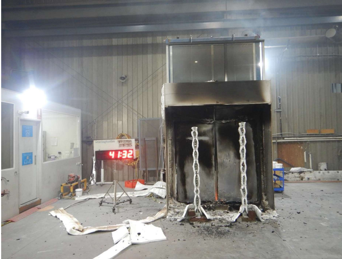
Figure 39 The specimen 11 minutes 32 seconds after the burner was turned off (41 minutes 32 seconds into the test)
