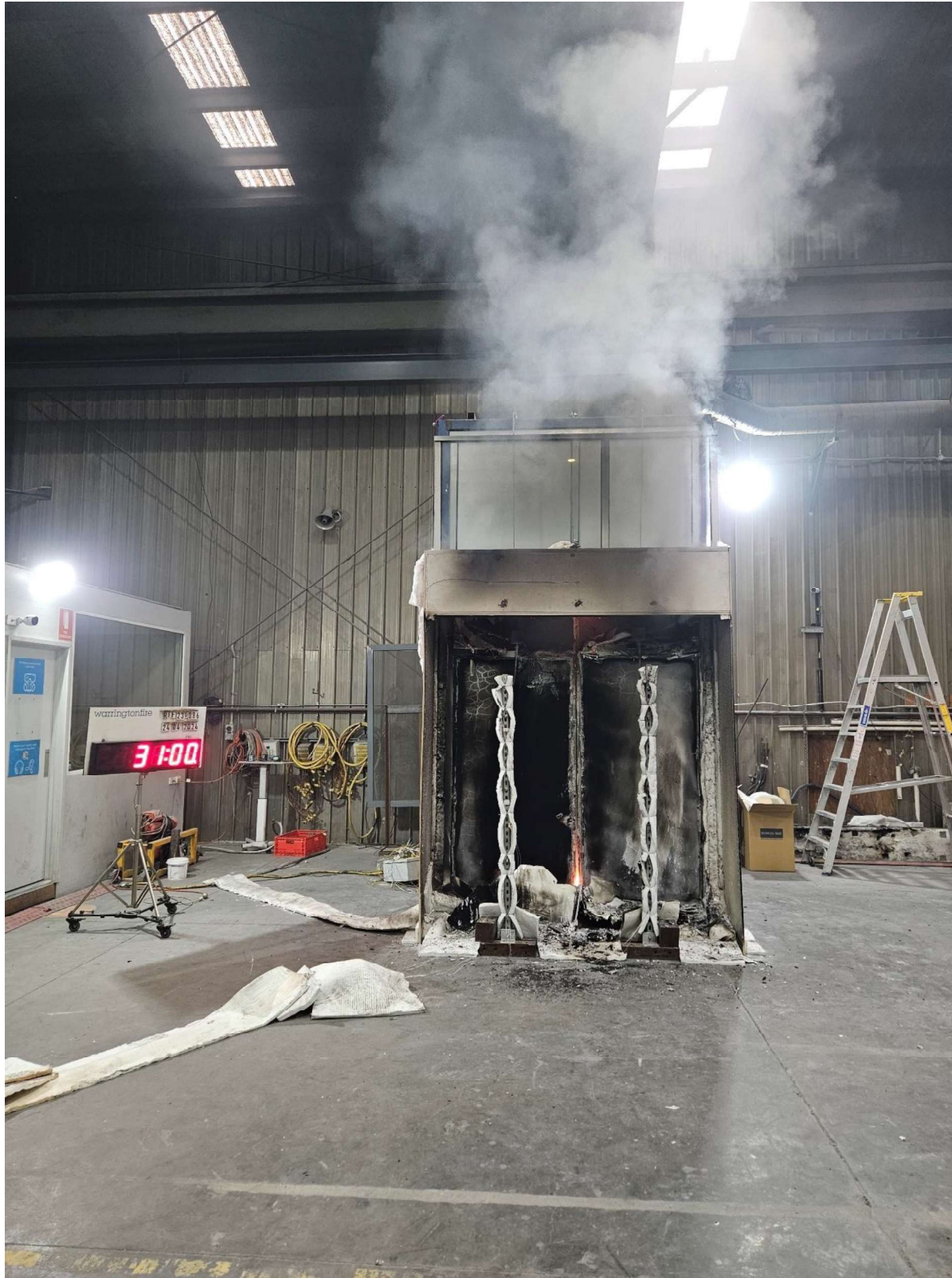
Figure 40 The specimen 1 minute after the burner was turned off (31 minutes into the test)
