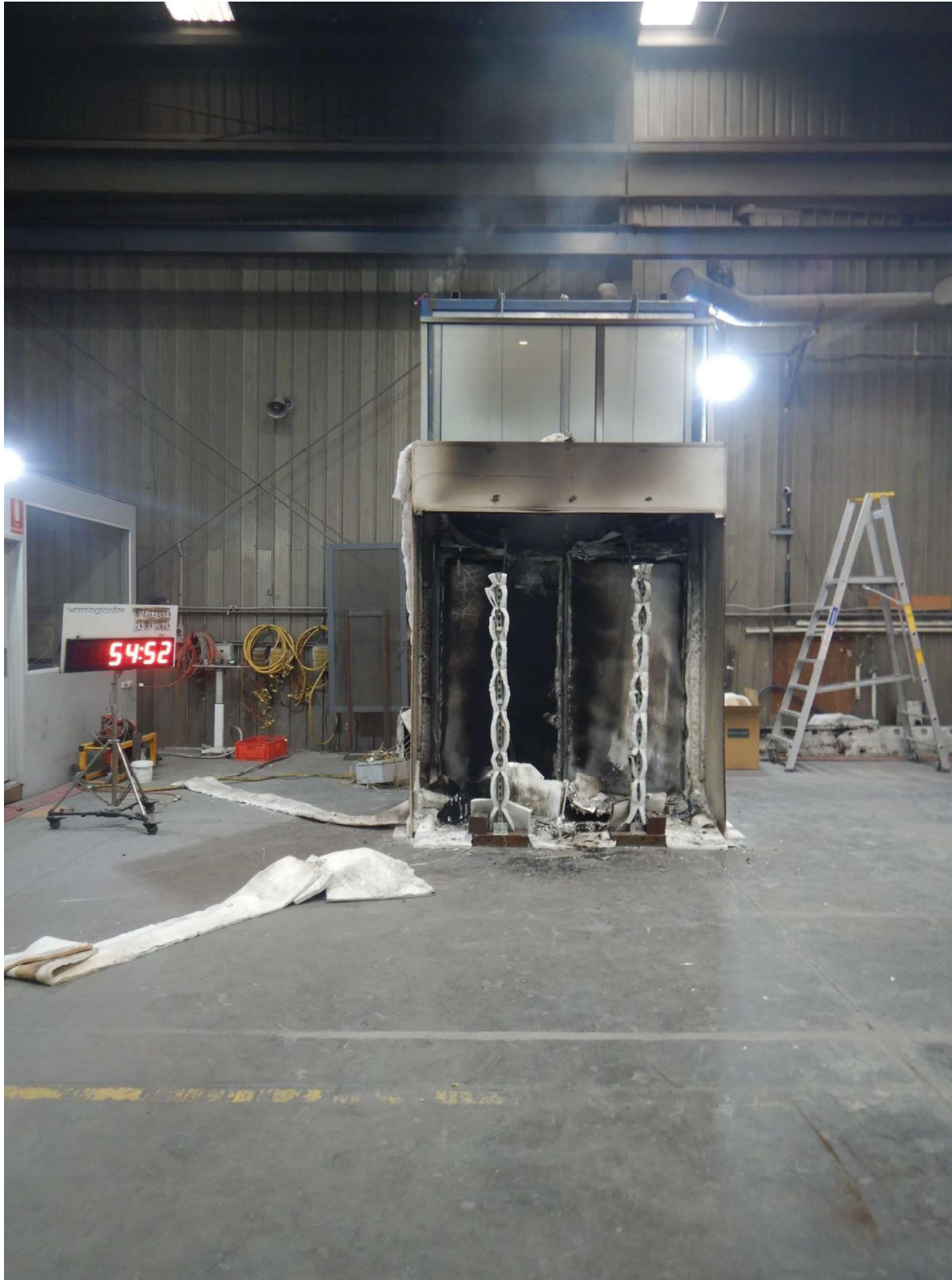
Figure 45 The specimen 24 minutes 52 seconds after the burner was turned off (54 minutes 52 seconds into the test)
