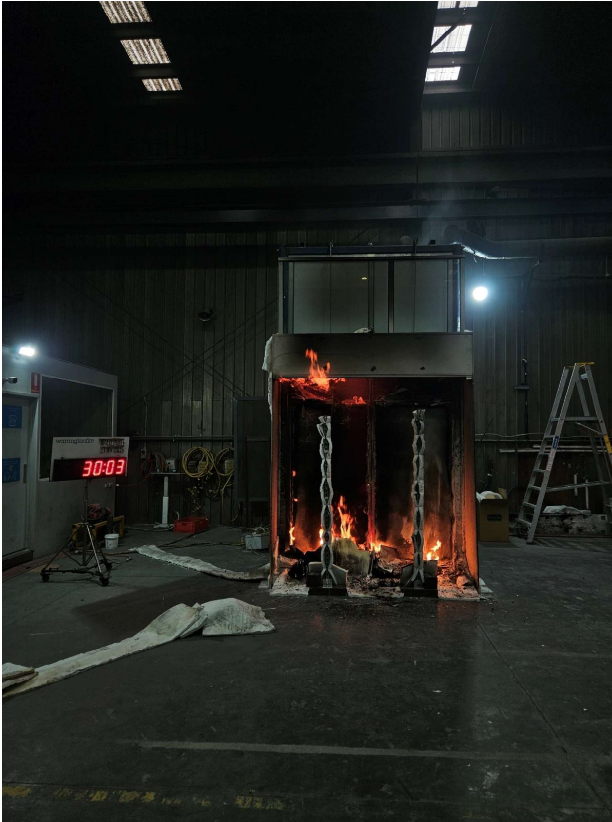
Figure 39 The specimen 3 seconds after the burner was turned off (30 minutes 3 seconds into the test)
