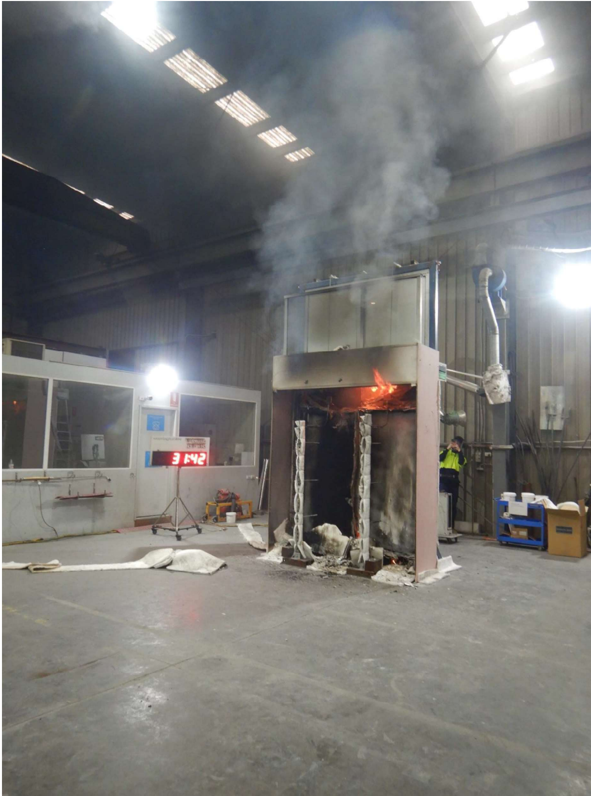
Figure 41 The specimen 1 minute 42 seconds after the burner was turned off (31 minutes 42 seconds into the test)
