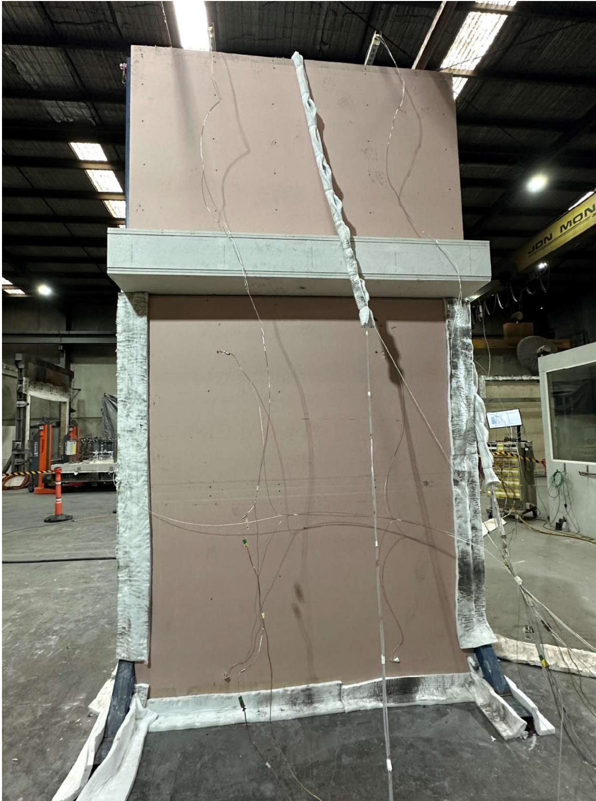
Figure 20 The specimen before the reaction to fire test – unexposed side
