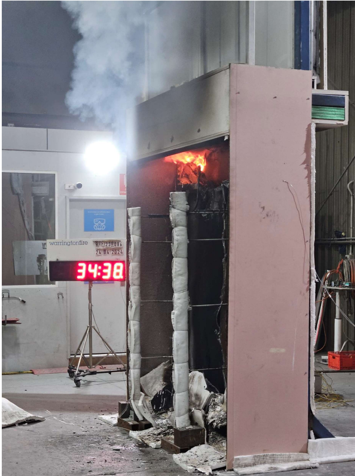
Figure 43 The specimen 4 minutes 38 seconds after the burner was turned off (34 minutes 38 seconds into the test)
