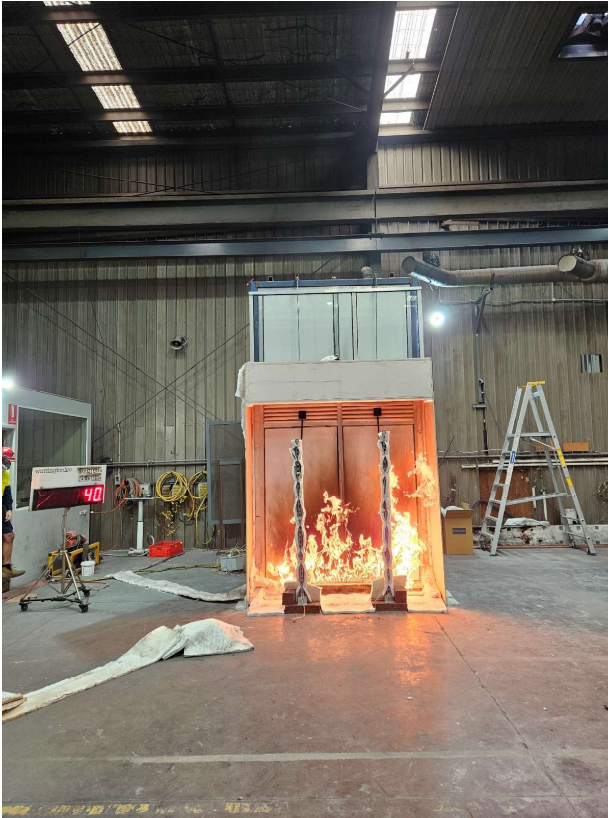
Figure 21 The specimen 40 seconds into the test (burner output set to 500 kW)
