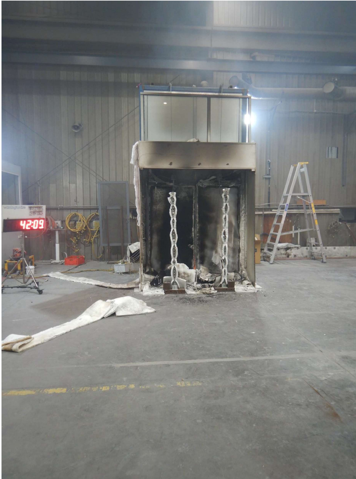
Figure 44 The specimen 22 minutes 9 seconds after the burner was turned off (42 minutes 9 seconds into the test)
