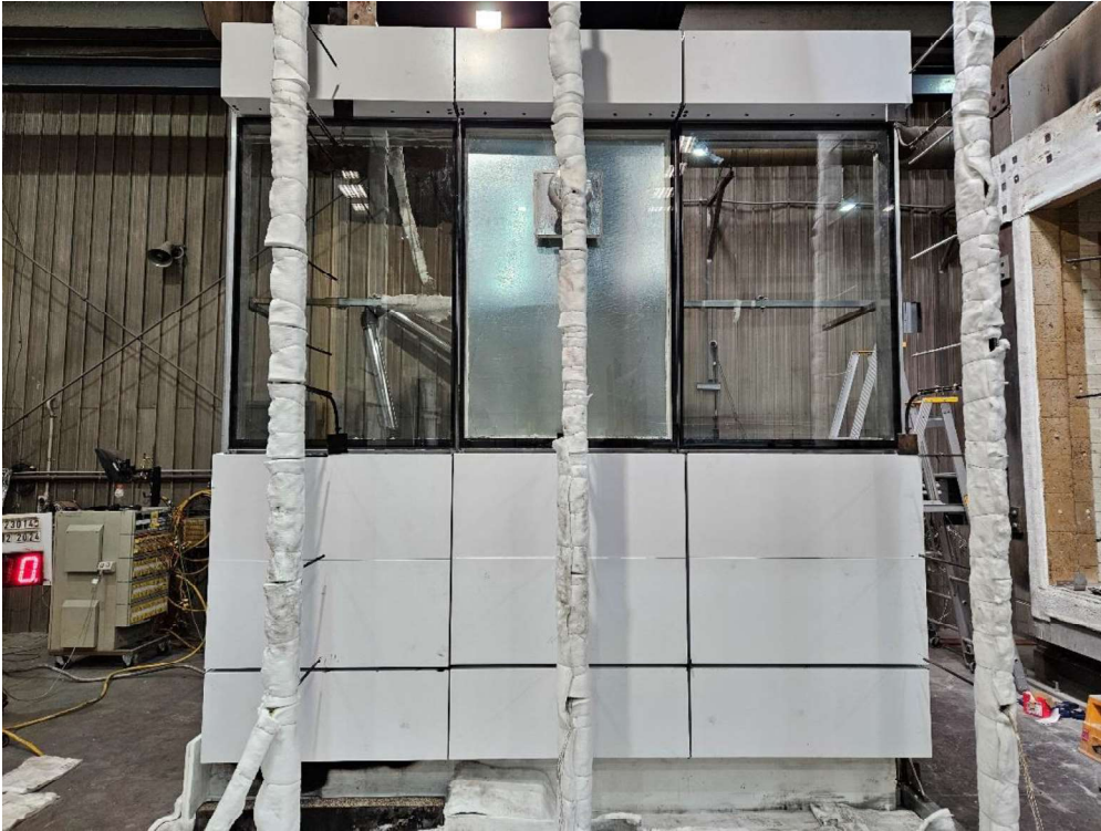
Figure 27 The specimen (exposed side) before the reaction to fire test
