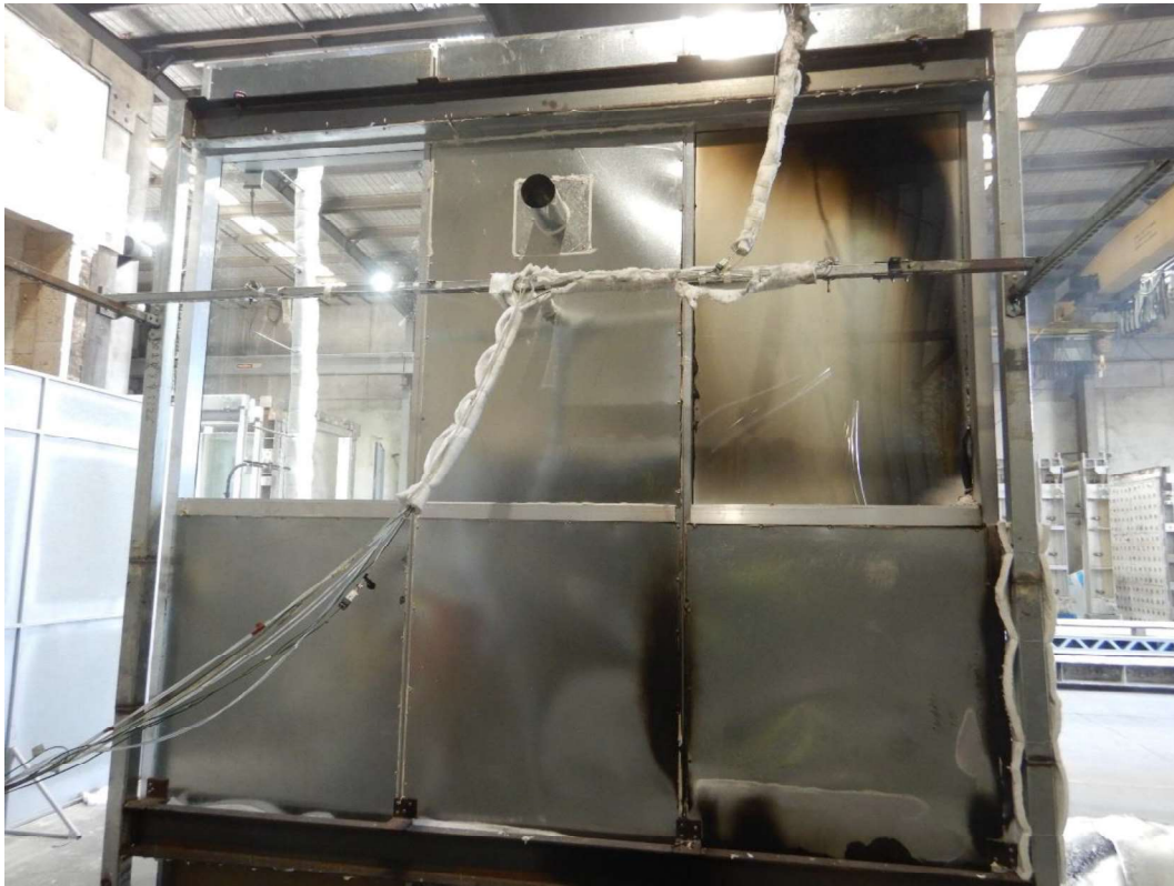
Figure 43 The specimen at end of test – unexposed side
