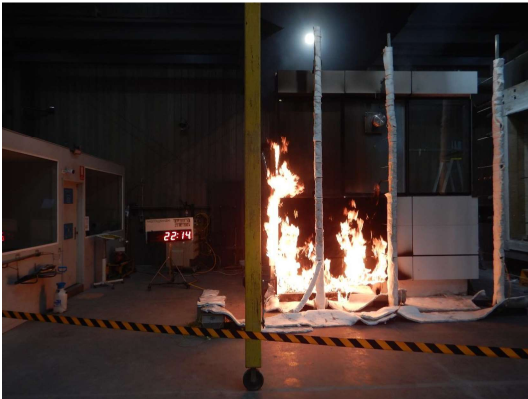
Figure 36 The specimen 22 minutes 14 seconds into the test (burner output at 300 kW)
