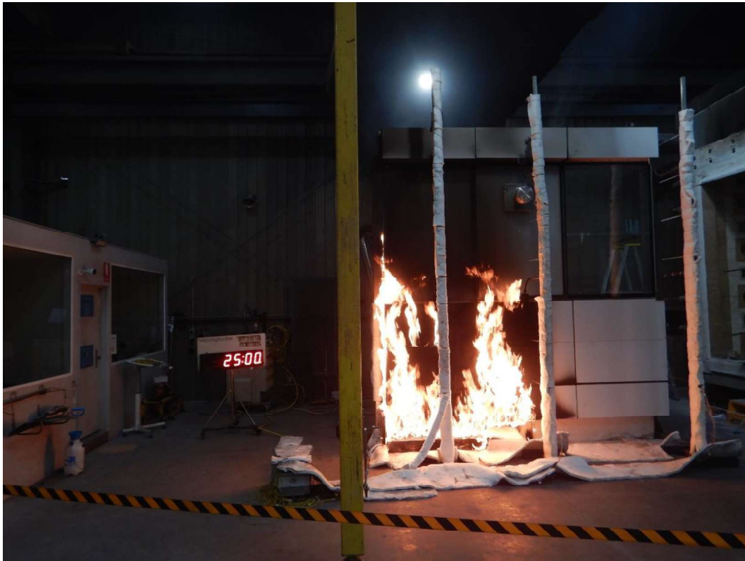
Figure 37 The specimen 25 minutes into the test (burner output at 300 kW)
