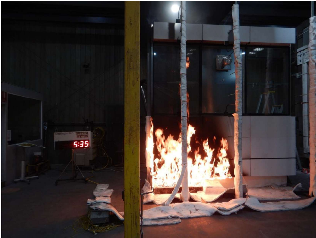
Figure 31 The specimen 5 minutes 35 seconds into the test (burner output at 300 kW)
