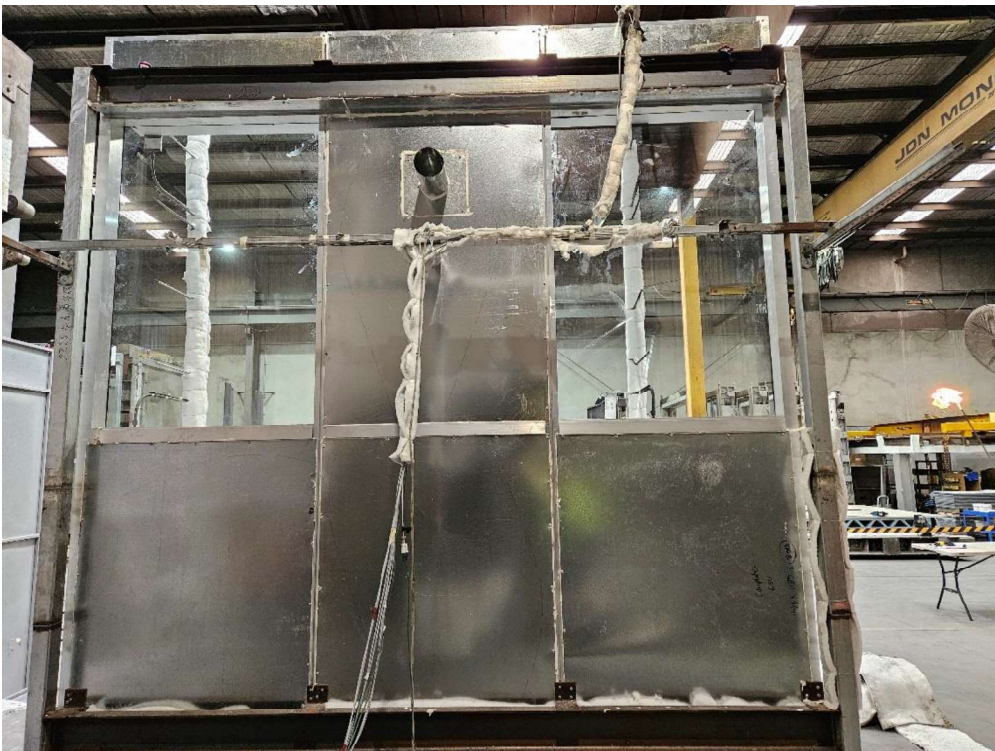
Figure 28 The specimen (unexposed side) before the reaction to fire test
