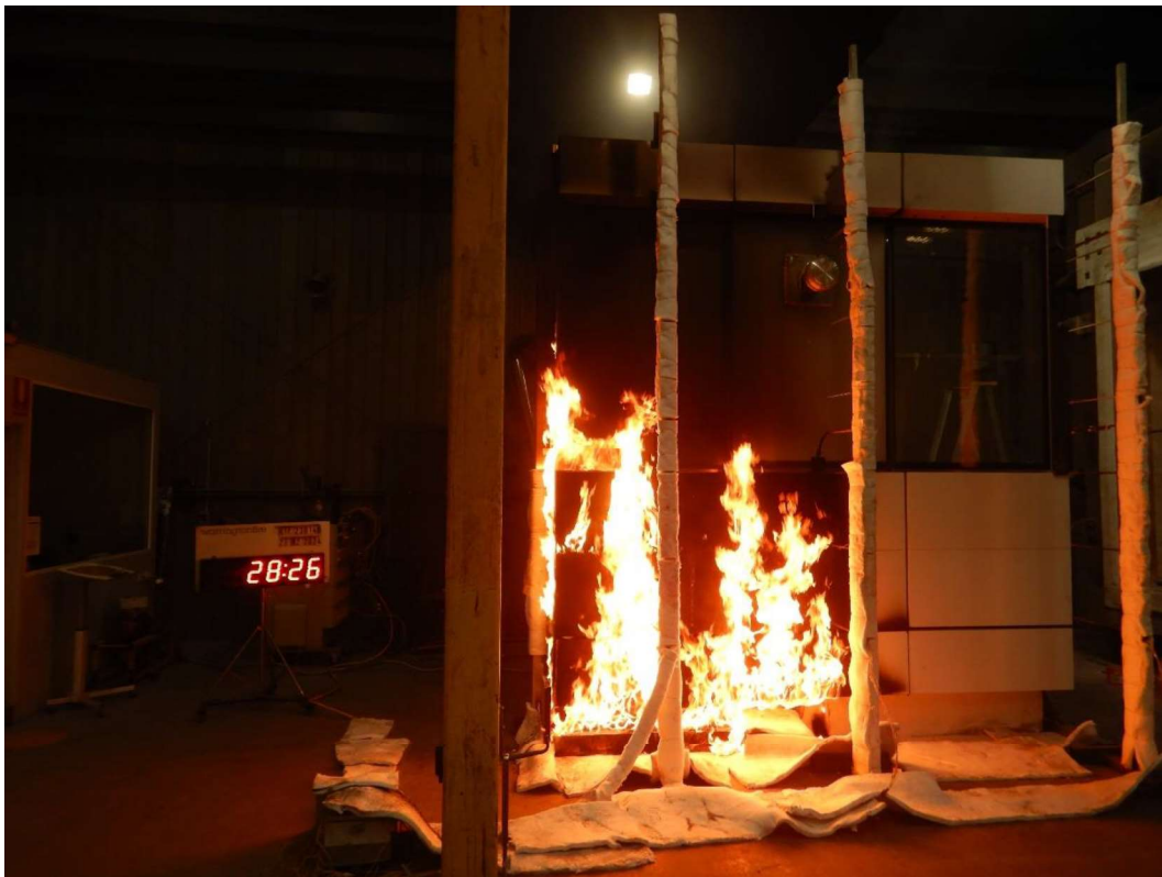
Figure 38 The specimen 28 minutes 26 seconds into the test (burner output at 300 kW)
