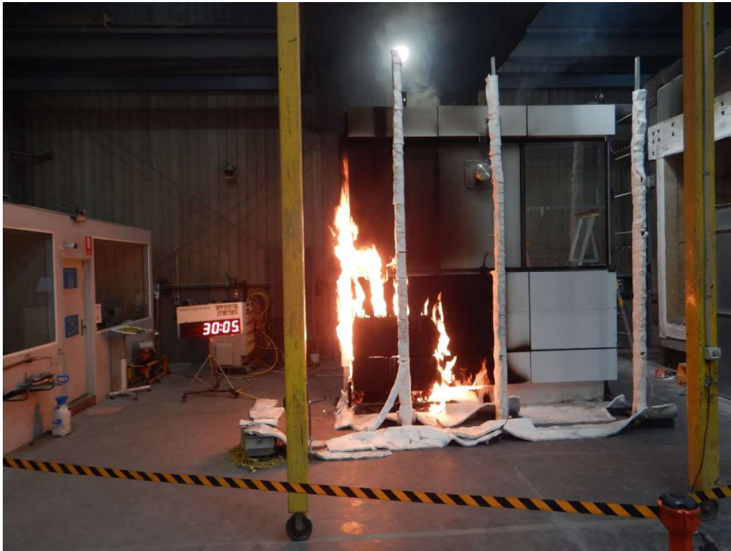
Figure 39 The specimen 30 minutes 5 seconds into the test (burner off)
