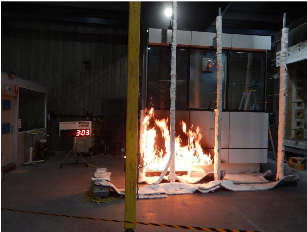
Figure 30 The specimen 3 minutes 3 seconds into the test (burner output at 300 kW)
