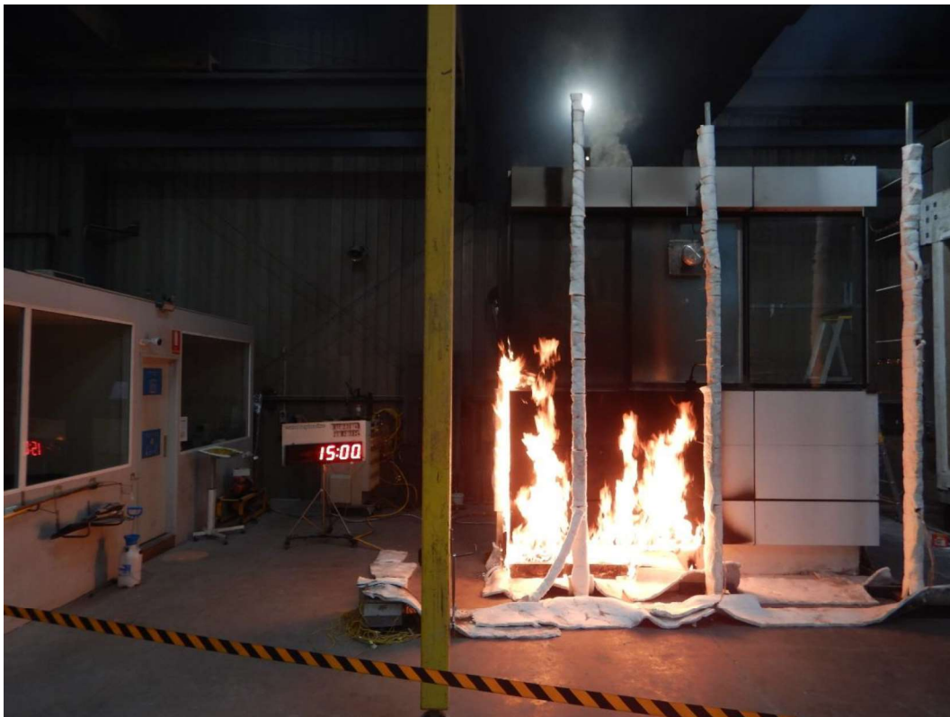
Figure 34 The specimen 15 minutes into the test (burner output at 300 kW)
