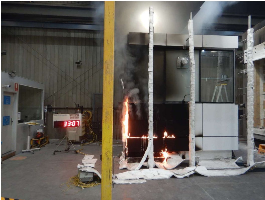
Figure 40 The specimen 33 minutes 7 seconds into the test (burner off)
