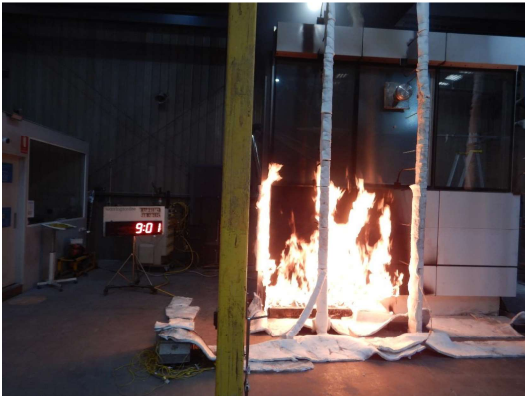
Figure 32 The specimen 9 minutes 1 second into the test (burner output at 300 kW)
