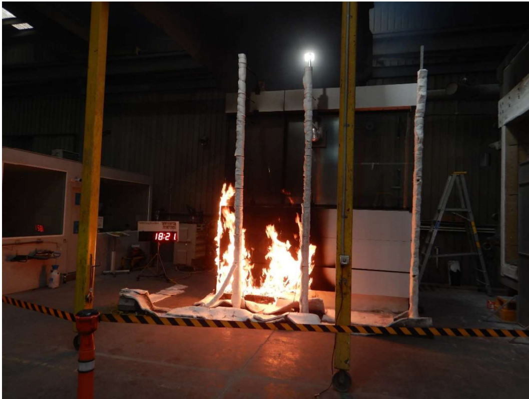
Figure 35 The specimen 18 minutes 21 seconds into the test (burner output at 300 kW)
