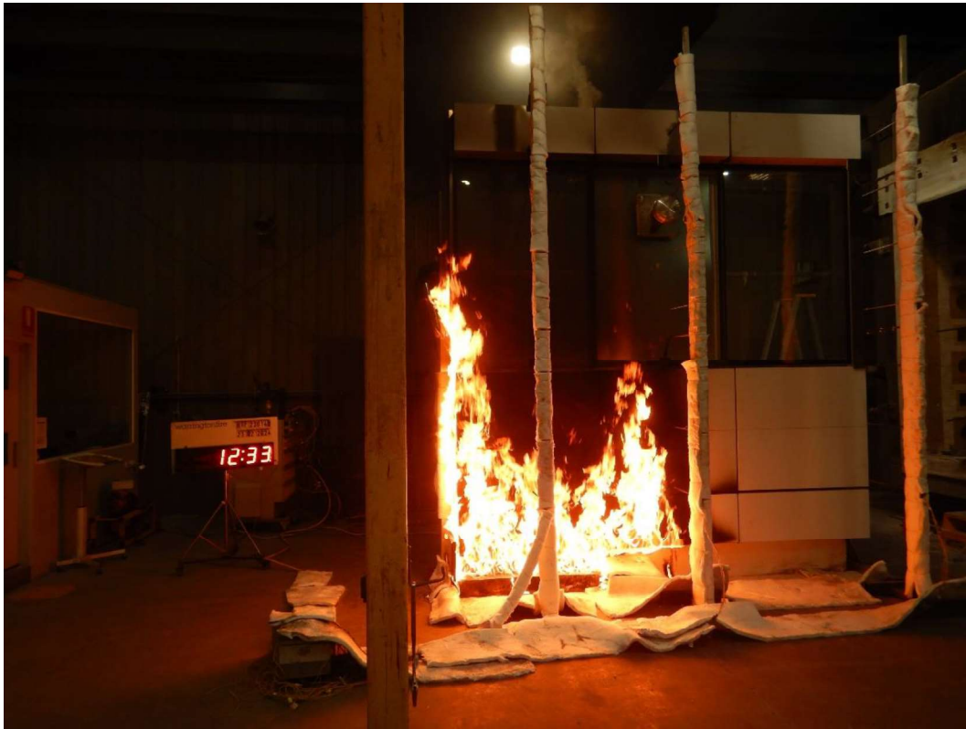
Figure 33 The specimen 12 minutes 33 seconds into the test (burner output at 300 kW)
