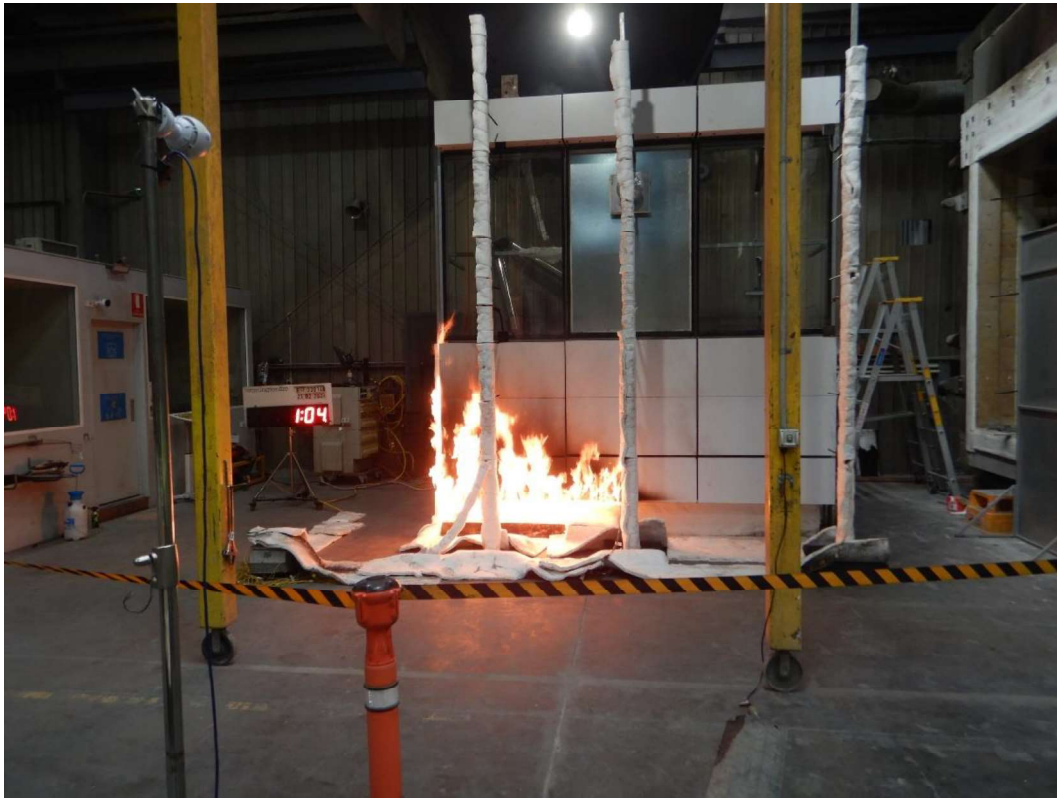
Figure 29 The specimen 1 minute 4 seconds into the test (burner output at 300 kW)
