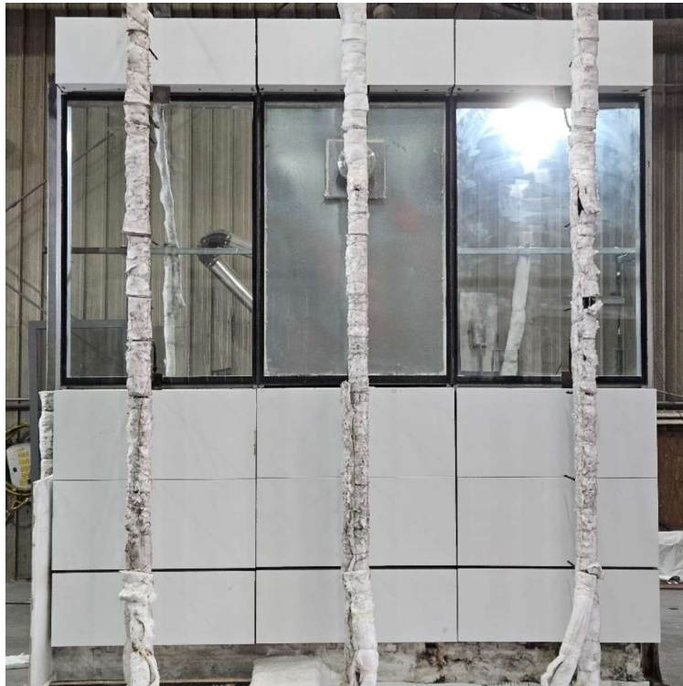
Figure 28 The specimen (exposed side) before the reaction to fire test
