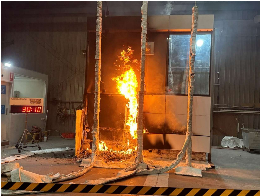
Figure 41 The specimen 30 minutes 10 seconds into the test (burner off)
