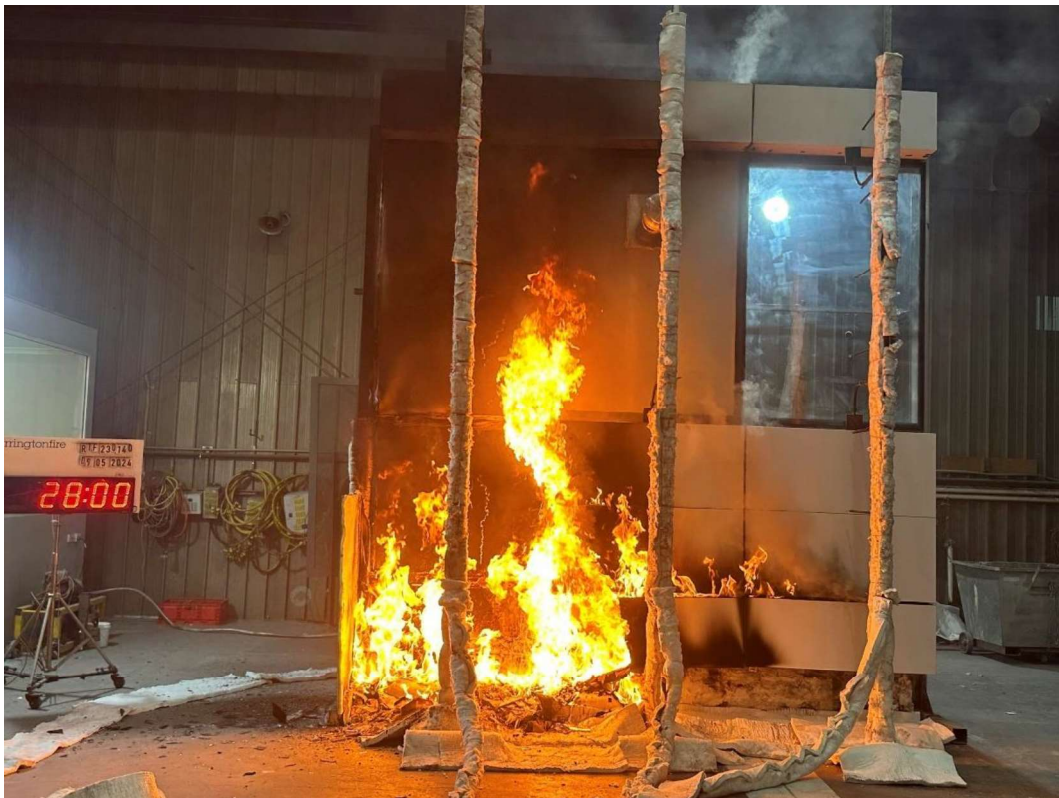
Figure 39 The specimen 28 minutes into the test (burner output at 300 kW)
