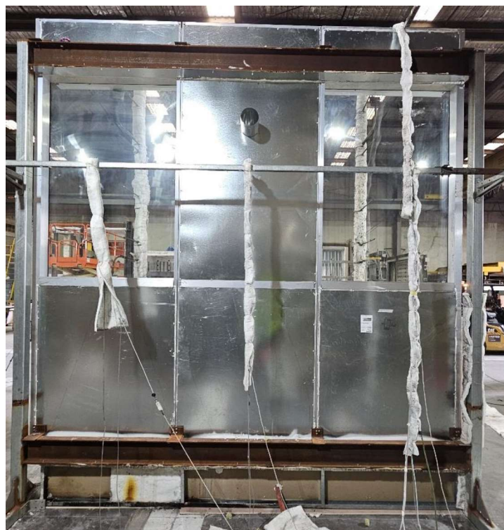
Figure 29 The specimen (unexposed side) before the reaction to fire test
