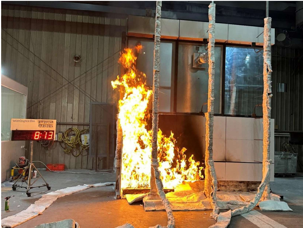
Figure 32 The specimen 8 minutes 13 seconds into the test (burner output at 300 kW)
