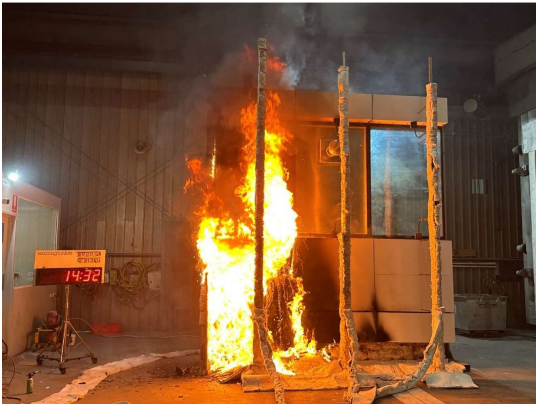
Figure 35 The specimen 14 minutes 32 seconds into the test (burner output at 300 kW)
