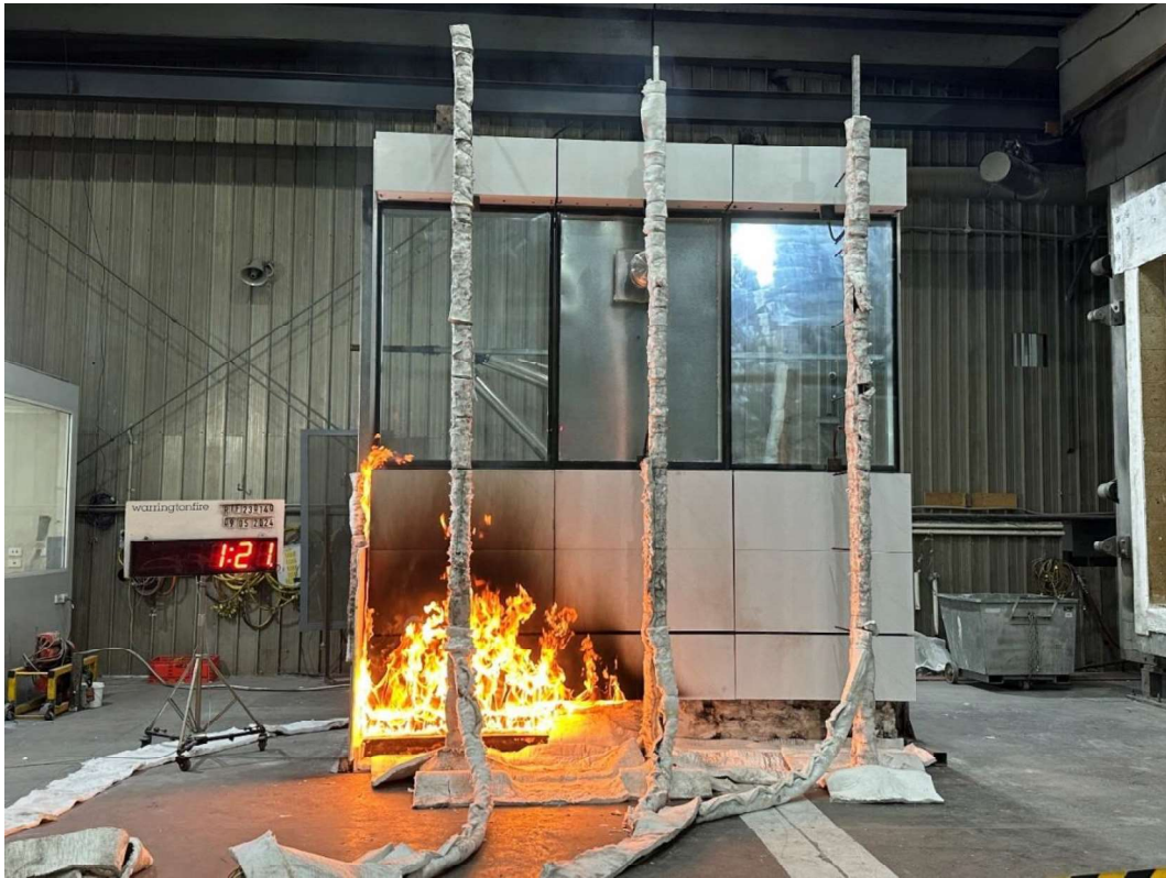
Figure 30 The specimen 1 minute 21 seconds into the test (burner output at 300 kW)
