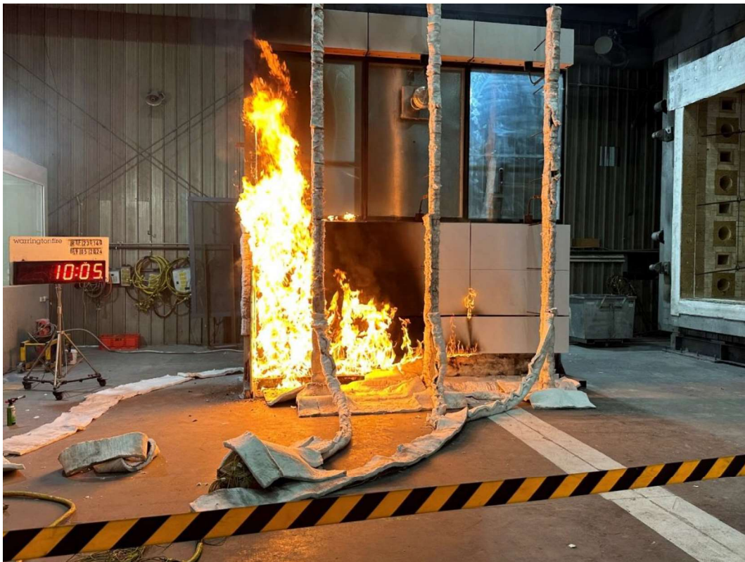
Figure 33 The specimen 10 minutes 5 seconds into the test (burner output at 300 kW)
