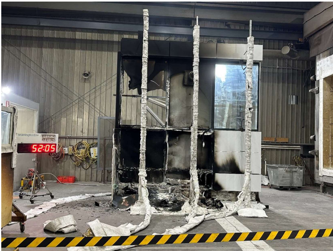
Figure 43 The specimen 52 minutes 5 seconds into the test (burner off)
