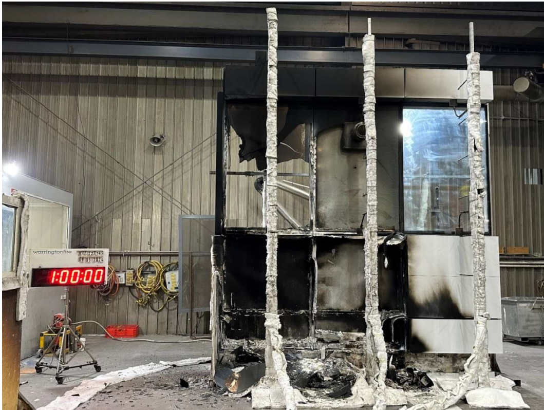
Figure 44 The specimen at end of test – exposed side
