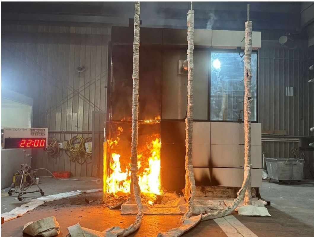
Figure 37 The specimen 22 minutes into the test (burner output at 300 kW)
