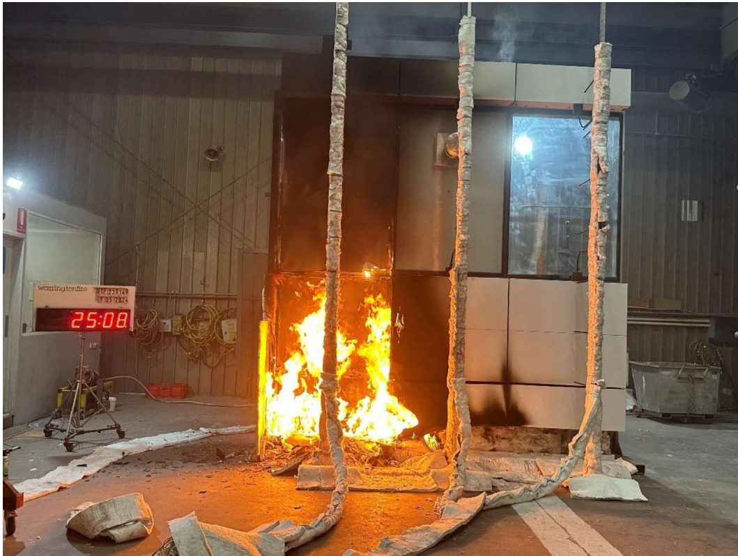
Figure 38 The specimen 25 minutes 8 seconds into the test (burner output at 300 kW)
