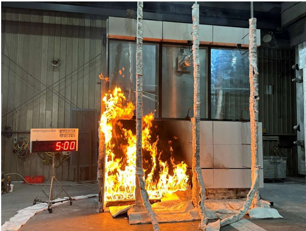
Figure 31 The specimen 5 minutes into the test (burner output at 300 kW)
