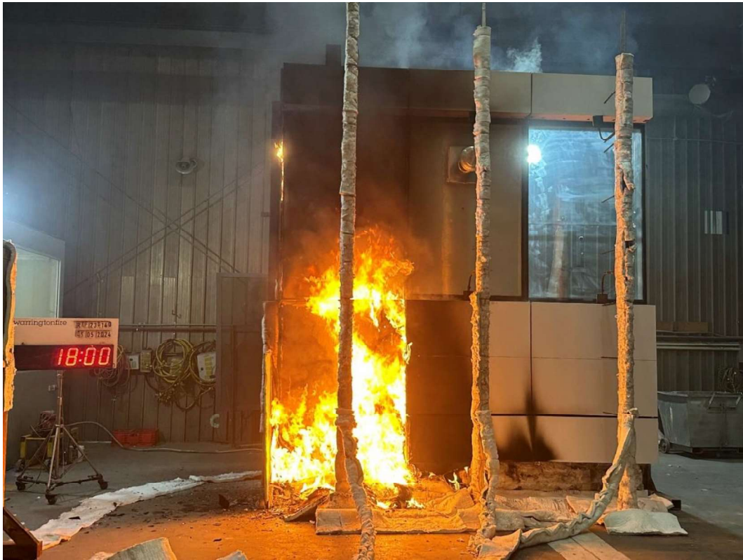
Figure 36 The specimen 18 minutes into the test (burner output at 300 kW)
