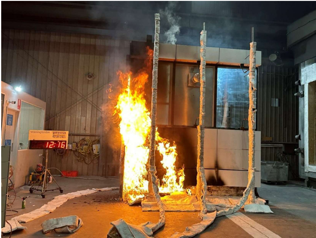
Figure 34 The specimen 12 minutes 16 seconds into the test (burner output at 300 kW)
