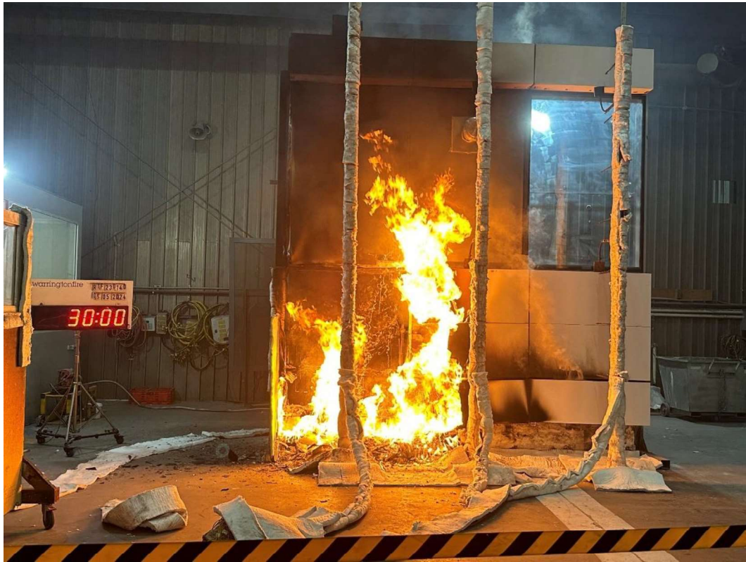
Figure 40 The specimen 30 minutes into the test (burner output at 300 kW)
