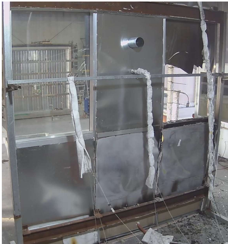
Figure 45 The specimen at end of test – unexposed side
