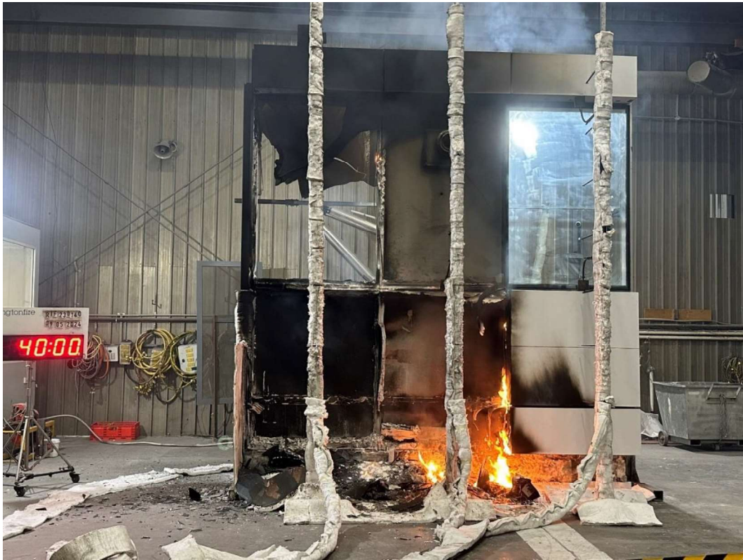
Figure 42 The specimen 40 minutes into the test (burner off)
