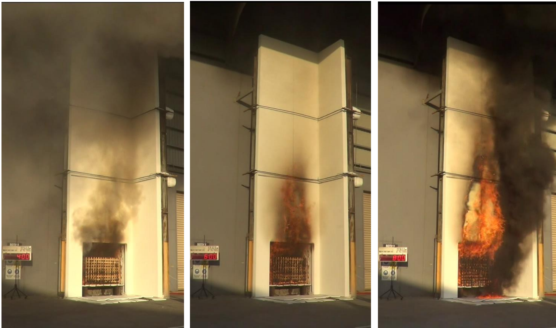
Figure 7. Rendered EPS external wall system at 4 minutes (left), 6 minutes (centre) and 8 minutes (right) after crib ignition
