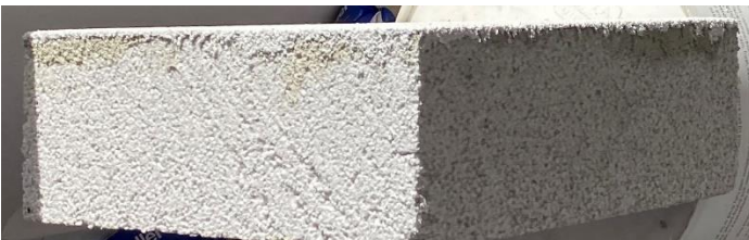
Figure 6. Cut section of 100 mm thick EPS with 1 mm base coat render to one side (left over section not installed to specimen) during CSIRO inspection of completed construction at Warringtonfire.
