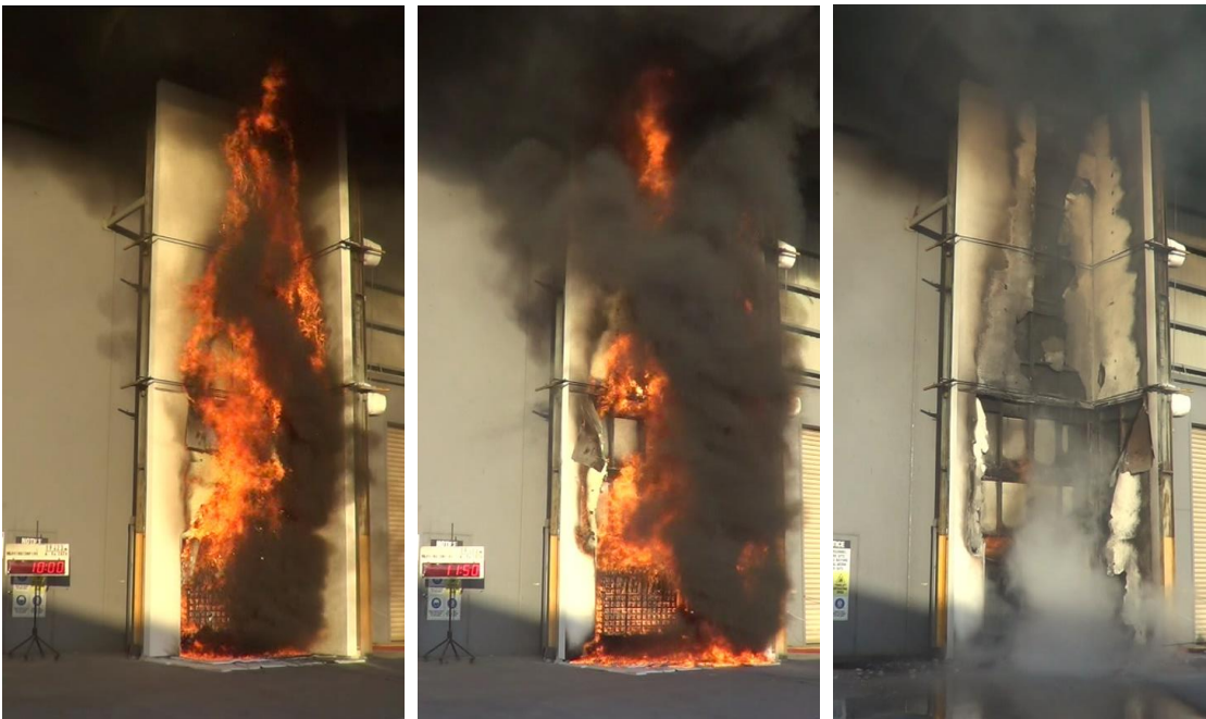
Figure 8. Rendered EPS external wall system at 10 minutes (left), 11:50 minutes (centre), immediately after water suppression (right)
