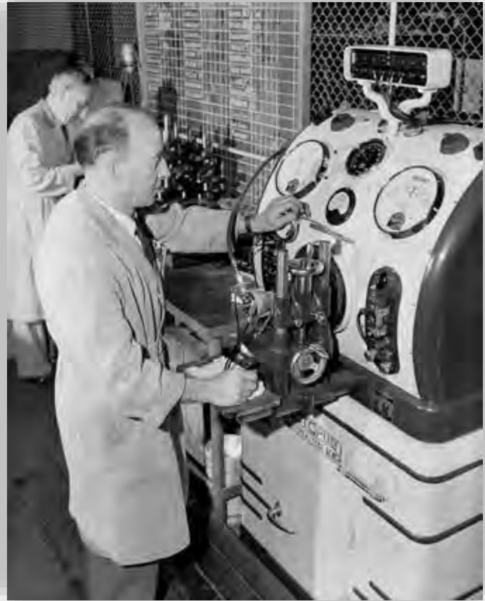
Figure 61: Testing and inspection of component parts before assembly is a feature of production methods, at the plant of the Standard Motor Company (Australia) Pty Ltd, at Fishermen's Bend, Victoria - Here a distributor is being electrically tested and adjusted, 1956, National Archives of Australia, A1200, L21179
