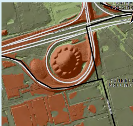
Figure 64: Example of Integrating Open Space and a Soil Repository, Entry ramp from Westgate Freeway onto CityLink
