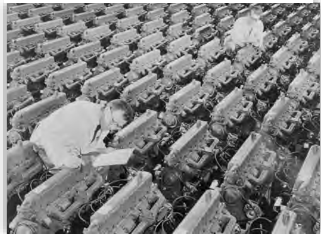
Figure 31: Checkers examine new Holden engines at the engine assembly plant at Fisherman's Bend near Melbourne, 1963, National Archives of Australia: A1200, L45049
