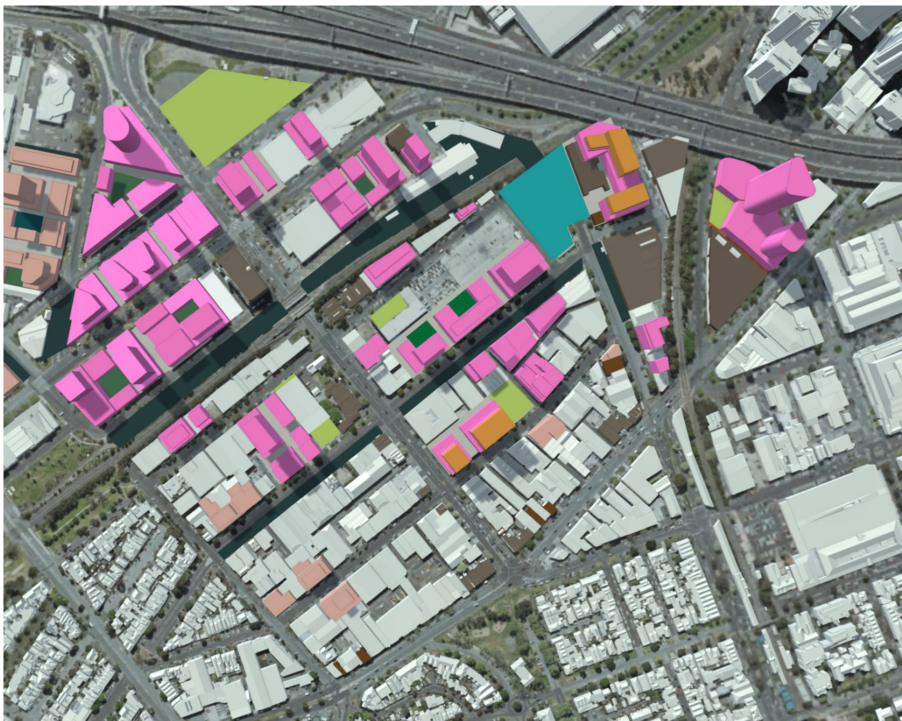
Figure 3 Montague plan view: In this illustration all sites are also modelled to the proposed FAR of 6.3 (core area) and 3.6 (non-core area) and in compliance with the built envelope controls (including overshadowing requirements). This demonstrates a variety of potential design responses that are possible within the proposed controls.
