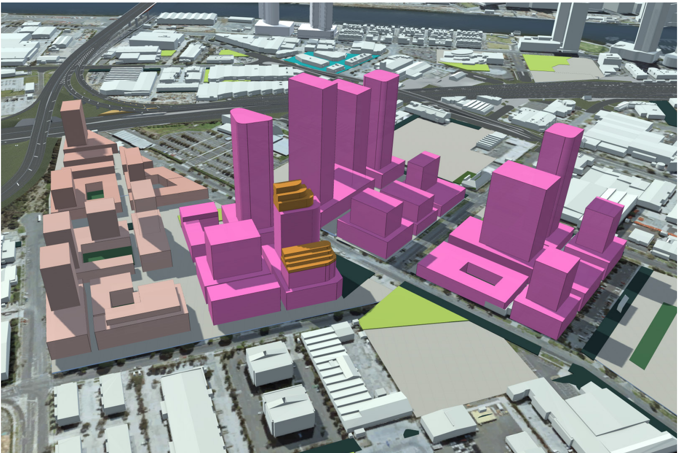
Figure 15 An potential design outcome for four blocks in Sandridge (view from south). In this example all sites are also modelled to the proposed FAR of 7.4 in the core area (taking into account recommendations in this report) and 3.3 in the non-core area and in compliance with the built envelope controls (including overshadowing requirements for the new parks). This demonstrates a variety of potential design responses that are possible within the proposed controls.
