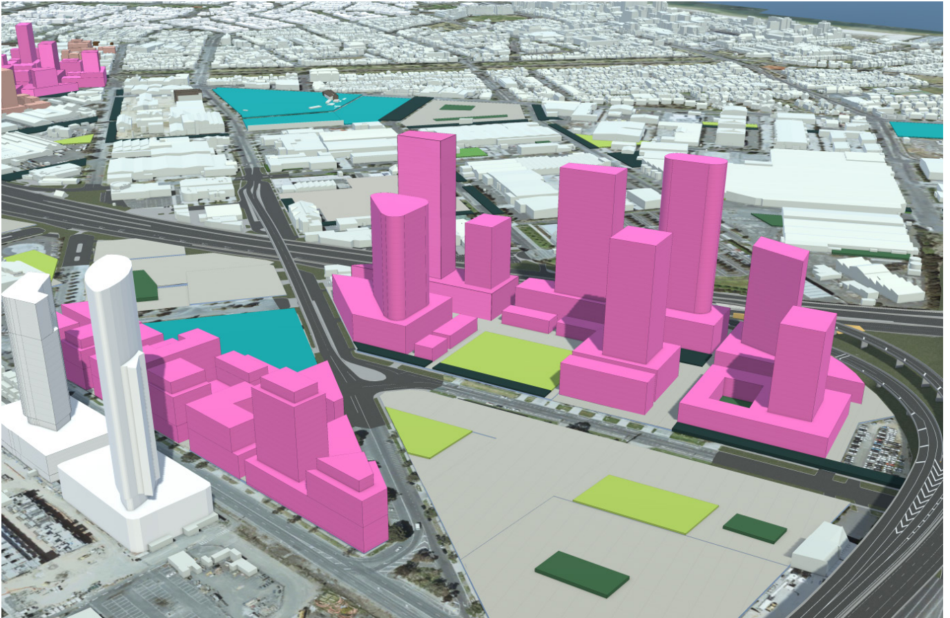
Figure 13 A potential design outcome for two blocks in Lorimer (view from north). In this example all sites are also modelled to the proposed FAR of 5.4 and in compliance with the built envelope controls (including overshadowing requirements for the new park). This demonstrates a variety of potential design responses that are possible within the proposed controls.
