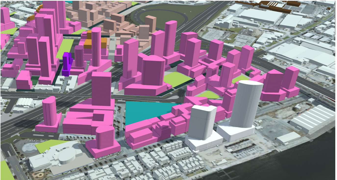
Figure 6 Lorimer perspective view: In this illustration all sites are also modelled to the proposed FAR of 5.4 and in compliance with the built envelope controls (including overshadowing requirements). This demonstrates a variety of potential design responses that are possible within the proposed controls.
