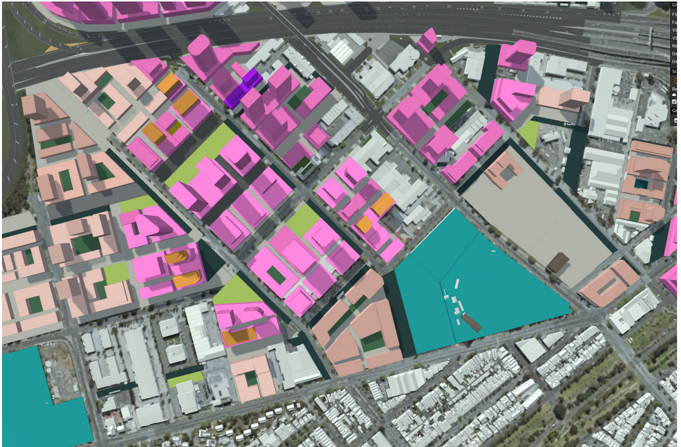
Figure 7 Sandridge plan view: In this illustration all sites are also modelled to the proposed FAR of 7.4 (core area) and 3.3 (non-core area) and in compliance with the built envelope controls (including overshadowing requirements). This demonstrates a variety of potential design responses that are possible within the proposed controls, including the delivery of family-friendly housing (mid-rise buildings with communal open space in the non-core area)
