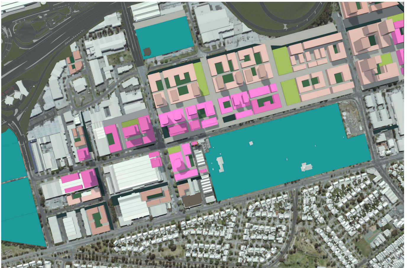
Figure 10 Wirraway plan view: In this illustration all sites are also modelled to the proposed FAR of 4.1 (core area) and 2.1 (non-core area) and in compliance with the built envelope controls (including overshadowing requirements). This demonstrates a variety of potential design responses that are possible within the proposed controls, including the delivery of family-friendly housing (mid-rise buildings with communal open space in the non-core area)
