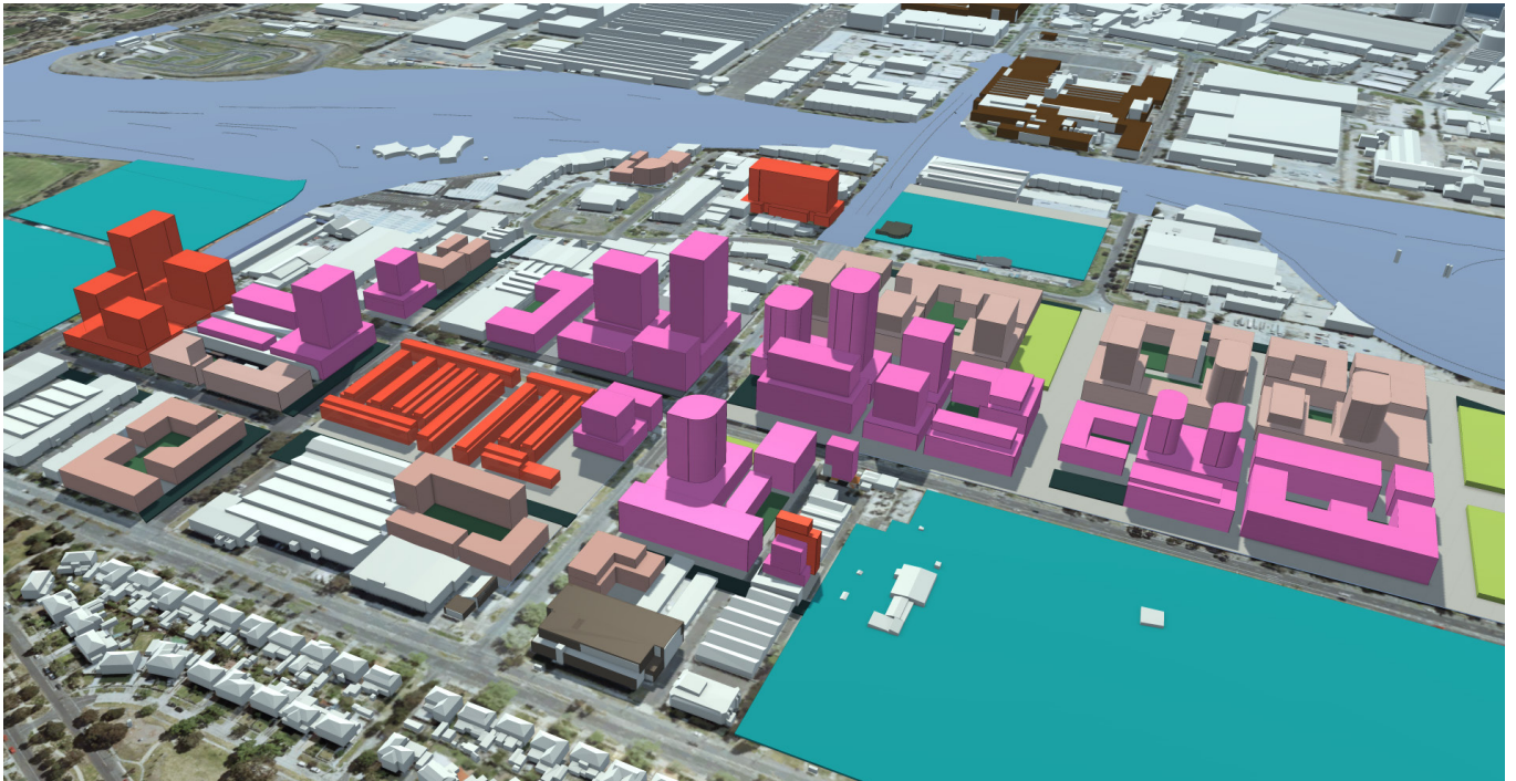
Figure 12 Wirraway perspective view (from south focused on core area): In this illustration all sites are also modelled to the proposed FAR of 4.1 (core area) and 2.1 (non-core area) and in compliance with the built envelope controls (including overshading requirements). This demonstrates a variety of potential design responses that are possible within the proposed controls, including the delivery of family-friendly housing (mid-rise buildings with communal open space in the non-core area)
