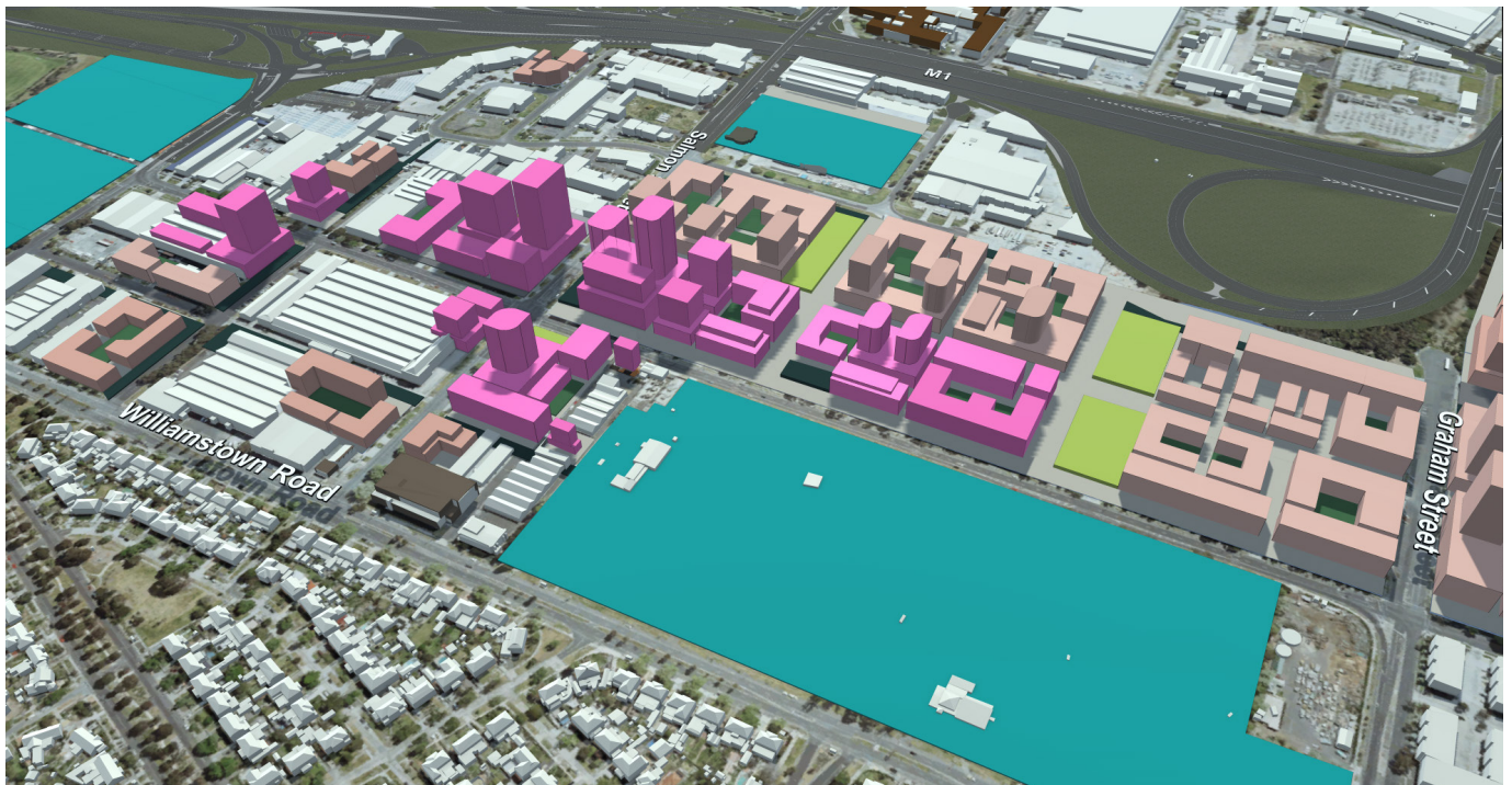
Figure 11 Wirraway perspective view (view from south): In this illustration all sites are also modelled to the proposed FAR of 4.1 (core area) and 2.1 (non-core area) and in compliance with the built envelope controls (including overshadowing requirements). This demonstrates a variety of potential design responses that are possible within the proposed controls, including the delivery of family-friendly housing (mid-rise buildings with communal open space in the non-core area)
