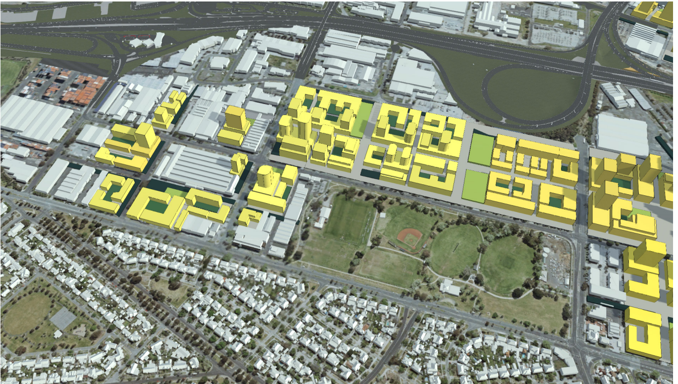
Figure 6 Wirraway perspective view - the application of the FAR together with all proposed building envelope controls support the delivery of the open space without loss of development yield on any site.
