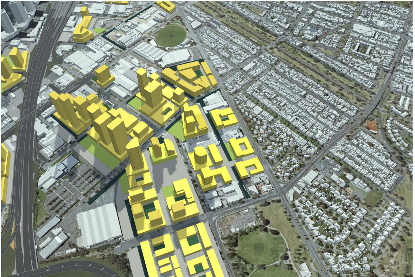
Figure 5 Sandridge perspective view - the application of the FAR together with all proposed building envelope controls support the delivery of the open space without loss of development yield on any site.
