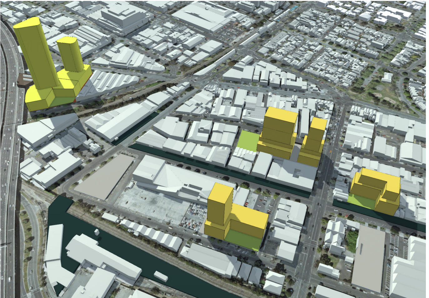
Figure 2 Montague perspective view - the application of the FAR together with all proposed building envelope controls support the delivery of the open space without loss of development yield on any site.
