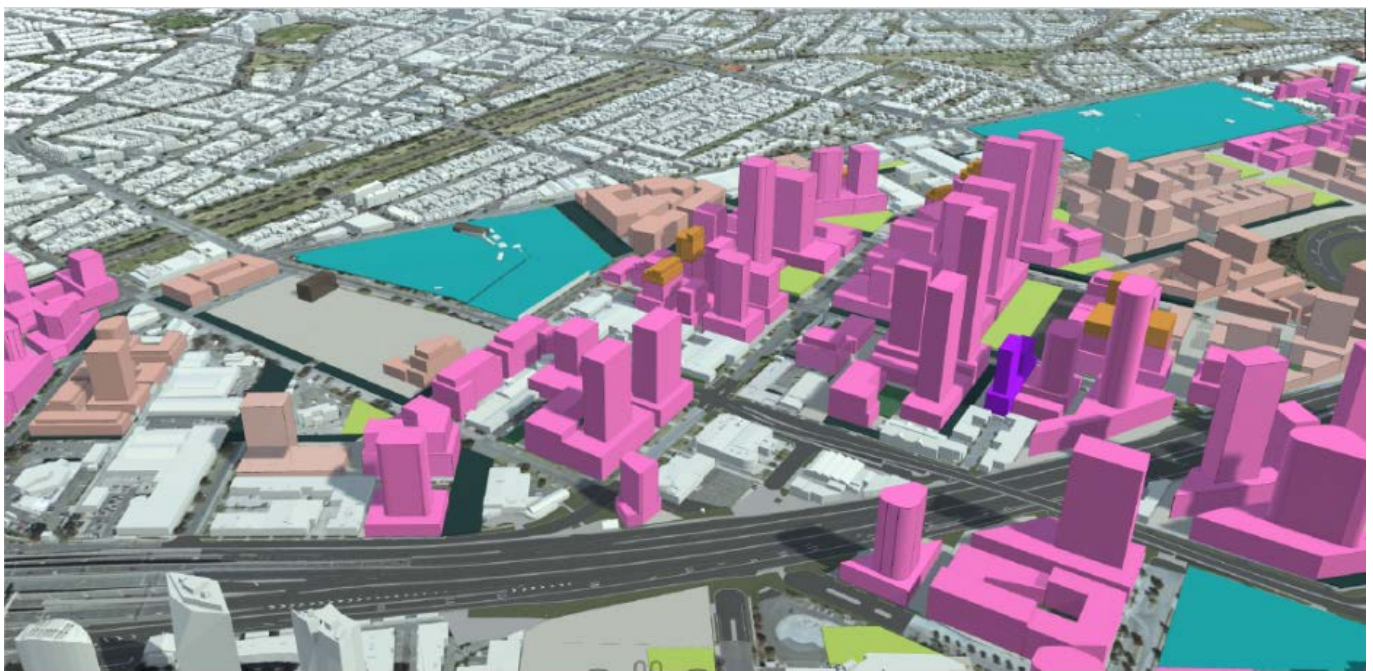
Figure 9 Sandridge perspective view (from the north): In this illustration all sites are also modelled to the proposed FAR of 7.4 (core area) and 3.3 (non-core area) and in compliance with the built envelope controls (including overshadowing requirements). This demonstrates a variety of potential design responses that are possible within the proposed controls, including the delivery of family-friendly housing (mid-rise buildings with communal open space in the non-core area)
