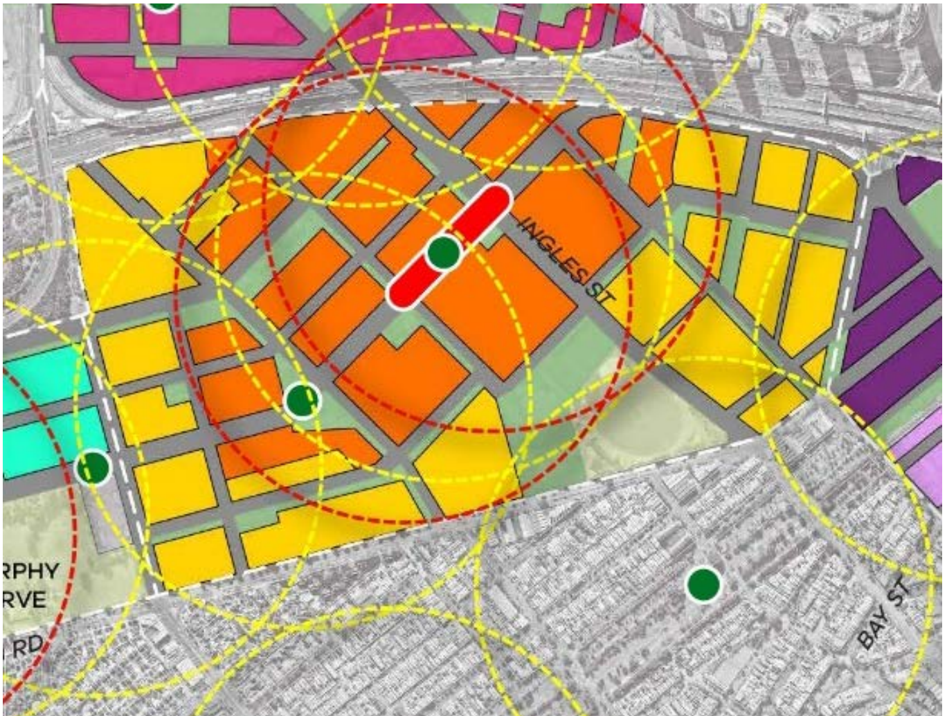
400m (approx. 5 minute) walkable catchments from proposed train stations (red) and existing and indicative tram stops (stops in green, catchments in yellow)
