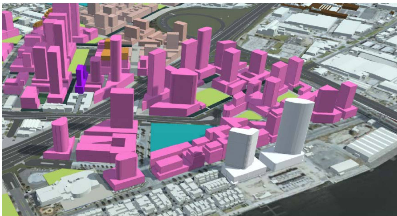
Figure 6 Lorimer perspective view: In this illustration all sites are also modelled to the proposed FAR of 5.4 and in compliance with the built envelope controls (including overshadowing requirements). This demonstrates a variety of potential design responses that are possible within the proposed controls.
