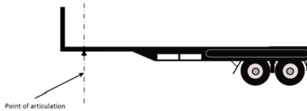
Figure 7: Illustration of point of articulation—kingpin for fifth wheel.
