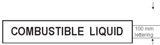
Figure 5—Placard for C1 combustible liquids
