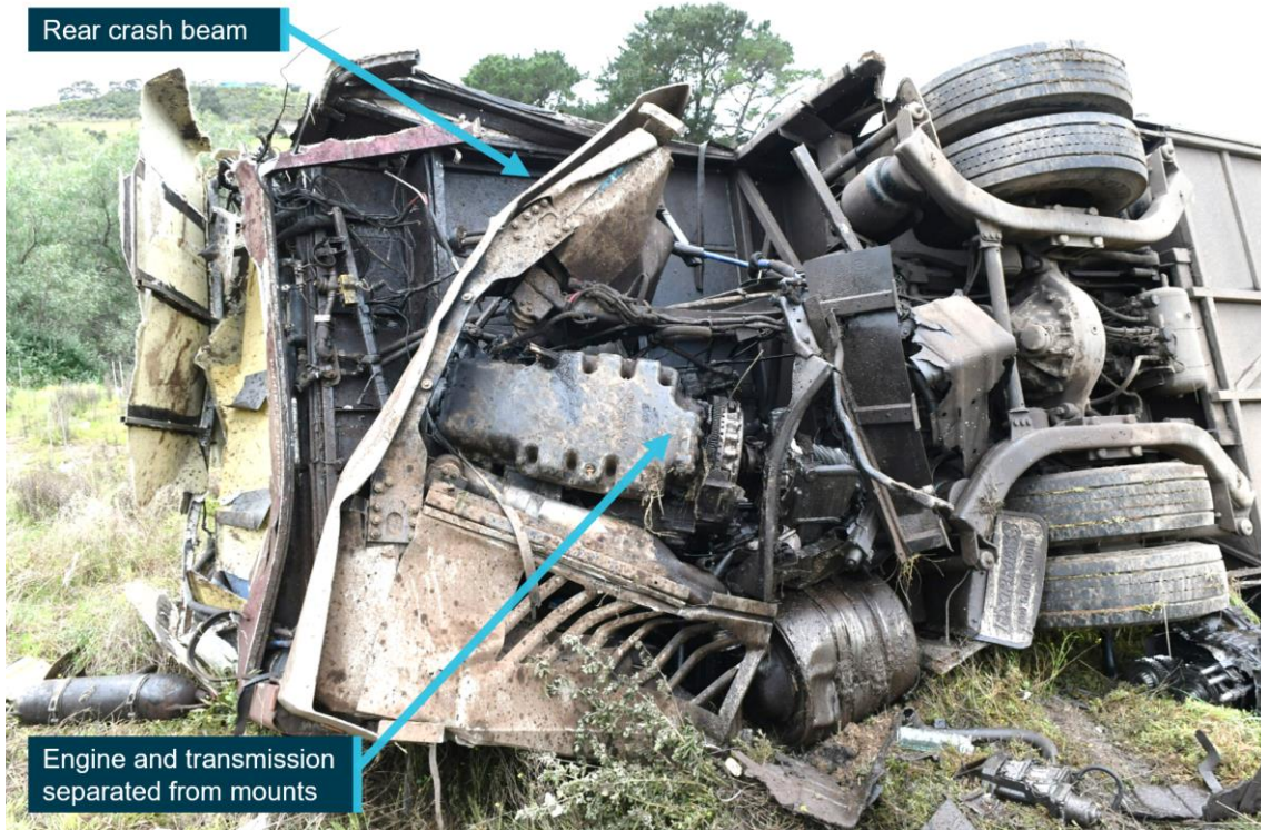
Figure 10: Passenger coach rear impact damage
