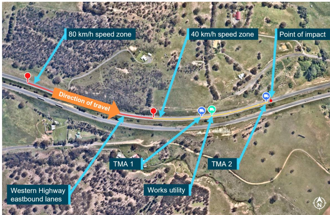
Figure 3: Temporary traffic management arrangement – Western Freeway eastbound
