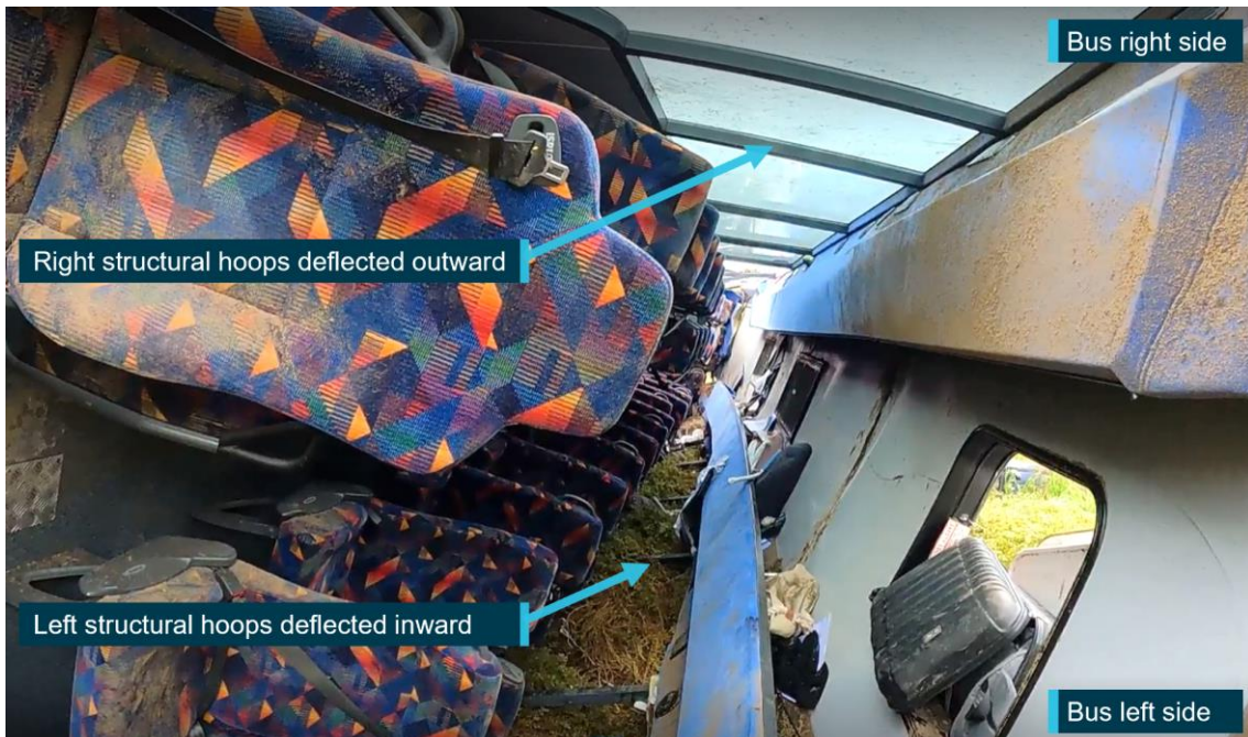
Figure 11: Passenger coach interior damage (view toward the rear of the vehicle)
